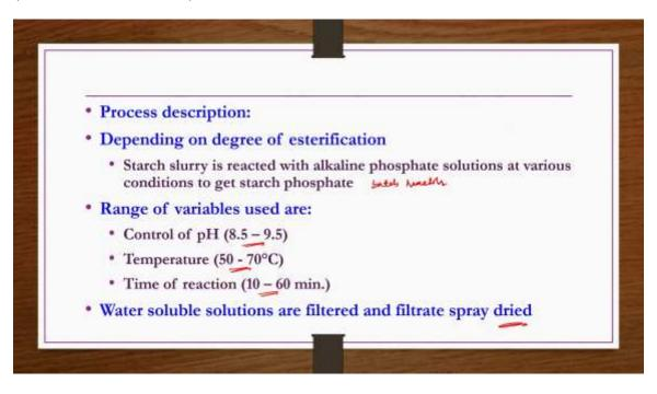
Chemical reaction, starch reacting with the sodium phosphates to get the starch phosphates by releasing the water, okay? Process description depending on degree of esterification required, starch slurry is reacted with alkaline phosphate solutions at various conditions to get starch phosphate in batch reactors, okay? Then the slurry is centrifuged to get the product.
