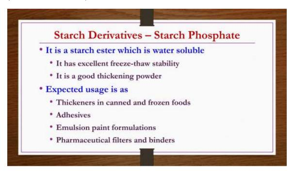
Next starch derivative is starch phosphate where starch is reacting with the sodium phosphates to get starch phosphates in a simple batch reactor. This is a starch ester which is water soluble.
