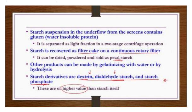
Starch suspension in the underflow from the screens contains gluten which is water insoluble protein. It is separated as light fraction in a two-stage centrifuge operation. Starch is recovered as filter cake on a continuous rotary filter. It can be dried, powdered and sold as peeled starch or other products can be made by gelatinizing with water or by hydrolysis if you do not want in dry conditions, okay? Starch derivatives are dextrin, dihaldehyde starch and starch phosphate, etc.
