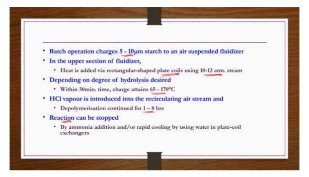
So, whatever we discussed here in the flowchart, the same thing we are going to see here again. Batch operation charges 5 to 10-micron starch to an air suspended fluidizer. In the
