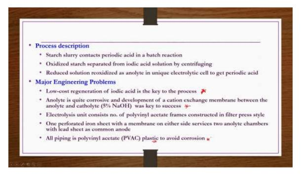
Process description, starch slurry contacts periodic acid in a batch reactor, oxidized starch separated from iodic acid solution by centrifuging, reduced solution reoxidized as analyte in unique electrolytic cell to get periodic acid which can be reused for the next step, next batch purpose.
