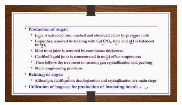
Then if you see the steps involved in the production of sugar, crudely juice is extracted from washed and shredded canes by pressure mills. This juice would be having so many
