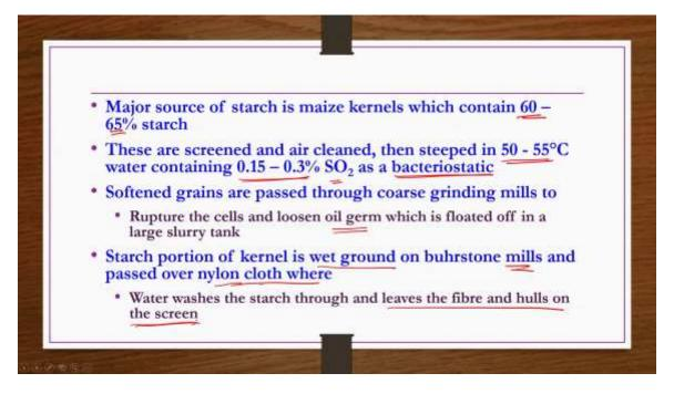
Whatever we discussed in the flowchart the same thing we are having here once again in the text form. Major source of starch is maize kernels which contains 60 to 65% starch which is very high. So, these are screened and air cleaned then steepened or soaked in 50 to 55-degree centigrade water containing 0.15 to 0.3% SO<sub>2</sub> as bacteriostatic you do not
