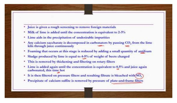
Whatever we discussed in the flowchart the same thing is provided here as a text for the understanding. Juice is given a rough screening to remove foreign materials after collecting from the diffuser. After collecting from the diffuser whatever the juice is there it is given a rough screening to remove foreign materials.
