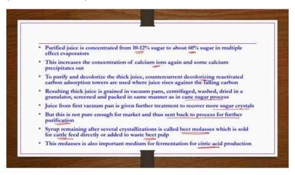
Then purified juice is concentrated from 10 to 12% sugar to about 60% sugar in multiple effect operators. This increases the concentration of calcium ions again and some calcium precipitates out. To purify and decolorize the thick juice, countercurrent decolorizing reactivated carbon adsorption towers are used where juice rises against the falling carbon.
