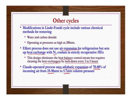
Other cycles are also there some modification something like that modification in Linde Frankl cycle include various chemical methods for removing water and carbon dioxide and then operating at pressures as high as 200 atmospheres; however, another process that is Elliott process does not use air expansion for refrigeration, but sets up heat exchange with O2 coolant in strictly recuperative heat exchangers.
