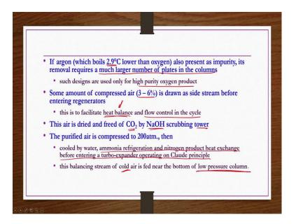
So, if argon which boils at 2.9 degree centigrade lower than oxygen is also present as impurity its removal requires much larger number of plates in the columns. In the fractionation column these are nothing but the these indicating the plates large number of plates may be required if you wanted to go for the you know high purity any of the chemicals that you wanted to purify by distillation.
