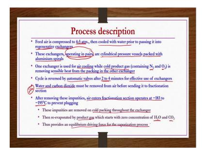
Now, we see process description then we are going to see the same thing in flow sheet as well ok. The feed air is compressed to 4 to 5 cool after compressing it is cooled with water prior to passing it into regenerative exchangers. These regenerative exchangers are very important aspects of the process because in other process or probably up to this exchangers step whatever is there; that means, to only different from one process to the other process.
