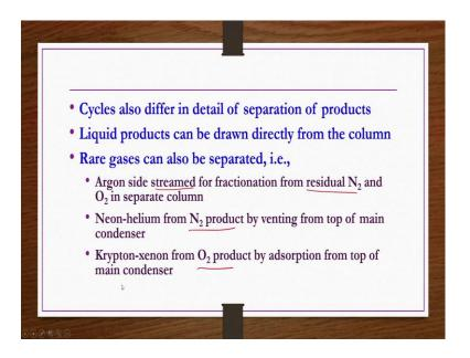
Cycles also differ in detail of separation of products how the separation is being done. So, liquid products can be drawn directly from the column rare gases can also be separated that is argon side streamed for a fractionation from residual N2 and then O2 in separate column or neon helium from N2 product by venting from top of main condenser or krypton-xenon from O2 product by adsorption from top of main condenser, ok.
