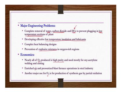
So, whatever the cycles that we have seen for the production of low purity oxygen or high purity oxygen now, they seems to be simple and then having only a compression and expansion kind of units, but however, there are certain kind of engineering problems associated with these cycles as well and then one must be careful about them what are the complete removal of water is one problem.
