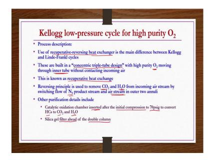
Now, what we do we see Kellogg low pressure cycle for high purity oxygen. So, process description as I mentioned use of recuperative reversing heat exchanger is the only or main difference between Kellogg cycle that we are going to see and then Linde-Frankl cycle that we have already seen in the previous slide. These are built in a concentric triple tube design with high purity O2 moving through inner tube without contacting incoming air this is known as recuperative heat exchanger.
