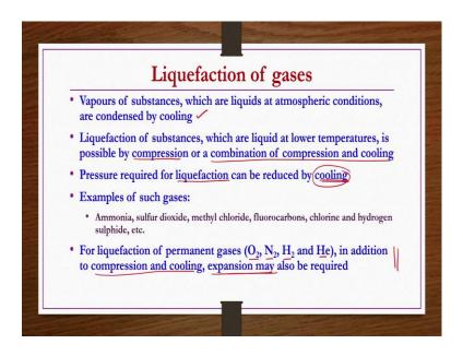
Let us say; however, liquefaction of substances if you wanted to those substances are liquid at lower temperature then it is possible to further do the liquefaction of such substances by compression or by a combination of compression and cooling ok. So, pressure required for liquefaction can be reduced by cooling as well.
