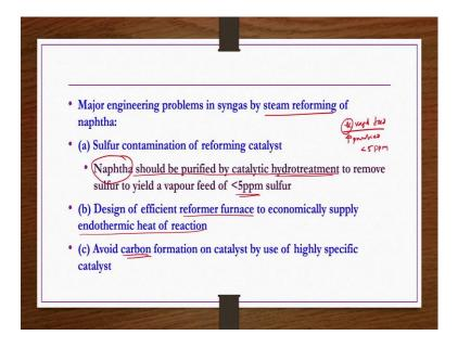
So, before going into the details of production of synthesis gas by partial combustion of naphtha or natural gas and what we do? We will be having a kind of a discussion about major engineering problems in production of syngas by steam reforming of naphtha that we have seen yesterday.
