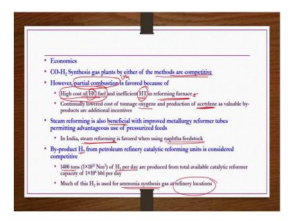
Coming to the economics of synthesis gas by both methods. CO H 2 synthesis gas plants by either of the methods are competitive. So, we cannot say which is good which is bad it depends on the feed and all that ok; however, partial combustion is favored because of high cost of hydrocarbon fuel.
