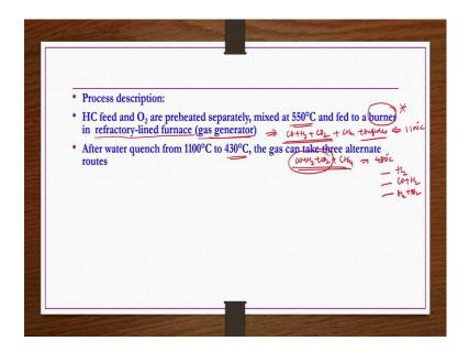
Now, first we see the process description because as I mentioned process description after the partial combustion reaction taking place in a gas generator reactor, the separation sections are more or less same as what we have seen in the previous class where steam reforming of naphtha has been studied discussed in order to get synthesis gas ok.
