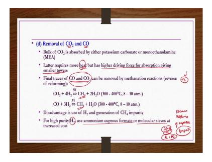
Then removal of CO 2 and then CO. Because we know that process if you are required to do the synthesis gas production this plant if you wanted to operate in order to produce high concentrate or highly purified hydrogen then this CO 2 and CO has to be removed. So, then how efficiently are you removing that is going to be very essential ok.
