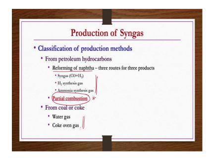
So, now, what are the different types of production methods we have seen? There are two major methods one is from petroleum hydrocarbons if you are using petroleum hydrocarbons or natural resources or something like a natural gas etcetera then we have two methods if you are producing this from coal or coke, then we have a two methods.
