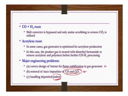
If you wanted to have CO plus H 2 route so, that to get synthesis gas with the various you know ratio of CO plus H 2 only without any CO 2. Then what you have to do? You just bypass that water gas shift converter and then remove CO 2 by absorption that is it.
