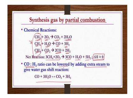
So, now we see synthesis gas production by partial combustion ok. Now first we see chemical reactions CH 4 reacts with O 2 to give CO 2 and 2 H 2 O, 2 moles of oxygen we are utilizing. And then CH 4 reacting with water giving rise to CO plus 3 H 2 and then another possible reaction is CH 4 reacting with already produce CO 2 giving rise 2 CO and 2 H 2 right.
