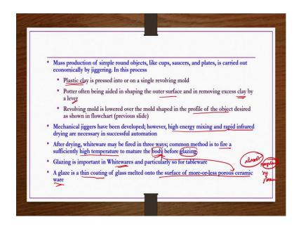
Mass production of simple round objects like cups, saucers and plates is carried out economically by jigging. In this process plastic clay plastic clay is the one after you know removing the flocculants and then removing the magnetic particles etcetera or materials having magnetic characteristics once you remove them.
