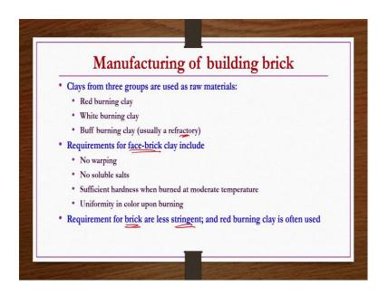
Volatilized salt reacts to form fusible coating or glaze. Now, we talk about manufacturing of building brick. Clays from three groups are used as raw materials these are nothing but red burning clay, white burning clay and buff burning clay which is usually a refractory. Requirements for face brick include several stringent conditions like
