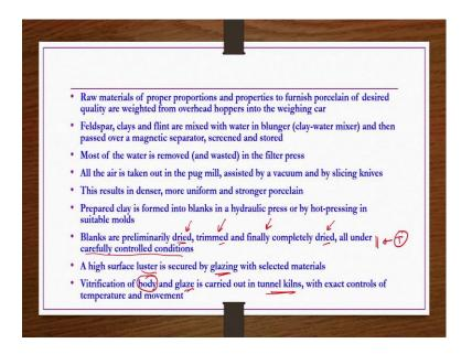
Raw materials of proper proportions and properties to furnish porcelain of desired quality are weighed from overhead hoppers into the weighing car Feldspar clays and flint are mixed with water in blunger and then passed over a magnetic separator screened and stored. Most of the water is removed in the filter press and then water is discarded as wastewater.
