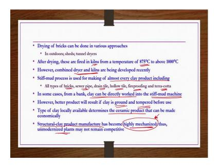
Drying can be done in various approaches. Three most important approaches are in outdoors, sheds or tunnel dryers. After drying these are fired in kilns from a temperature of 875 degree centigrades to 1000 degree centigrades. However combined dryer and kilns are also being developed recently. Stiff mud process is used for making almost every clay product including all types of bricks, sewer pipe, drain tiles, hollow tiles, fireproofing and terracotta.
