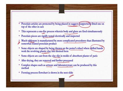
Porcelain articles are protected by being placed in saggers. In saggers which are nothing but supporters fitted one on top of the other in cars. This represents a one-fire process wherein body and glaze are fired simultaneously. Porcelain pieces are rigidly tested electrically and inspected alright.
