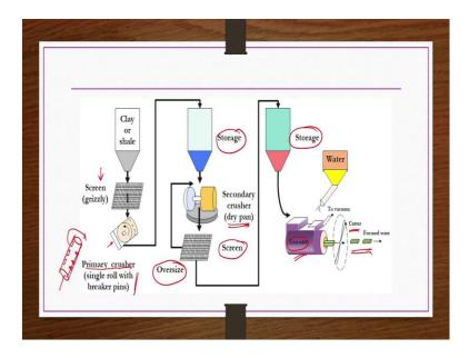
So, flowchart is shown here, so whatever the clay or shale etcetera. Raw materials are there, they will be passed through screens, grizzlery kind of screens. So, that to remove bigger particles or unnecessary particles of different shapes etcetera alright or you know needle kind of particles etcetera all those kind of things are removed here.
