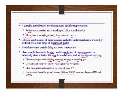
This glazing contains ingredients of two distinct types in different proportions. Refractory materials such as feldspar silica and china clay and then fluxes such as soda, potash, fluorspar and borax. Refractory materials provide thermal stability, chemical stability whereas, the fluxes they reduce the reaction temperature as well as the vitrification temperature.
