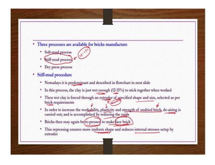
Three processes are available for bricks manufacture also what are they, they are nothing but soft mud process, stiff mud process, dry press process ok. So, we will be discussing about a stiff mud process what it is. Stiff mud process in the sense it will be having only limited water it will use only water of up to 12 to 15 percent. So, that to you know make a the raw materials mixed together.
