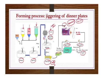
So, forming process here we talk about jiggering of dinner plates. Now, flow sheet here if you see up to getting a slurry wet filter cake the process is similar whatever we have seen in previous steps, but; however, we have the details here. So, the clays flint and feldspars are taken as per the proportions required or as per the composition into a blunger to which water is also provided the blunger is nothing but a kind of mixers.
