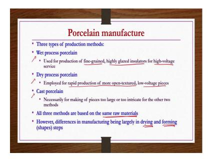
Now, we discuss about the manufacturing of porcelain. Three types of production methods are possible for the manufacturing of porcelain; one of which is wet process or wet process porcelain. It used for production of fine grained highly glazed insulators for high voltage services purpose. Second one is the dry process porcelain. It is employed for rapid production of more open textured low voltage pieces whereas, third one is cast porcelain.
