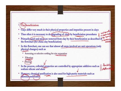
So, as we have already seen, the clays that are we are having, you know it is having impurities, impurities like sand, mica, iron oxide, etcetera. So, they have to be removed. Removal of these impurities from the clay is known as clay beneficiation. We are not calling clay purification because clay is not one single component that we are purifying. It is a combination of different components, right.
