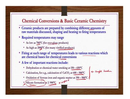
Now, we are going to see second important topic of the today's lecture that is basic ceramic chemistry. Chemical conversions and basic ceramic chemistry. Ceramic products are prepared by combining different amounts of raw materials that we have discussed, shaping and heating to firing temperatures.
