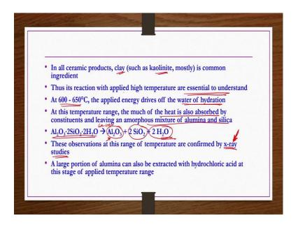
So, now what we understand until now, in ceramic products, clay such as kaolinite, mostly not the only one is very common ingredient. And then thus, its reaction with applied high temperature or essential to understand, right. So, at 600 to 650 degree centigrade, the applied energy drives off the water of hydration that is, you know dehydration reaction etcetera takes place.
