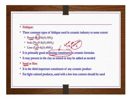
Now, we go to the second raw material that is feldspar. 3 common types of feldspar used in ceramic industry to some extent. They are nothing but potash, soda and then lime based feldspar. So, potash based is nothing but K2O, Al2O3 because of K2O presence, it is known as a potash feldspar. Whereas, the soda is having Na2O, that is the reason it is called as soda feldspar.
