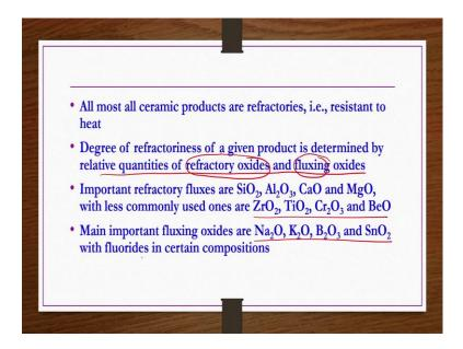
Almost all ceramic products are refractories that is resistant to heat. Degree of refractoriness of a given product is determined by the relative quantities of refractory oxides and fluxing oxides. Fluxing oxides we have seen. So, fluxing oxides, they reduce the reaction temperature or vitrification temperature. Whereas, the refractory oxides, they provide required thermal resistance or thermal stability.
