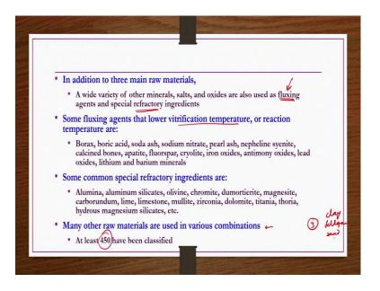
In addition to 3 main raw materials, a wide variety of other minerals, salt, oxides are also used as fluxing agents and special refractory ingredients. Fluxing agents, they purpose, they reduce the reaction temperature or vitrification temperature. That is the reason you need to have such fluxing agents.
