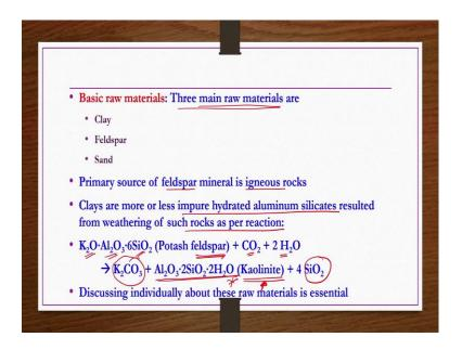
So, basic raw materials of ceramic industry, 3 main raw materials are very common in any of the ceramic product that you take. So, one of them is clay, another one is the feldspar, third one is the sand, ok. Primary source of a feldspar mineral is igneous rocks. Clays are more or less impure hydrated aluminum silicates resulted from weathering of such rocks as per the reaction given below.
