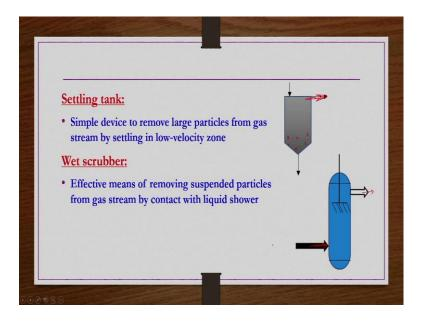
Then, settling tank – they are simple device to remove large particles from gas stream by settling in low velocity zone. So, we have a container here what we do particle lead and gases whatever are they we allowed to come into this container. So, the particles are having you know higher settling velocity compared to the gas particles rather gas particles do not settle at all.
