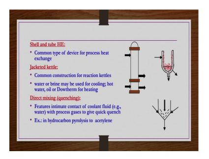
Shell and tube heat exchanger common type of device for process heat exchange. Pictorial it is shown here. Jacketed kettle: common construction for reaction kettles; water or brine may be used for cooling; hot water oil or dowtherm for heating is used in general. So, let us say what we have? We have a reactor vessel like this. This is the reactor vessel and then whatever the reactant that you wanted to react with or the provider, they are taken here.
