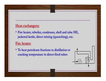
Heat exchangers: there are different types of heat exchangers are there. One particular type of heat exchanger which is very common is a shell and tube heat exchanger. Others are like fire heater, reboiler, condenser, jacketed kettle, direct mixing or quenching etcetera.
