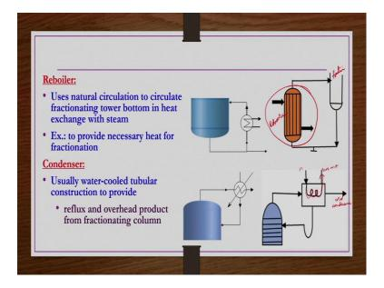
A reboiler uses natural circulation to circulate fractionating tower bottom in heat exchange with steam. Example: to provide necessary heat for fractionation. Pictorially if you see, so, this is the fractionator. This column which is not completely shown now here the reboiler is important. So, this is reboiler actually.
