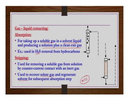
Gas-liquid contacting: absorption: for taking up a soluble gas soluble gas in a solvent liquid and producing a solution plus a clean exit gas we are using this absorption, alright. Such as, used in H 2 S removal from hydrocarbons usually also contain H 2 S because petroleum crude whatever we have the sulfur components would also be there.
