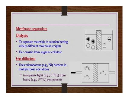
Membrane separations, there are different types of membrane separation processes are there like you know micro filtration, ultra filtration, nano filtration, dialysis, electro dialysis like several types are there. So, some of them based on the size, some of some of them are based on the delta p, some of them are based on delta c, some of them are based on the delta charge whatever electromagnetic force difference differences are there.
