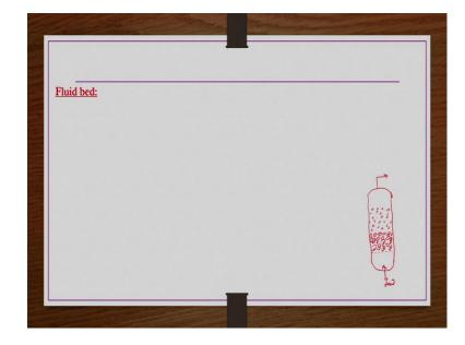
Now, if you have a kind of a fluid bed reactor or fluidized bed reactor so, then how does it look like? Let us say you have a column again. Cylindrical column at the bottom you what you have you have a perforated plate like this right and then this is the top of the column. So, here you are not closing the top of the bed now, rather bed what you have? You have a packing material. now, let us say catalyst like this which is not packed which is not packed initially, right.
