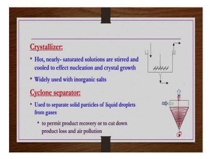
Crystallizer: Hot nearly saturated solutions are stirred and cooled to effect nucleation and crystal growth. Pictorially it is shown here. They are widely used in inorganic salts. Cyclone separator: used to separate solid particles of liquid droplets from gases or very fine or very fine solid particles from the gases – to permit product recovery or to cut down product losses and air pollution.
