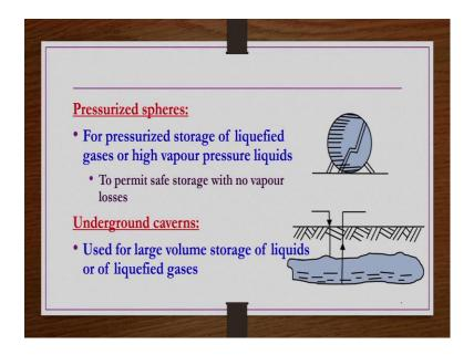
Pressurized spheres – for pressurized storage of liquefied gases or high vapour pressure liquids these pressurized spheres are used so that to permit safe storage with no vapour losses. Pictorially shown here. Then underground caverns – used for large volume storage of liquids or of liquefied gases. Pictorially they are shown here like this, ok.
