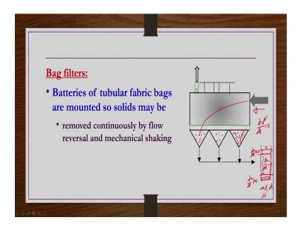
Then bag filters is very simple process where batteries of tubular fabric bags are mounted. So, solids may be removed continuously by flow reversal and mechanical shaking. So, let us say you have a you know a column like this. Now, what you have? You are you are having different bags fabric bags like this 1, 2, 3 like this and number of you can have.
