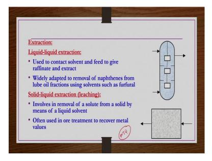
Extraction: liquid-liquid extraction and solid-liquid extraction are possible. In the liquidliquid extraction they are used to contact solvent and feed to give raffinate and extract. Widely adapted to removal of naphthenes from a lubricated from lube oil fractions using solvents such as furfural. Pictorially it is shown here.
