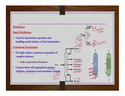
Next important unit operation is distillation. There are different types of distillations are there. So, then we are going to see only batch and continuous distillation. Batch distillation used for intermittent operation and then handling small volumes of feed and product.
