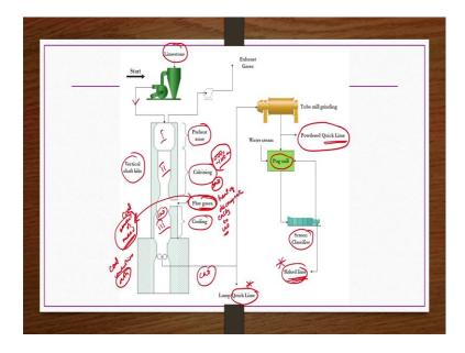
Now, this is the flow chart for making quick lime as well as slake lime as well hydrated lime. So, we see in detail here. Whatever the limestone rock is there, raw limestone or
