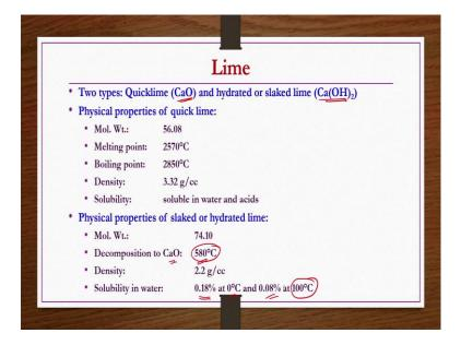
Two types of limes are possible, one is the quick lime that is calcium oxide and another one is the hydrated or slaked lime which is nothing, but calcium hydroxide. Now, we see the physical properties of both individually. Physical properties of quick lime, molecular weight is 56.08, melting point is 2570 degree centigrades, boiling point is 2850 degree centigrade, density is 3.32 gram per cc, solubility, soluble in water and the acids.
