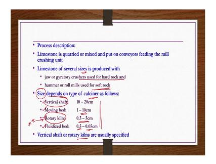
Now we see description of this process here. Process description limestone is quarried or mixed and put on conveyors feeding the mill crushing unit, limestone of several sizes is produced with jar or gyratory crushers used for hard rock and then if the rock is soft rock then hammer or roll mills are used especially when the soft rock is there. Size depends on the type of calciner as follows, different types of calciners are there in general that is what it means by.
