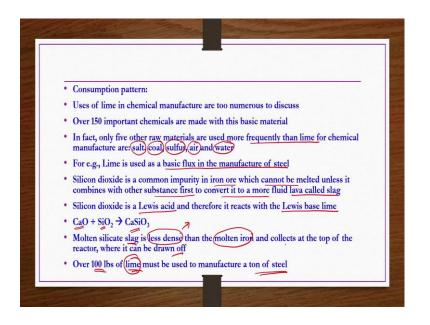
Consumption pattern, so the application or utilization of calcium hydroxide for chemical industries is huge more than 150 chemicals are produced either by using this one directly or indirectly for the process. Such largely it is used. In fact, it is one of the top 5 chemicals, which are vastly used.
