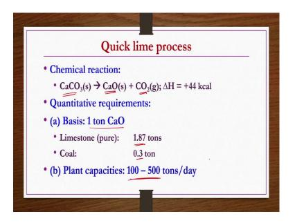
Quick lime process, chemical reactions if you see. If you apply heat to the calcium carbonate, you can get the calcium oxide by releasing the carbon dioxide. Quantitative requirements, if you want to produce one ton of calcium oxide, pure limestone 1.87 tons required, coal 0.3 tons required and plant capacity varies between 100 and 500 tons per day in general.
