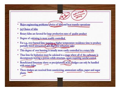
Major engineering problems of this process two important are there; one is the choice of kiln and then another one is the heat transfer operation. Choice of the kiln as I already specified in the one of the previous slide depending on the size of size reduced lime stone based on that one has to select but.
