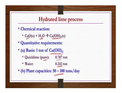
Now, hydrated lime process, here chemical reactions if you see calcium oxide whatever the lime quick lime you got that if you do the hydration then you get calcium hydroxide or hydrated lime ok. Quantitative requirements in order to get a one ton of calcium hydroxide or hydrated lime, quick lime pure one you need 0.787 tons, water you required 0.242 tons and then plant capacity between 500 and 100 tons per day in general.
