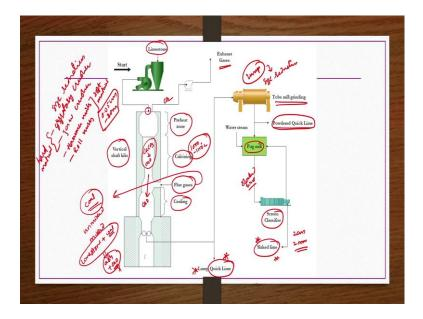
So, the same flow sheet is shown here again ok. So, the limestone whatever is there, that is usually size reduced in a size reduction unit, size reduction can be done by you know gyratory crushers or jaw crushers. If the material is wet, these kind of gyratory crushers are used if the material or the limestone is hard material, if it is soft material then hammer mills or roll mills are used for soft material soft limestone if you are having that one you do.
