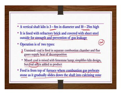
A vertical shaft kiln is 3 to 8 meters in diameter and 10 to 25 meters high that whatever the flowchart we have seen that is usually having 10 to 25 meters high and then 3 to 8 meters diameter. It is lined with refractory brick and covered with a sheet steel outside for strength and prevention of gas leakage. Operations are two types because in this kind of material the coal is also mixed sometimes.
