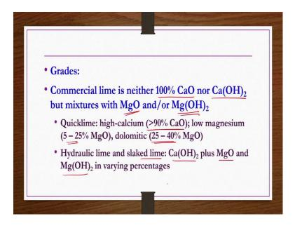
Grades, whether quick lime or hydrated lime it is not available in 100 percent pure form commercially, so they are usually mixed. Commercial lime is neither 100 percent CaO nor 100 percent calcium hydroxide, but it makes sure with magnesium oxide and or magnesium hydroxide.
