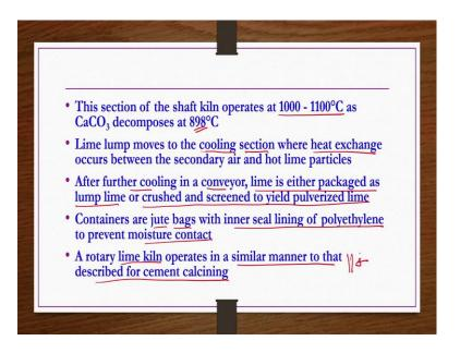
This section of the shaft that is calcining zone of the kiln operates at 1000 to 1100 degree centigrade as calcium carbonate decomposes at around 898 degree centigrades. Lime lump moves the cooling section where heat exchange occurs between the secondary air and hot lime particles. After further cooling in a conveyor, lime is either packaged as lump lime or crushed and screened to yield pulverized lime as per the requirement.
