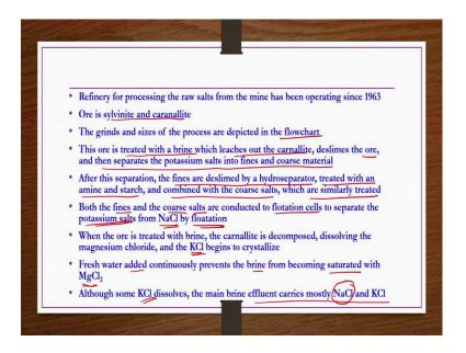
So, now the details we see in descriptive text form here refinery for processing the raw salts from the mine has been operating since 1963 ore is sylvinite and carnallite. The grinds and sizes of the process are depicted in the flowchart as discussed in the previous slide. This ore is treated with a brine which leaches out the carnallite, deslimes the ore then separates the potassium salts into fines and coarse material using the screens.
