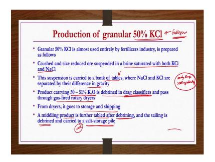
Now, granular 50 percent KCl production, how do you do? Because 50 percent KCl is often used as it is for a fertilizer purpose or in fertilizer industries, ok. Granular 50 percent KCl is almost used entirely by fertilizers industry is prepared as follows it is very simple process crushed and size reduced ore suspended in brine saturated with both NaCl and KCl, ok.
