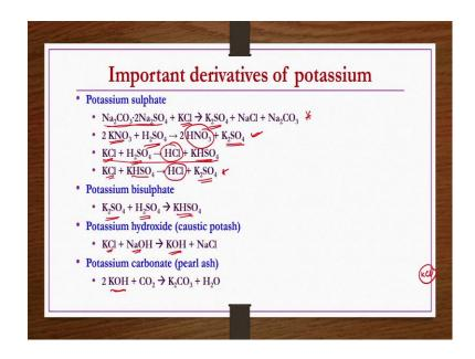
For example, some of the important derivatives of potassium under this category if you take potassium sulphate you take a burkeite that is mineral Na 2 CO 3 2Na 2 SO 4 and then react with KCl you can get potassium sulphate sodium chloride and sodium carbonate. This is one possible way, but there are other possible ways also. Let us say if you take potassium nitride and then react with sulfuric acid then also you can get potassium sulphate.
