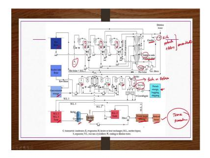
Briefly, if we recapitulate this trona-procedure, then what we have? We have a brine, we make it hot by using this steam and then it is fed to triple effect evaporator. So, that it can be concentrated. Whatever the concentrated brine after passing through this triple effect evaporator, it will be much more concentrated and then water would be evaporated off, ok that water would be condensed and collected anyway, right.
