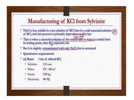
Now, what we will be doing in this lecture? In this lecture we will be having a discussion how to get the potassium chloride by different approaches as well. So, first one is manufacturing of KCl from sylvinite. Here the basis of this process is that NaCl or sodium chloride is less soluble in hot potassium chloride solution than in cold saturated potassium chloride solution, right.
