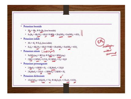
Potassium bromide if you want it to do it is a two-step process. Iron reacts with the bromine to give iron bromide which further reacts with the potassium carbonate and water to give potassium bromide and then hydroxide of iron ok along with the carbon dioxide.
