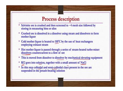
This is one process the description of the process is given here sylvinite ore is crushed and then screen to 4 mesh size followed by storing in measuring bins or silos crushed, ore is dissolved in a dissolver using steam to form mother liquor cold mother liquor is heated to 110 degree centigrades by use of heat exchangers employing exhaust steam.
