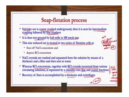
Soap floatation process is another process where you can produce a KCl easily ok. What we do here sylvinite is the ore that we take it is crushed in a three different types of crushers one is the coarse crushers followed by the intermediate crushing then followed by the fine crushers.
