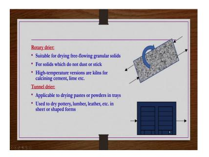
Then rotary drier they are suitable for drying free flowing granular solids, for solids which do not dust or stick and then high temperature versions or kilns for calcining, cement, lime etcetera they are very common in organic chemical industries. So, pictorial representation is given here. Then tunnel driers applicable to drying pastes or powders in trays used to dry pottery, lumber, leather etcetera in sheet or shaped forms.
