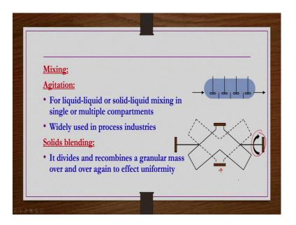
Then mixing agitation is one of the type of mixing which is used for the liquid-liquid or solid-liquid mixing in single or multiple compartments. For example, here you have a agitation equipment where different multiple compartments are there, where these materials are coming and being agitated or mixed and then uniform or properly mixed material is taken out from this end ok.
