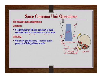
The grinding is next level size reduction equipment as I mentioned crushing is a one kind of operation which is used for the coarse reduction, grinding is a kind of one operation where intermediate or medium size reduction has to be done. So, here wet or dry grinding may be carried out in presence of balls, pebbles or rods.
