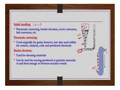
Next is Solids handling, pneumatic conveying, bucket elevators, screw conveyors, belt conveyors etcetera comes under this picture. So, these things also you may find in mechanical unit operation course much details. In the pneumatic conveying what happened there is usually used for the grains; however, now also used widely for cement catalysts coke and powder chemicals etcetera.
