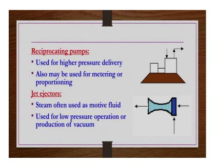
Reciprocating pumps used for higher pressure delivery also may be used for metering or proportioning, a pictorial representation is shown here. Jet ejectors steam often used as motive fluid used for low pressure operation or production of vacuum, pictorially shown here in jet ejectors ok. This is about a few of a common unit operations in the next class we are going to see a few more unit operations which are very common in chemical plants ok.
