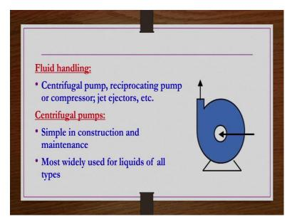
Next is Fluid handling, different types of fluid handling equipments or pumps are available some of them are centrifugal pump, reciprocating pump or compressors, jet ejectors etcetera. Centrifugal pumps simple in construction and maintenance mostly used for liquids of all types, where centrifugation principles are used to transport the fluid from one level to the other level.
