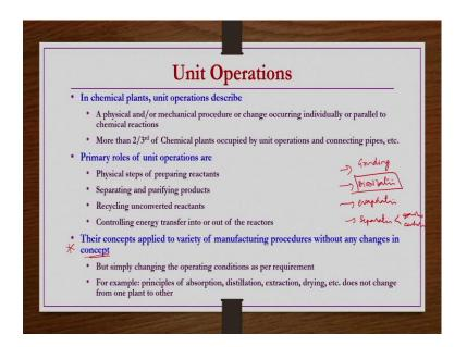
So, in chemical plants unit operations describe a physical and a mechanical procedure or change occurring individually or parallel to chemical reactions or unit processes and then more than 2 by 3rd of chemical plants occupied by unit operations and connecting pipes etcetera.
