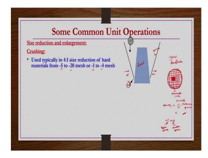
Crushing let us say it is a jaw crusher type it is one of the equipment representation of one of the coarse reduction equipment we call it jaw crusher; where there are 2 jaws are there one is fixed another one is moving right. So, let us say here it is fixed it can be other way also not necessary only this one has to be fixed and then this one has to be moved it is other way also and then this is moving and then this moves in this direction in one particular direction like this right.
