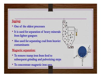
Jigging is one of the oldest processes it is used for separation of heavy minerals from lighter gangues, also used for separating coal from heavier contaminants in general. But
