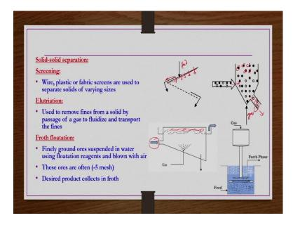
Next solid-solid operations such kind of unit operations also we studied in detail in mechanical unit operations course; however, few details we see here Screening. Screening as I mentioned you know they are wire plastic or fabric screens often they are used to separate solids of varying sizes.
