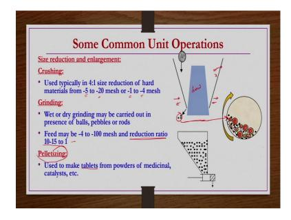
Now, here feed may be minus 4 to minus 100 mesh size and then reduction ratio may be 10 to 15 to 1 ok. Reduction ratio is nothing but the it is feed size divided by the product size, product size is obviously the smaller one compared to the feed size ok. Pelletizing is a size enlargement equipment size enlargement process alright.
