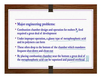
Major engineering problem combustion chamber design and operation for molten P 4 feed required a great deal of development under improper operation a glassy type of meta phosphoric acid and its polymers can form which is not desirable product. These often drop to the bottom of the chamber which mandates frequent shutdown and clean out. So, one has to control the feed ok.
