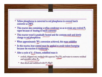
Yellow phosphorus is converted to the red phosphorus in covered batch converter at 250 degree centigrades. This reactor also containing a reflux condenser so, as to retain any evolved P 4 vapor because of heating in the batch converter. This reactor vessel is gradually heated and contents melt and slowly change to red phosphorus. When approximately 70 percent conversion is achieved this mass gets solidified.
