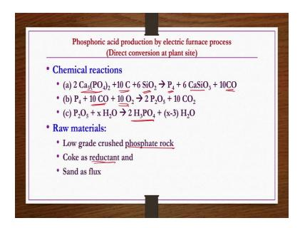
Phosphoric acid production by electric furnace process that is direct conversion at plant site. Chemical reactions whatever the fluorapatite mineral is there that is in the phosphate rock that would be reacting with the coke and then silica of the sand to give phosphorus and then calcium silicate and carbon monoxide.
