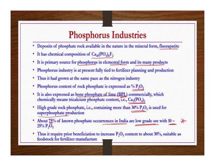
This phosphate rock available in the nature in the mineral form, which is known as fluorapatite. This is having chemical structure Ca 10, PO 4 6, F 2. It is primary source for phosphorus in elemental form and its many products as well, whatever the phosphoric acid, P 2 O 5 etcetera or any other mixed chemical fertilizers, where phosphorus is also used.
