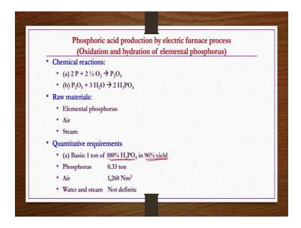
Now, we see phosphoric acid production by electric furnace process, oxidation and hydration of elemental phosphorous. Here the chemical reactions whatever the elemental phosphorous is there that you do oxidation then you get P 2 O 5. This P 2 O 5 reacts with water to give phosphoric acid raw materials; obviously, elemental phosphorous and then air and then steam.
