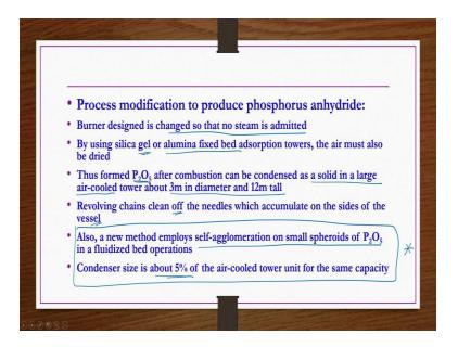
Process modification to produce phosphorous anhydride. Burner designed is changed so, that no steam is admitted and then by using silica gel or alumina fixed bed adsorption towers the air must also be dried. Thus formed P 2 O 5 after combustion can be condensed as a solid in large air cooled tower about 3 meter in diameter and 12-meter-tall. Revolving chains clean off the needles which accumulate on the sides of the vessel.
