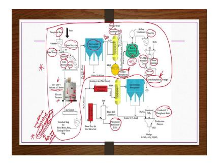
Now, this is the flow chart for the production of a yellow phosphorus, red phosphorus, phosphoric anhydride P 2 O 5 and then purified phosphoric acid right. These many are there in one plant usually it is there. So, we take step by step what we do? We first concentrate on production of yellow and red phosphorus.
