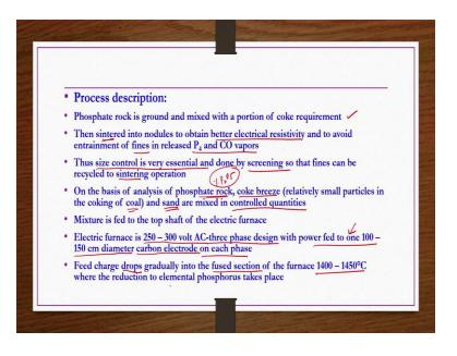
Phosphate rock is ground and mixed with portion of coke requirement, then sintered into nodules to obtain better electrical resistivity and to avoid entrainment of fines in released P 4 and CO vapors whatever are forming after the reduction reaction in the furnace that is the advantage of sintering essentiality of the sintering.
