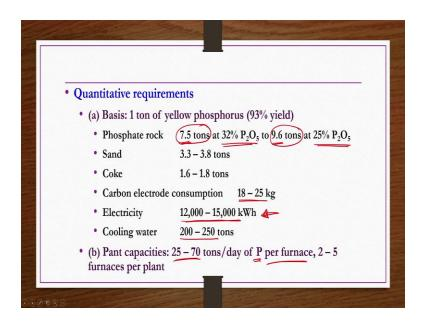
Quantitative requirements if you see basis 1 ton of yellow phosphorus with 93 percent yield if you wanted to produce phosphate rock you need 7.5 tons at 32 percent P 2 O 5 to 9.6 tons at 25 percent P 2 O 5. So, this number of tons 7.5 to 9.6 that depends on the what is the purity of P 2 O 5 in the raw material phosphate rock that you have taken right.
