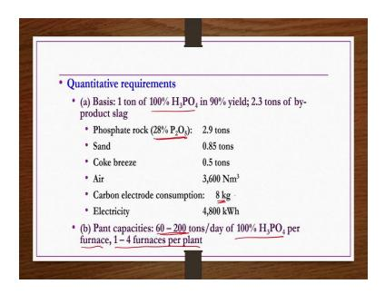
Quantitative requirements basis 1 ton of 100 percent H 3 PO 4 in 90 percent yield in addition to that 2.3 tons of by-product slack if you wanted to produce. Phosphate rock 28 percent P 2 O 5 you need 2.9 tons, sand 0.85 tons, coke bridge 0.5 tons, air 3600 normal cubic meters, carbon electrode consumption 8 kgs, electricity 4800 kilowatt hour and then plant capacity 60 to 200 tons per day of 100 percent H 3 PO 4 per furnace and then there may be 1 to 4 furnaces per plant.
