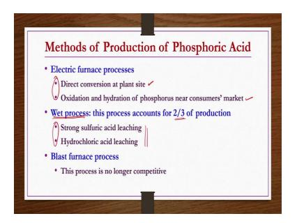
Methods of production of phosphoric acid there are several methods. We take one by one. The first one is electric furnace method where we have direct conversion at plant site and then oxidation and hydration of phosphorus near consumers market. So, these two methods we are going to discuss now. Then wet process, this process account for two-third of phosphoric acid production.
