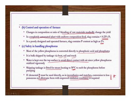
Control and operation of furnace changes in composition or ratio of blending of raw materials markedly change the yield because of the percentage of P 2 O 5 that is present and then because of the size of the sintered phosphate rock. If you have a completely automated plant with uniform composition feed then slag contains less than 0.25 percent P.
