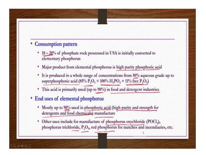
Consumption pattern if you see in USA whatever phosphate rock processed out of which 18 to 20 percent is utilized for converting into elemental phosphorus. Major product from elemental phosphorus is high purity phosphoric acid which is used for different purposes.
