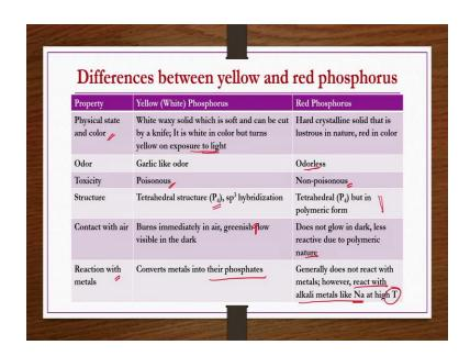
Now, we see a few basic differences between yellow and red phosphorus. Physical property physical state and color if you see this yellow phosphorus actually which is white in color white waxy solid which is soft and can be cut by knife, but though it is in white in color, but turns into yellow on exposure to light that's the reason it is also known as the yellow phosphorus as well.
