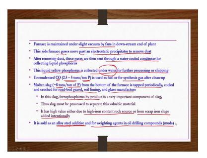
Furnace is maintained under slight vacuum by fans in downstream end of plant this aids furnace gases move fast an electrostatic precipitator to remove the dust. After removing the dust these gases are then sent through a water cooled condenser for collecting liquid phosphorus product. This liquid yellow phosphorus is collected under water for further processing or shipping under water because of safety concerns because when it comes into contact with air it immediately ignites.
