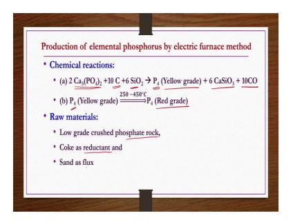
Now, we see production of elemental phosphorus by electric furnace method ok. So, we start with the conventional process of starting with reactions raw materials, basis etcetera. So, chemical reactions whatever the phosphate rock is there fluorapatite that is in the mineral form that reacts with the coke and then silica that is available in the sand we are going to use sand also for this process.
