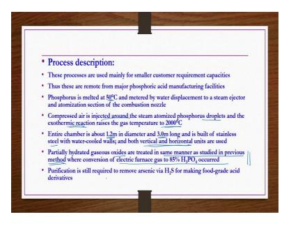
So, this is the third method right. The same method description we are saying these processes are used mainly for smaller customer requirement quantities thus these are removed from major phosphoric acid manufacturing facilities. Phosphorus is melted at 50 degree centigrade and metered by water displacement to a steam ejector and atomization section of the combustion nozzle.
