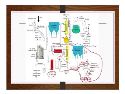
So, now the process is same actually mostly up to the production of these fines whatever from the furnace whatever the P 4 CO are you are producing and then dust etcetera. They are removing the dust from the electrostatic precipitator all that process from up to that point is same.
