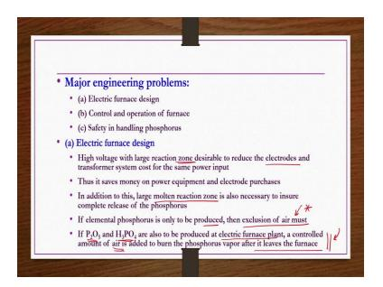
Now, we see major engineering problems, the electric furnace design must be done very carefully because the process is electric furnace process. So, then whatever the reaction is taking place within the reaction is taking place. So, the reaction zone has to be sufficiently large such kind of problems may be there ok. And then power and then how to save the money by giving how much power saving you can do all those things are also needed to be carefully evaluated.
