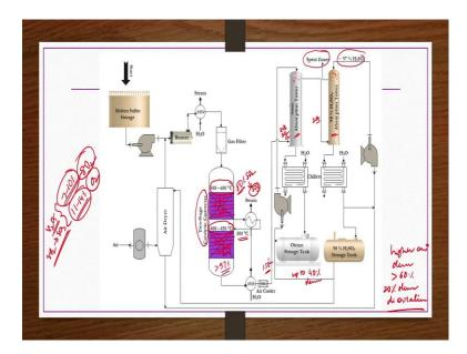
So, now we see contact process by a flowchart. So, whatever the gases, actually for the contact process SO 2 and then oxygen are the primary raw materials, ok. These are actually fed to a catalytic converter, right. These gases have to be dry enough, if they are
