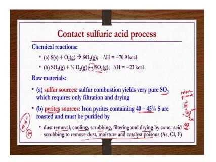
So, now we see details of contact sulfuric acid process. Chemical reactions, elemental sulfur whatever is there that will be oxidized to give sulfur dioxide. This sulfur dioxide will be further oxidized to give sulfur trioxide, this sulfur trioxide would be dissolved in water to get the sulfuric acid.
