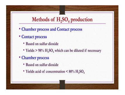
So, methods of sulfuric acid production, chamber process and contact process are two very famous processes. Contact process is based on sulfur dioxide. It yields acid of concentration more than 98 percent, if required which can be diluted. Whereas, the chamber process is also based on sulfur dioxide, but it yields acid of concentration less than 80 percent H 2 SO 4, ok.
