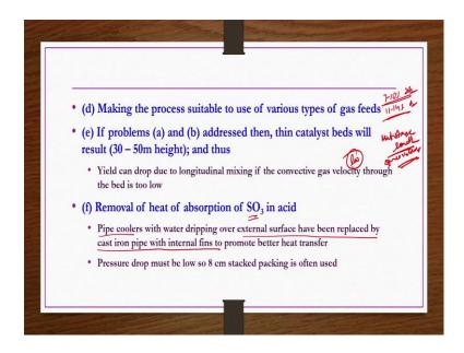
Then, making the process suitable to use of various types of gas feeds. Now, gas feeds in this process what we have seen 7 to 10 percent of SO 2 and then 11 to 14 percent of O 2 only. Why not other percentages? Right. So, such kind of issues should be properly addressed.
