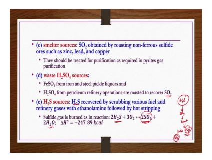
Likewise, smelter sources SO 2 obtained by roasting non-ferrous sulfide ores also such as zinc, lead and copper. And then, here also whatever the sulfur dioxide you get that will not be pure enough. So, then, proper purification should be done as has been done in the case of a iron pyrites ok.
