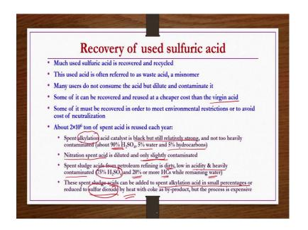
Now, recovery of used sulfuric acid: Sulfuric acid actually for example, it is also used for catalyst purpose. We have seen in the previous lecture, it is a good oxidizing agent, it is also good dehydrating agent etcetera. But it is also used as a catalyst for several organic reactions also, something like alkylation etcetera.
