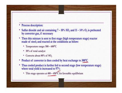
So, this process whatever we have discussed the same thing is provided as a text here. Sulfur dioxide and air containing 7 to 10 percent SO 2 and 11 to 14 percent O 2 is preheated by converter gas if necessary. If necessary in the sense, if the gases are not dry enough then this process is required.
