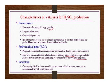
Now, we see characteristics of catalyst for sulfuric acid production. Porous carrier it should have a carrier which is sufficiently porous in nature. For example, alumina, silica, gel, zeolite etcetera. And then, large surface area should be there and then controlled pore size should be there. In zeolites, usually pore size is very much controlled.
