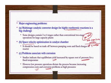
Major engineering problems. First problem is the design of multi-stage converters. Here we have seen only two-stage converters, high temperature and low temperature converters only. But in general, some plants where the capacity is very large up to 1000 tons per day. In such cases, the plant may be having 3-4 stages as well.
