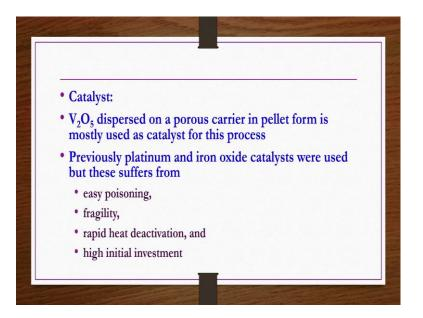
Then, people found V 2 O 5, vanadium pentoxide as a very best catalyst for the production of sulfuric acid. This catalyst is actually used for the conversion of SO 2 to SO 3, ok. So, V 2 O 5 dispersed on a porous carrier in pellet form is mostly used as catalyst for this purpose.
