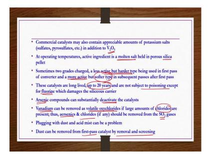
Some more characteristics of this V 2 O 5, with respect to the sulfuric acid production if you see commercial catalyst may also contain appreciable amounts of potassium sulfate, potassium salts in addition to V 2 O 5. At operating temperatures, active ingredients are in general in a molten salt form held in porous silica pellets if you are using silica as base or as carrier or the supporter.
