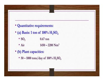
Quantitative requirements if you see, if you wanted to produce 1 ton of 100 percent sulfuric acid, then you need 0.67 tons of sulfur dioxide and air 1450 to 2200 normal cubic meters of air is required. Plant capacities, vary between 50 to 1000 tons per day of 100 percent pure H 2 SO 4 sulfuric acid.
