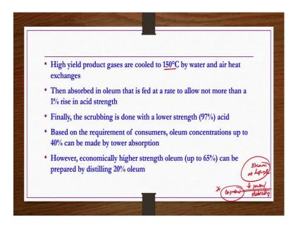
High yield product gases whatever are there after second stage or cold stage. They are cooled to 150 degree centigrade by water and air heat exchanges. Then, absorbed in oleum that is fed at a rate to allow not more than a 1 percent rise in acid strength.
