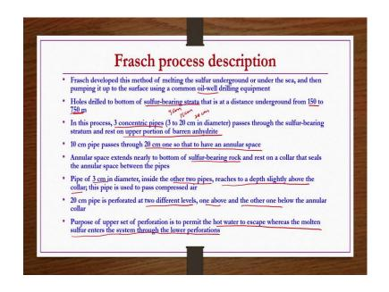
So, what is this process? First we see the description and then we see the same thing by pictorial form also. Frasch is a scientist who developed this method of melting the sulfur underground or under the sea and then pumping it up to the surface using a common oil well drilling equipment. How it is pictorially we are going to see anyway.
