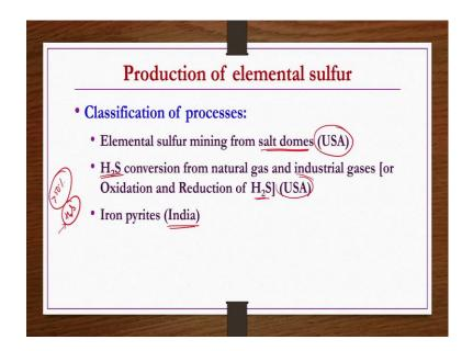
Primarily three methods are there elemental sulfur mining from salt domes. So, these are available or such process are very famous in America, Canada and some part of Europe. Then H 2 S conversion from natural gas and industrial gases or oxidation and reduction of H 2 S this process is also very much famous in USA and Canada and then European countries right.
