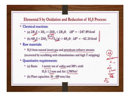
So, next process is elemental S by oxidation and reduction of H 2 S process. Chemical reactions if you see H 2 S reacting with the oxygen to give sulfur dioxide and then water. The sulfur dioxide may be further oxidized to give sulfur trioxide and then when the sulfur trioxide dissolved into water one can get the you know sulfuric acid, but what happens?
