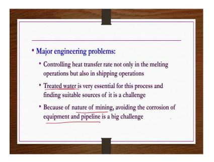
If you see the major engineering problems; obviously, what you understand the heat transfer rate heat transfer rate is very essential not only in the drilling area, but also in the you know shipping operation also because the drilling area because the sulfur rocks are there at different levels in different locations. Some are at just 150 meters distance some are even up to 700, 750 meters you have to drill. So, then; obviously, heat transfer calculations are going to be affected by the distance.
