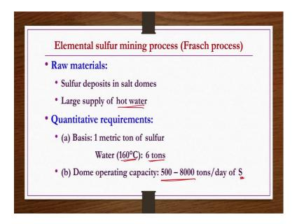
So, let us start with elemental sulfur mining process which is also known as the Frasch process. Raw materials: sulfur deposit in salt domes and then large supply of hot water is required. Because when you do the mining and then underground the mining wherever the sulfur rocks are found calcite sulfur containing rocks like calcite etcetera are found and what you have to do?
