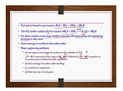
So, if you recapitulate what we have seen elemental sulfur recovery by oxidation of H 2 S process. H 2 S and air burned as per reactions this one first reaction A and then this SO 2 further oxidizes H 2 S by this reaction to give elemental sulfur S 6 in gases form. For above reaction two-stage catalytic converter with inter cooling and condensing provisions are often used.
