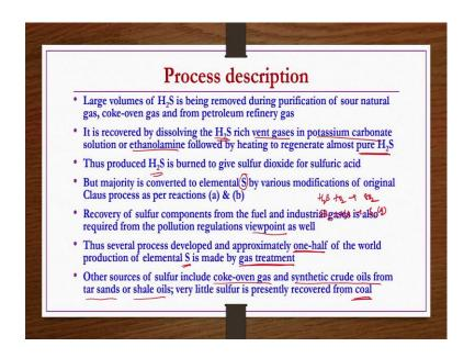
Process description if you see - large volumes of H 2 S is being removed during purification of sour natural gas, coke oven gas and from petroleum refinery gas. It is recovered by dissolving the H 2 S rich vent gases in potassium carbonate solution or ethanol amine solution followed by heating to regenerate almost pure H 2 S, right.
