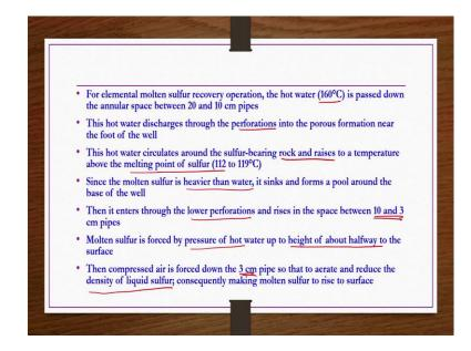
For elemental molten sulfur recovery operation the hot water approximately 160 degree centigrade is passed down the annular space between 20 and 10 centimeter pipes. This hot water discharges through the perforation into the porous formation near the foot of the well. This hot water circulates around the sulfur bearing rock and raises to a temperature above the melting point of sulfur between 112 to 119 degree centigrade.
