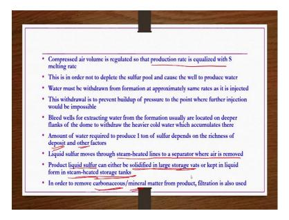
So, but basic principle what has to follow while doing this calculation that compressed air volume is regulated, so that production rate is equalized with sulfur melting rate. This is in order not to deplete the sulfur pool and cause the well to produce water. If you send the compressed air at a higher rate than the melting rate of the sulfur, then what happens?
