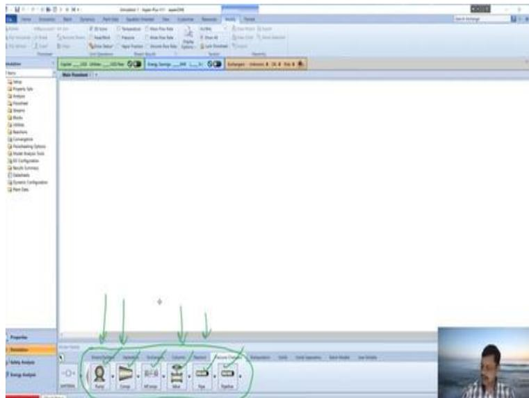
You will find the pressure changers block in Aspen simulation window over here. You have pump, compressor, multi-stage compressor, valve, pipe and pipeline. We will mostly cover this pump and compressor with some help of valve and pipe. Multi-stage compressor and pipeline they are for advanced users, so we will avoid these two in this lecture.
