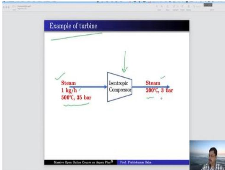
Now, we will take this example of turbine where the isentropic compressor model will be used as a turbine. The inlet to the turbine is steam flow rate 1 kg/hour and temperature 500-degree centigrade pressure is 35 bar. The outlet of the turbine is against steam with 200 degree centigrade and 3 bar pressure. So, the entire thermal energy will be converted into electrical energy and power will be generated through this turbine. So, we shall model this system.
