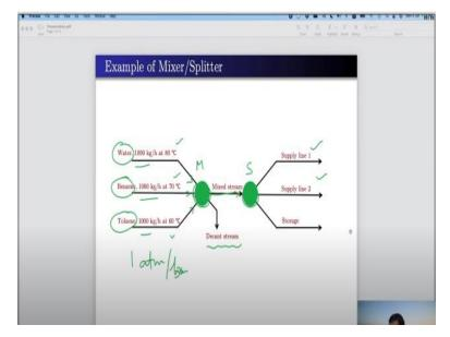
Here we find one mixer and one splitter. As you can notice that three streams are merging into this mixer, one is water, the benzene and toluene. For each one of them the flow rate is 1000 kg/hour and the temperatures are 80 degree centigrade, 70 degree centigrade and 60 degree centigrade respectively. The pressure has not been given in the problem but let us assume that the pressure is one atmosphere or one bar, whatever you use. So, they are mixed into this mixer.
