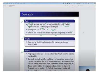
The next one is separators. There are three types of separators, flash, decanter and separator. In flash we have two types, flash 2 and flash 3. The flash 2 separates the feed into two outlets, one
