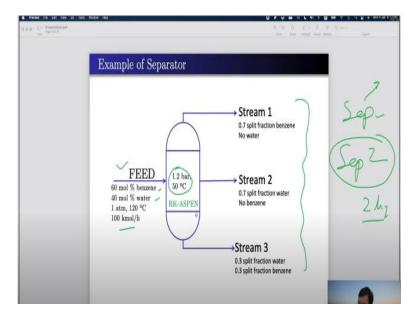
This example will have three outlet streams. So, we have only one feed and three outlet streams. The feed contains 60 mole % benzene, 40 mole % water and temperature and pressure given, the flow rate is also given. It will operate at this condition the separator. We will use RK-ASPEN. The stream one condition the split fractions are given. So, we want to operate this one. Now let us go to the Aspen Plus simulation window. Let us open a new simulation blank. Close the current one, do not save it.
