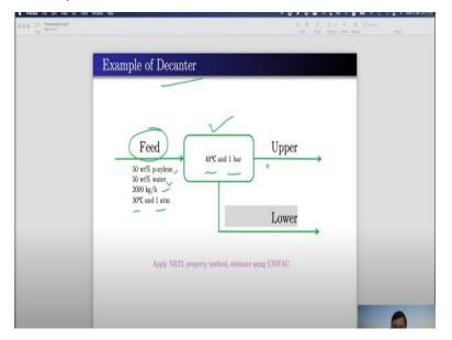
The next example is of a decanter. So as the name suggests the decanter always separates two liquids based on their density. That means the liquid with higher density will go through the bottom flow whereas the liquid with lower density will go through the top flow. So in this case we have a decanter over here we have a feed which contains 50% Para xylene, 50% water. Total flow rate is 2000 kg/hour and its temperature is 30 degree centigrade, pressure 1 atmosphere.
