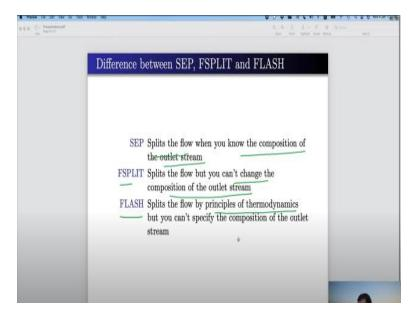
Now; one thing is common for Sep splitter and flash. All of them they FSPLIT the flow. But Sep splits the flow when you know the composition of the outlet stream. Not all but up to the degrees of freedom. While f split it also splits the flow but you cannot change the composition of the outlet flow. It is decided by the model equations. And flash this also splits the flow into vapour and liquid but it follows the principle of thermodynamics.
