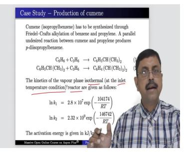
In today's lecture, we shall perform another case study that is on production of cumene. Cumene is actually another name for isopropylbenzene which can be synthesized through Friedel-Crafts alkylation reaction of benzene and propylene or propene. So, this is the main reaction and the desired reaction, reaction number 1 and the parallel undesired reaction between cumene and propylene produces p-diisopropylbenzene this one, this is undesired.
