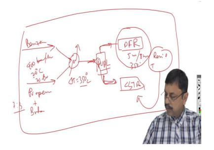
So, basically we have this benzene line, we have this propylene and butane line which is 7:3 ratios both of them are 400 kmol/hr 20 °C 20 bar pressure. They are mixed and heated where there is a temperature rise of 350 °C. So, actually it becomes 350 + 20, so, 370 °C alone. Then one needs to evaluate the performance of PFR and CSTR to find out the better equipment for cumene production.
