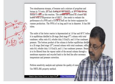
Some more information we have about the process, we have 2 simultaneous streams of benzene and a mixture of propylene and butane. So, we have one stream of benzene and another stream of propylene and Butane. Actually, benzene and propylene, they react with each other but butane is inert in this reaction. So, the mixture contains propylene and butane, in 7:3 ratios.
