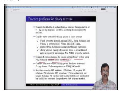
So, the answer to the query that has been asked in the question whether, change of pressure helps a separation of water acetonitrile azeotrope? The answer is yes, it helps. So, our next problem is comparing K values diagram for butane heptane binary system using Peng-Robinson and Lee-Kesler Plücker equation of state. So, for that again we have to go to the aspen simulation window.
