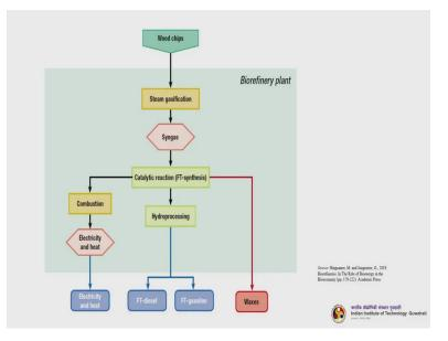
You can see this particular slide. So, this is one typical example from the wood chips. It is a biorefinery plant concept. So the wood chips goes to the steam gasification. So, you get syngas. So, syngas you catalytically convert using the Fischer Tropsch (FT synthesis basically). Then when it goes to combustion, we get electricity and heat. So you further process it (hydroprocessing basically). So, you get the Fischer Tropsch diesel and you get the Fischer Tropsch gasoline, fractionate them.
