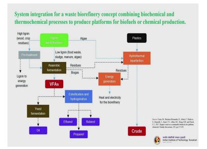
This is one last slide I wish to show you. So, this is the system integration for a waste biorefinery concept combining biochemical and thermochemical processes to produce platforms for biofuels and chemical products. So, have a look at the organic waste and biomass, if it is having algae, it goes to hydrothermal liquefaction, one of the most important technique will learn about this later on.
