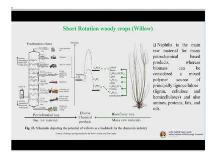
So, you can see this; if you compare it with the usual petro, Naphtha (crude oil basically), the same sort of things (products) you can get it from the biorefinery way using the willow. So, in petrochemical way one raw material and you get diverse chemical products, whereas, in a biorefinery way you have many raw materials and you get many different products. This is the beauty of the biorefinery concept.
