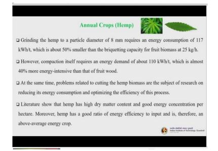
So, grinding the hemp to a particle diameter of 8 mm requires an energy consumption of 117 kilowatt hour per tonne, which is about 50% smaller than the briquetting capacity of fruit biomass at 25 kg per hour. However, compaction itself requires an energy demand of about 110 kilowatt hour per tonne, which is almost 40% more energy intensive than that of the fruit wood.
