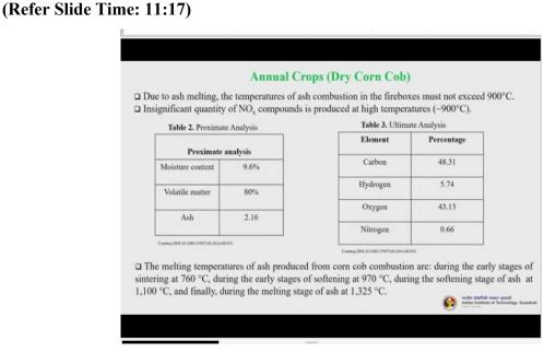
Then dry corn cob. So, due to ash melting, the temperatures of ash combustion in the fireboxes must not exceed 900 degrees centigrade. Insignificant quantity of  $NO_X$  compounds
