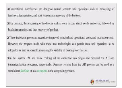
Conventional biorefineries are designed around separate unit operations such as processing of feedstock, fermentation and post fermentation recovery of the biofuels. For instance, the processing of feedstocks such as corn or corn starch needs hydrolysis, followed by batch fermentation and then recovery of product. These individual processes necessitate improved principal and operational cost and production cost.
