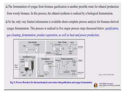
So, the fermentation of syngas from biomass gasification is another possible route for ethanol production from woody biomass. In this process, the ethanol synthesis is realized by a biological fermentation. So far only very limited information is available about complete process analysis for biomass derived syngas fermentation. Now, this process is realised in 5 major process steps discussed below or shown here.
