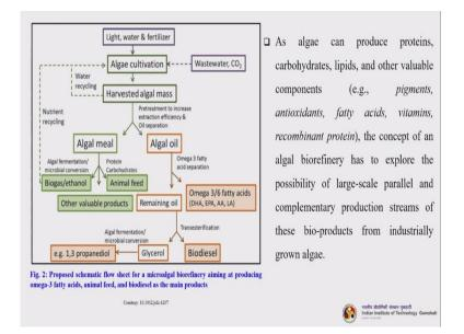
So, let us concentrate on this proposed scheme. So, this scheme talks about, this is the flow sheet for the microalgae biorefinery aiming at producing omega-3 fatty acids, animal feed and biodiesel as the main products simultaneously. So, algae grow with the presence of light, water and fertilizer or some nutrient source. While you are cultivating algae, so you can use wastewater and even carbon dioxide from different sources like power plants, the flue gas.
