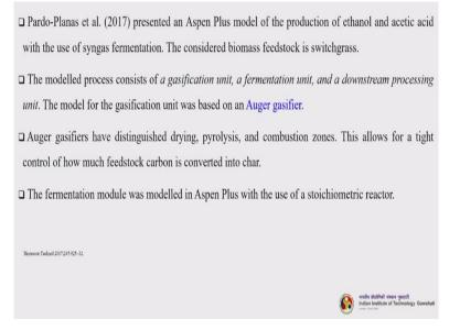
So, Pardo-Planas et al in 2017 presented an Aspen Plus model of the production of ethanol and acetic acid with the use of syngas fermentation. The reference is given below. The considered biomass feedstock is switchgrass. The modelled process consists of a gasification unit, a fermentation unit and a downstream processing unit. The model for the gasification unit was based on an Auger gasifier.
