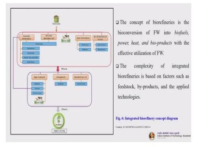
So, this is a slide where integrated biorefinery concept diagram using food waste as the substrate or feedstock has been presented. So, you can see that so food waste, so we can have anaerobic fermentation. We get biohydrogen, biomethane, biohythane, VFA the volatile fatty acids and biofertilizers the leftover. From microbial electrolysis cell also you get all these things. We can have animal feed the left out things.
