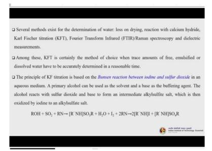
Several methods exist for the determination of water, so like loss on drying, reaction with calcium hydride, Karl Fischer titration which is the most adapted one, then Fourier transform infrared or Raman spectroscopy and dielectric measurements. Now among these the KFT or the Karl Fischer titration is certainly the method of choice when trace amounts of free emulsified or dissolved water have to be accurately determined in a reasonable time.
