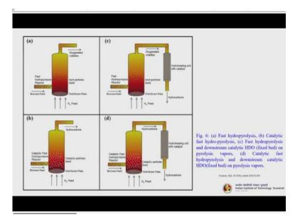
I will show you the schematic representation of these 4 systems what we have just mentioned. The first one. So, this is fast hydropyrolysis, here whatever you are seeing that is a pyrolyzer or pyrolysis reactor; the biomass is being fed and you use some sort of inner particles bed basically to carry out the fluidization, they are not catalyst. So, hydrogen is being fed and you get the oxygenated volatiles.
