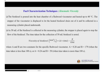
Then kinematic viscosity: The biodiesel is poured into the heat chamber of a Redwood viscometer and heated up to 40 degree centigrade. The stopper of the viscometer is displaced to let the heater biodiesel drain out of it and be collected in a measuring cylinder placed underneath. As 50 ml of the biodiesel is collected in the measuring cylinder the stopper is placed again to stop the flow of the biodiesel.
