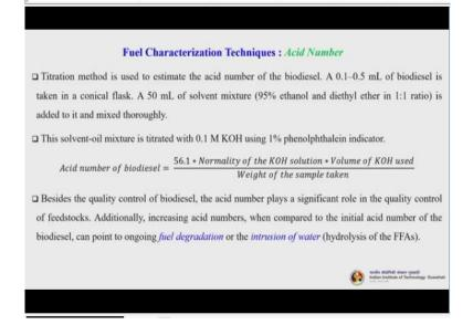
So, we will see one by one. The first is acid number. Titration method is used to estimate the acid number of the biodiesel. Usually 0.1 to 0.5 ml of biodiesel is taken in a conical flask. A 50 ml of the solvent mixture which is usually 95% ethanol and diethyl ether in 1 : 1 ratio is added to it and mixed thoroughly. Now this solvent oil mixture is titrated against 0.1 molar KOH using a 1% phenolphthalein indicator.
