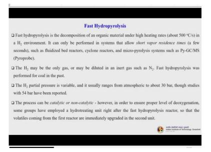
We will now discuss about fast hydropyrolysis. Fast hydropyrolysis is the decomposition of an organic material under high heating rates almost about 500 degree centigrade per second in a hydrogen environment. It can only be performed in systems that allow short vapour residence time, few seconds only, such as fluidized bed reactors, cyclone reactors, micro pyrolysis systems such as the Py-GC/MS (Pyroprobe).
