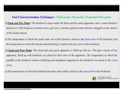
So, then we will talk about the flash point, fire point, cloud and pour point. These are very important properties for any liquid fuels. So, flash and fire point: the biodiesel is kept inside
