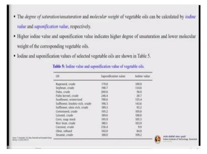
So, we will move ahead. So, the degree of saturation/unsaturation and molecular weight of vegetable oils can be calculated by two things, first is something called an iodine value and second is called saponification value (respectively). Now higher iodine value and saponification value indicates higher degree of unsaturation and lower molecular weight of the corresponding vegetable oils. Iodine and saponification values of selected vegetable oils are shown in the table 5.
