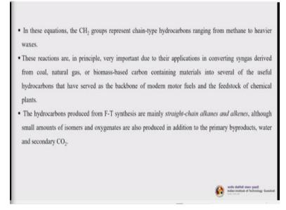
Now, in these equations the CH<sub>2</sub> group represent the chain type hydrocarbons ranging from methane to heavier waxes. These reactions are in principle, very important due to their applications in converting syngas derived from coal, natural gas or biomass based carbon containing materials into several of the useful hydrocarbons that has served as the backbone of modern motor fuels and the feedstock of chemical plants.
