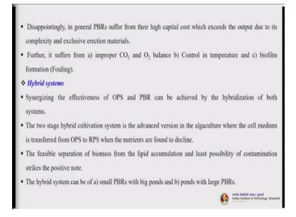
Disappointingly, in general photobioreactors suffer from their high capital cost (this is one of the most important thing actually which hinders its application in large commercial sector) which exceeds the output due to it is complexity and exclusive erection materials. Further, it suffers from improper carbon dioxide and oxygen balance, control in temperature and biofilm formation - fouling.
