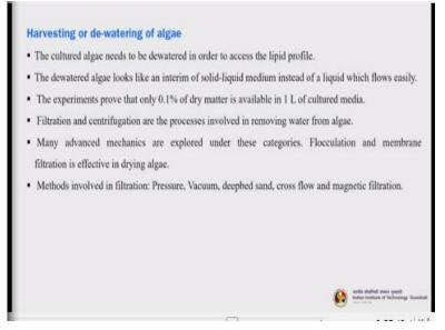
Then harvesting or dewatering of algae. The cultured algae needs to be dewatered in order to access the lipid profile. The dewatered algae looks like an interim of solid-liquid medium instead of a liquid which flows easily. The experiments prove that only 0.1% of dry matter is available in 1 litre of the culture media. Filtration and centrifugation are the processes involved in removing water from algae.
