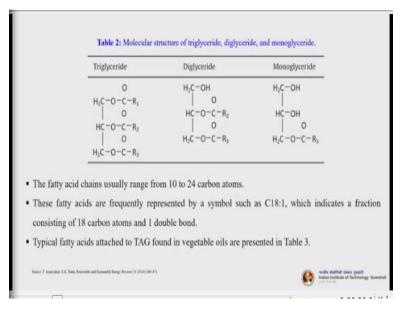
Now this table will give you the understanding about the molecular structure of the triglyceride, diglycerides and monoglyceride. So, the fatty acid chains usually range from 10 to 24 carbon atoms. These fatty acids are frequently represented by a symbol such as C18:1, which indicates that a fraction consists of 18 carbon atoms and 1 double bond. So, typical fatty acids attached to TAG found in vegetable oils are presented in the table 3.
