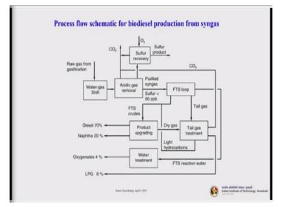
So, this is an interesting process flow schematic for the biodiesel production from the syngas. So, the raw gas from the gasification unit that is coming - it goes to the water gas shift reaction. Then it goes to the acidic gas removal where carbon dioxide has been removed and you can have the sulfur recovery coupled with that carbon dioxide removal process. And part of the carbon dioxide also can be recycled back to other processes like this tail gas treatment.
