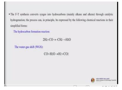
So, the FT synthesis converts syngas into hydrocarbons mainly alkane and alkene through catalytic hydrogenation; the process can in principle be expressed by the following chemical reactions in their simplified forms:
