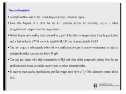
So, we will try to understand the process in a better way. Let us go through it. So, a simplified flowchart of the Fischer Tropsch process that is what we have already seen it. From this diagram, it is clear that the FT synthesis process for processing syngas is rather very straightforward
