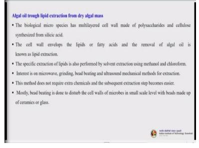
So, then algal oil through lipid extraction from dry algal mass. The biological micro species has multilayered cell wall made up of polysaccharides and cellulose synthesized from silicic acid. The cell wall envelopes the lipid or fatty acids and the removal of algal oil is known as that lipid extraction. The specific extraction of lipids is also performed by solvent extraction using methanol and chloroform.
