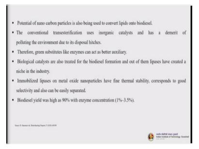
Potential of nano carbon particles is also being used to convert lipids onto biodiesel. The conventional transesterification uses inorganic catalyst and has the demerit of polluting the environment due to it is disposal hitches. Therefore, green substitutes like enzymes can act as a better auxiliary. Biological catalysts, which are treated for the biodiesel formation and out of them lipases have created a niche in the industry.
