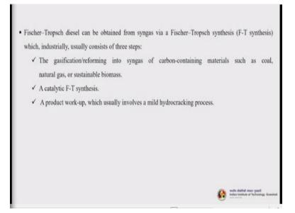
So, FT diesel can be obtained from syngas via the Fischer Tropsch synthesis process which industrially usually consist of 3 steps. The first is the gasification or reforming into syngas of the carbon containing materials such coal, natural gas or sustainable biomass. Second is the catalytic Fischer Tropsch synthesis. The third: a product work-up, usually involves a mild hydrocracking step.
