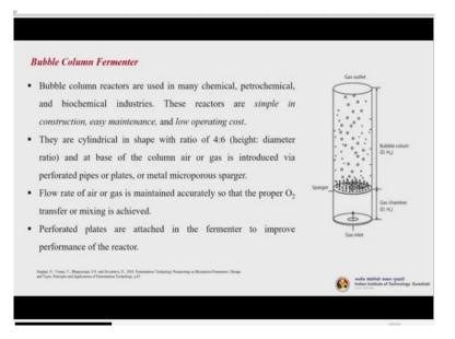
So, the next is bubble column fermenter. So, these are very classical reactors, which are used in many chemical, petrochemical and biochemical industries. Now, these reactors are simple in construction, they are easy to maintain and they have low operating costs. So, these are cylindrical in shape with a ratio of 4 is to 6 : height to diameter ratio basically and at the base of the column air or gas is introduced via perforated pipes or plates or metal microporous sparger.
