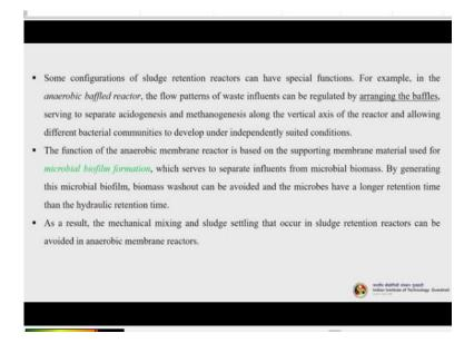
Some configurations of sludge retention reactors can have special functions. For example, in the anaerobic baffled reactor, the flow patterns of waste influents can be regulated by arranging the baffles, serving to separate acidogenesis and methanogenesis along the vertical axis of the reactor and allowing different bacterial communities to develop under independently suited conditions.
