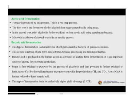
So, the next one is acetic acid fermentation. Vinegar, which is one of the most widely used product, in the food and beverage and this one restaurant industries is produced by this process. So, this is a 2 step process. The first step is the formation of ethyl alcohol from sugar anaerobically using yeast and in the second step ethyl alcohol is further oxidized to form acetic acid using acetobacter bacteria. Now microbial oxidation of alcohol to acid is an aerobic process.
