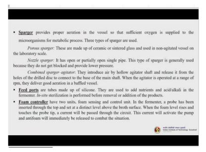
So, sparger provides proper aeration in the vessels so that sufficient oxygen is supplied to the microorganisms for metabolic process. Three types of spargers are used porous spargers, nozzle spargers and combined spargers and agitator. In the porous spargers these are made up of ceramic or sintered glass and used in non-agitated vessel on the laboratory scale. Nozzle sparger has opened or partially open single pipe.
