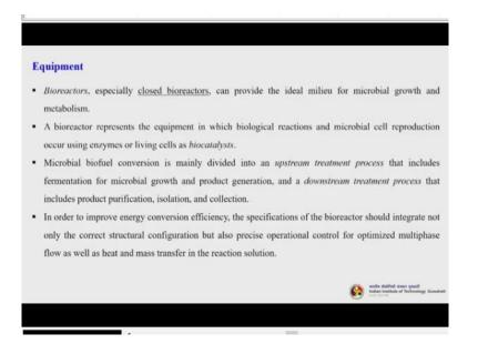
Now, let us understand the different equipments, those are essentially required to accomplish the microbial conversion processes. So, bioreactors, especially are closed bioreactors can provide the ideal milieu for the microbial growth and metabolism, because why we are talking about closed bioreactors, because we can easily control all the parameters in a closed system.
