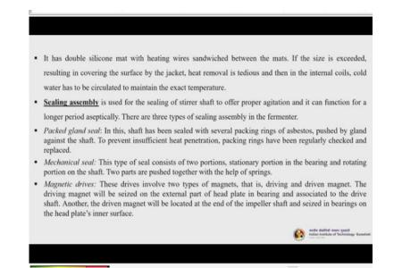
So, it has doubled silicon mat with heating wires sandwiched between the mats. Now, if the size is exceeded, resulting in covering the surface by the jacket heat removal is tedious and then in the internal coils cold water has to be circulated to maintain the exact temperature, it is always easy if you have an outside temperature control. Now, that is possible only when you have a smaller reactors or fermenters.
