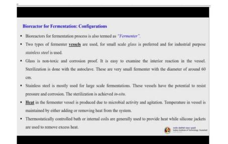
Let us understand the bioreactors for fermentation. So, their configuration. So, bioreactors for fermentation process are also termed as fermenters. Two types of fermenter vessels are used. So, the small scales are usually made up of glass and for the industrial purposes, we use stainless steel. So, glass is non toxic and corrosion proof, it is easy to examine the interior reaction what is happening inside the vessel.
