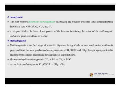
Now acetogenesis, this step employs acetogenic microorganisms catabolizing the products created in a acidogenesis phases into acetic acid CH<sub>3</sub>COOH, carbon dioxide and hydrogen. Now acetogens finalize the breakdown process of the biomass facilitating the action of the methanogenic archaea to produce methane as biofuel.
