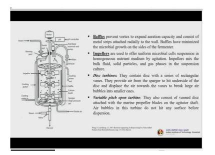
Now, let us see this particular schematic representation of a usual fermenter, it can be a lab scale fermenter, it can be industrial scale fermenter. Let us see. So, you can see that this is the reactor: there is a motor and this is the impeller. This is the impeller; you can see these are the small plates which are there. So, please understand that impellers there are so many different types of impeller designs are available, it is not that only this has to be used, this is a particular design.
