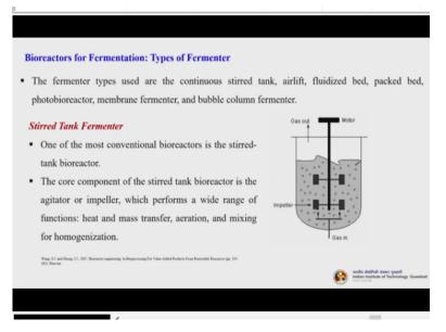
Now let us discuss about the types of fermenters. We will quickly discuss about the basics of the few fermenters which are essentially adapted in the lab scale as well as commercial scale. There are many types. So, the first one is the continuous stirred tank reactor, then we have airlift reactor, we have fluidized bed reactor, we have packed bed reactors, we have photobioreactors, membrane fermenters and bubble column fermemter.
