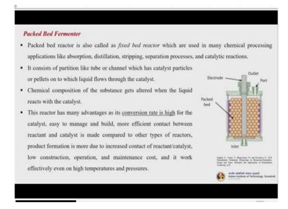
So, the next is packed bed fermenter. Now, packed bed fermenter reactors are also called as fixed bed reactors, which are used in many chemical processing applications like absorption, distillation, stripping, separation processes and catalytic reactions. It consists of partition like tube or channel which has catalytic particles of pellets on to which liquid flows through the catalyst.
