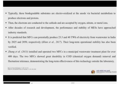
Typically, these biodegradable substances are electro-oxidized at the anode via bacterial metabolism to produce electrons and protons. Then the electrons are conducted to the cathode and are accepted by oxygen nitrate and metal ions. After decades of research and development, the performance and stability of MES have approached industry standards. It is predicted that MFCs can potentially produce 23.3 and 40 terawatt hour of electricity from wastewater in India by 2025 and 2050 respectively.
