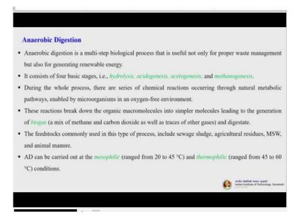
So, we will see all of these briefly. So, first one is anaerobic digestion. Now, anaerobic digestion is a multi-step biological process that is useful not only for proper waste management, but also for generating renewable energy. It consists of 4 basic stages: hydrolysis, acidogenesis, acetogenesis and methanogenesis. Now, during the whole process, there are a series of chemical reactions occurring through natural metabolic pathways enabled by microorganisms in an oxygen free environment.
