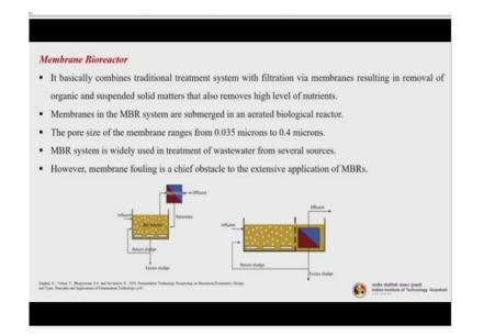
So, next is these are latest development in the environmental and energy sites actually the membrane bioreactors. So, it basically combines traditional treatment with filtration via membranes, resulting in the removal of organic and suspended solid matters that are also removes high level of nutrients. Now, membrane bioreactor systems are submerged in an aerated biological reactor. The pore size of the membrane ranges from 0.035 microns to 0.4 microns.
