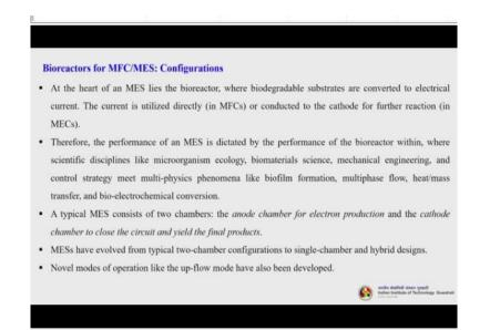
So, then we will talk about the bioreactors for microbial fuel cell and microbial electrolysis systems their configurations. At the heart of an MES lies the bioreactor where biodegradable substrates are converted to electrical current. The current is utilized directly in the MFCs or conducted to the cathode for further reaction in case of the MECs.
