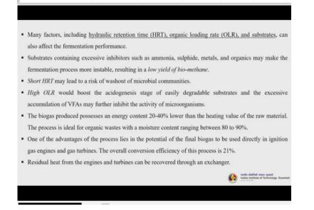
Many factors including hydraulic retention time, organic loading rate and substrates can also affect the fermentation performance. Now, substrates containing excessive inhibitors such as ammonia, sulphide, metals and organics may make the fermentation process more instable resulting in a low yield of bio-methane.
