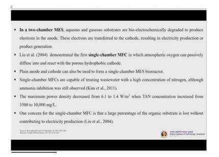
In a 2 chamber MES aqueous and gaseous substrates are bioelectrochemically degraded to produce electrons in the anode, these electrons are transferred to the cathode resulting in electricity production or product generation. Liu et al demonstrated the first single chamber MFC in which atmospheric oxygen can passively diffuse into and react with the porous hydrophobic cathode.
