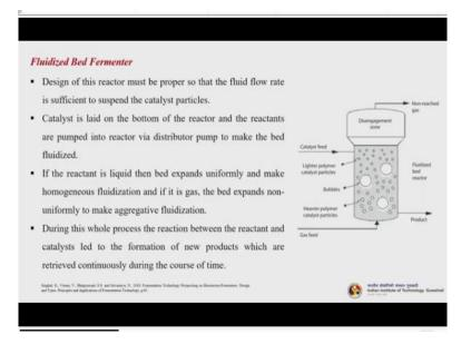
So, the next is another class of fermenters which are also industrially used and adapted. So, are called fluidized bed fermenters. Now, design of the reactor must be proper so that fluid flow rate is sufficient to suspend the catalyst particles. So, catalyst is laid on the bottom of the reactor and the reactants are pumped into reactor via distributor pump to make the bed fluidized.
