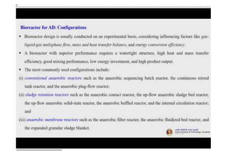
So, let us now discuss about the bioreactors for anaerobic digestion and their configurations. Bioreactor design is usually conducted on an experimental basis considering influencing factors like gas-liquid-gas multiphase flow, mass and heat transfer balance and energy conversion efficiency. A bioreactor with superior performance requires a watertight structure, high heat and mass transfer efficiency, good mixing performance, low energy investment and high product output.
