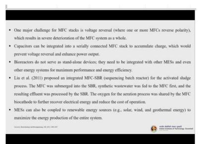
One major challenge for MFC stacks is voltage reversal. When one or more MFCs reverse polarity. So, this results in severe deterioration of the MFC system as a whole. Capacitors can be integrated into a serially connected MFC stack to accumulate charge, which should prevent voltage reversal and enhance power output. So, bioreactors do not serve as stand-alone devices, they need to be integrated with other MES and even other energy systems for maximum performance and energy efficiency.
