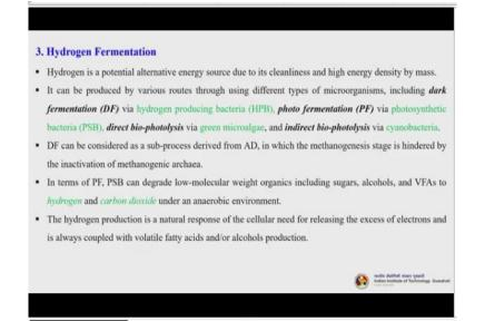
The next is hydrogen fermentation. Now, hydrogen is a potential alternative energy source due to its cleanliness and high energy density by mass. It can be produced by various routes through using different types of microorganisms, including dark fermentation via hydrogen producing bacteria, photo fermentation via photosynthetic bacteria and direct bio-photolysis using green microalgae or indirect bio-photolysis using cyanobacteria.
