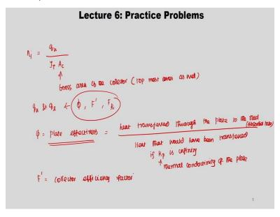
After doing that we are going to calculate instantaneous efficiency which is nothing but q u upon I T into A c this A c is nothing but grass area of the collector which includes the topmost cover as well. In calculating this q u and q l we might require certain other parameters which are phi F
