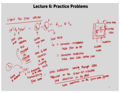
So before going into that details of given data we are going to see certain parameters whatever we learnt in lecture 4 flat plate collector. Whatever the plate area into this is solar radiation Flux observed on absorber plate. So this is plate area which is equivalent to q u + q l what is q u this is nothing but useful heat gained what is that? That is nothing but rate of heat transfer to the working fluid then this is q l which is nothing but heat losses.
