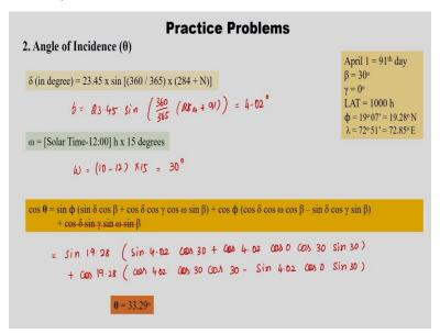
And then using this we would be calculating delta which is declination angle 23.45 sin 360 upon  $365\ 284 + 91$ . So if you call it this would come around 4.02 degree. So omega is solar time that is  $10\ -12$  into 15 since it is in the morning it should be in plus so 30 degree then substitute the same and  $19.2\ \sin 4.02\ \cos 30 + \cos 4.02$  and the collector is facing due south.
