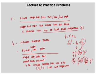
Which is defined as actual useful heat gain rate per tube per unit length upon gain, gain in the sense useful heat gain that would have been gained by gained if absorber plate was at local fluid temperature local fluid temperature F dash is actually useful head gained rate per tube per unit length to useful head gained that would have been gained if absorber plate was at local fluid temperature which is nothing but T f.
