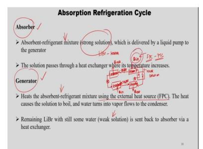
That is what is being done in absorption refrigeration cycle. So, here there are 4 components absorber, generator and condenser and then evaporator. So, if you see here absorber this is the new one here and generator is new one here otherwise same operator condenser pretty much similar. In absorber, the absorbent refrigerant mixture usually a strong solution of salt and water they are not common absorption mixture uses Li Br lithium bromide, salt and water solution.
