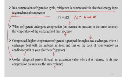
So, the next one is we are going to see the solar cooling cycle. Before going into solar cooling cycle we will see what compression refrigeration cycle, how it works is and which component is replaced by solar energy. In compression refrigeration cycle that refrigerant is compressed via electrical energy input into your mechanical compressor. So, it works based on this ideal gas law principle, P is proportional to T at constant V.
