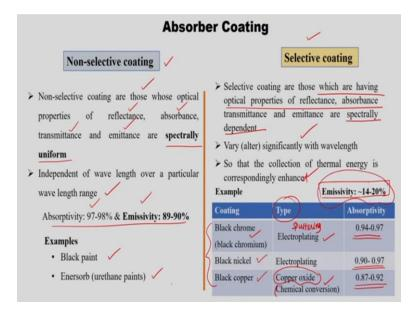
The first one absorber coating, we are going to see the 2 main categories are non-selective coating and selective coating, the difference between these 2 is in non-selective coating, so, we do not differentiate the properties of reflectance, absorbance, transmittance and emittance based on any spectral variation. So that means, the properties of reflectance absorbance, transmittance emittance are spectrally uniform.
