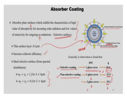
The next we are going to see the definition of selective surfaces. So, absorber plate surfaces s which exhibits the characteristics of high value of absorptivity for incoming solar radiation and low values of emissivity for outgoing re-radiation. So, those were called selective surfaces. So, if you see here, so, this is the steel tube, this is inner wall, outer wall. So, outer wall of the steel tube is given with the solar selective absorbing coating.
