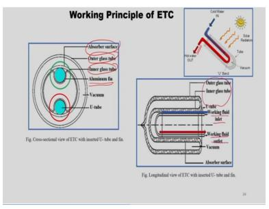
Working principle of ETC is same. So, here you have a glass cover you have an absorber tube. Absorber tubes coated with the selective coating material and to remove this air in between these 2 tubes, the 2 ends are closed and vacuum is maintained between the 2 tubes. So, here if you see this is the absorber surface that is outer surface of the inner glass tube, this is outer glass tube which is nothing but a glass cover inner glass tube which is nothing better absorber.
