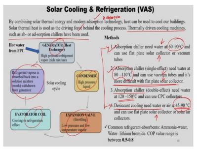
So, by combining the solar thermal energy and modern adsorption technology or absorption technology as well as heat can be used to cool our building. Solar thermal heat is used as the driving force behind this cooling process thermally driven cooling missions such as adsorption or absorption chillers have been used. Nowadays, if it is an adsorption chiller, it needs water at 60 to 90 degree. So, we can use flat plate collector or vacuum tubes which is nothing but ETC.
