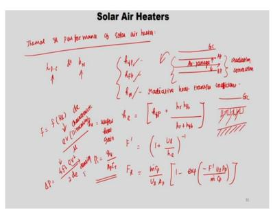
So, if we want to discuss about the thermal and performance analysis of solar air heater. We can see not in detail, but briefly there we used h pc and h w. So, this is for outside surrounding air, this is heat transfer coefficient between plate and cover system. So, here also we use 2 heat transfer coefficient h fp and h fb. So, what is p? This is the absorber plate. So, this is the bottom plate and in between the air is flowing.
