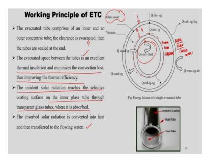
So, next what we are going to see is evacuated tube collector? The evacuated tube comprises of an inner and an outer concentric tube: the clearances evacuated, so then the tubes are sealed at the end. So, this is the arrangement where you where fluid is flowing inside the inner tube. So, this is inner tube, so, this is outer tube. So, in between there is a vacuum the air gap in between the inner tube and outer tube is totally evacuated.
