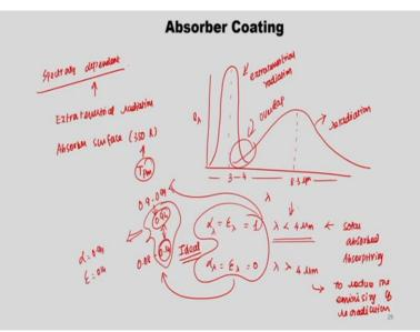
So, this variation of selective coating so, we said that they are spectrally dependent. So, the research says that how do we first select that spectrally dependent variation. So, there are 2 things to be considered one is normal extra-terrestrial radiation; the second one is the absorber surface. So which is about 350 Kelvin plate temperature, this is the normal plate temperature we would get in the absorber plate.
