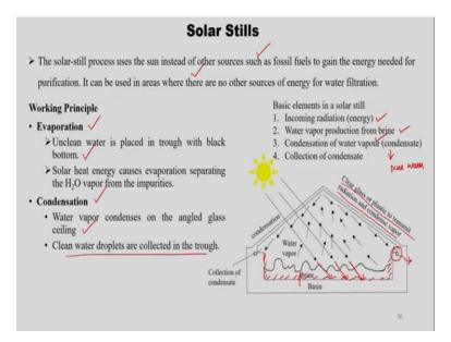
The second major application is solar stills. So it is being used for water purification. The solar still process uses the sun instead of other sources such as fossil fuels to gain the energy needed for purification, it can be used in areas where there are no sources of energy for water filtration and the basic elements are incoming solar radiation and water vapor production from brine and condensation of water vapor. So, this is a pure water and collection of condensate.
