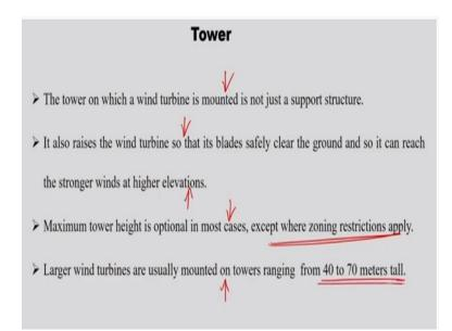
So tower is nothing but on which wind turbine is mounted and is not just a support structure it also raises the wind turbine so that it blades safely clear the ground and so it can reach the stronger wind at the higher elevations. So that is not only support structure it also helps in getting more wind power maximum tower height has optional in most cases except where zoning restrictions apply this also we have seen during the obstacles sections of the zones.
