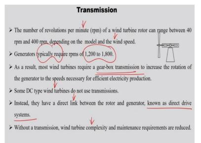
The transmission line the number of revolutions per minute of a wind turbine rotor can range between 40 to 400 rpm depending on the model and the wind speed. But generator typically the require rpms of around 1200 to 800 so which can help us that is nothing but a gear box transmission to increase the rotation of generator to the speed necessary for efficient energy protection.
