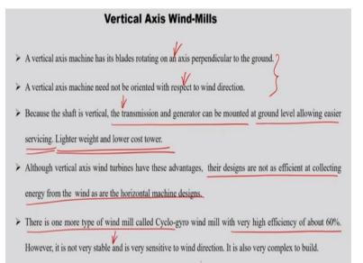
In vertical axis machine they are having their blades rotating on an axis perpendicular to the ground and vertical axis machine need not to be oriented with respect to wind direction. This we have already seen and because the shaft is vertical that transmission and generator can be mounted at the ground level allowing easier servicing. So for horizontal machine you suppose to keep it in the higher height with the supporting structure.
