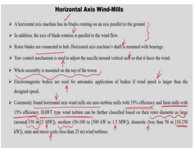
In horizontal axis wind mills this horizontal axis machine as is blades rotating on an axis parallel to the ground. In addition axis of blade of rotation is also parallel to the wind flow these 2 points we have already seen the rotor blades are connected to hub you know what is hub by now. And horizontal axis machine shafted with bearings the yaw control mechanism is used to adjust the nacelle around vertical axis so that it faces the wind.
