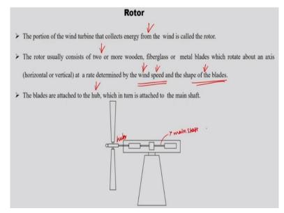
And this is again few points about the various components of the horizontal axis wind machine. So the rotor is the portion of the wind turbine that collects energy from the wind is called rotor. And the rotor usually consist of 2 or more wooden fiber glass or metal blades which rotate about axis horizontal or vertical based on the wind mill at a rate determined by the wind speed and the shape of the blades.
