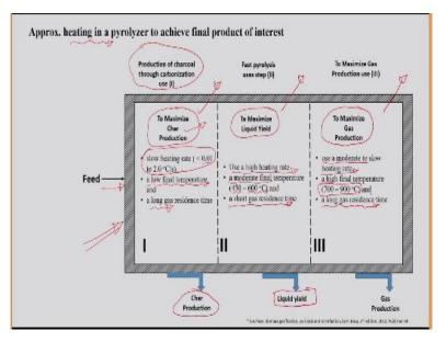
After learning the types of pyrolysis operation in the pyrolyzer, the pyrolysis of the carbonaceous material is carried out using a specific operating condition to meet the requirement of the final product of the interest. So, here one schematic has been shown, which is represented in the form of different stages that is stage one, stage 2 and the stage three.
