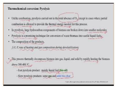
Unlike combustión process, the pyrolysis process it is carried out in total absence of oxygen. Except in some cases, where partial combustion is allowed to provide the thermal energy which is required for the process. So, by partially combusting the char and the gas during the pyrolysis process, it can provide the thermal energy which is required for the process, because the pyrolysis process is a endothermic reaction.
