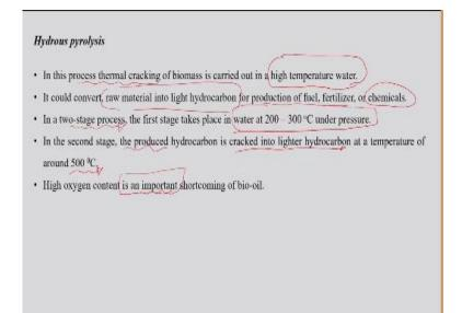
Whereas, in case of the hydrous pyrolysis, the thermal cracking of the biomass is carried out in a high temperature water. So, here the medium is high temperature water whereas, in the previous case, the process is carried out using a hydrogen as a medium. So, it could convert a raw material into the light hydrocarbon for the production of the fuel as well as fertiliser and chemical as a product.
