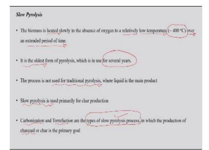
Now, the slow pyrolysis process. In case of the slow pyrolysis process, the biomass is heated slowly in the absence of oxygen to a relatively low temperatura. And in this case the temperature is relatively low over an extended period of time. Because, as we already discussed earlier, the product of interest in the slow pyrolysis process is the char. So, as a result, it allows the heating over extended period of time.
