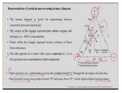
And the ternary diagram here, it is useful for representing the biomass conversion processes. And here our focus of interest is on the pyrolysis process. So the ternary diagram which is shown here, it mainly discusses about the pyrolysis process. Apart from that, the ternary diagram can also be used to represent the other biomass conversion processes that is the gasification as well as the combustión.
