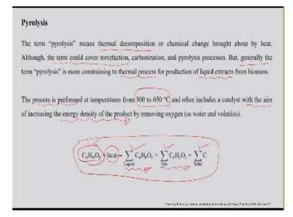
The term pyrolysis means the thermal decomposition or chemical change brought about by heat. The term pyrolysis could cover the torrefaction, carbonization and the pyrolysis process as well. If you recall our discussion about torrefaction and the carbonization process, so, torrefaction process is also carried out in absence of oxygen, but in a very narrow temperature range.
