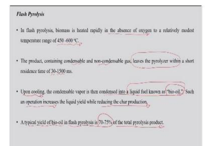
In case of flash pyrolysis the biomass is also heated rapidly in absence of oxygen, but to relatively a modest temperature around like 450 to 600 degree C only. The product containing condensable, non condensable gases leaves the pyrolyzer within a short residence time of around 30 to your 1500 milliseconds. So, in this case, the gases are not allowed to stay for a longer period of time inside the reactor.
