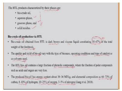
So, the hydrothermal liquefaction of the biomass and the product produced from the hydrothermal liquefaction of biomass are categorised based on their phases. That is the biocrude oil phase, aqueous phase, gaseous phase and solid residue as the product. So, the biocrude oil which is obtained from the HTL process is a dark brown and the viscous liquid consisting around 18 to 67 % of the total weight of the feedstock.
