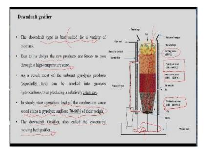
So, first is the down draft gasifier. So, if you see here, this is the schematic of the down draft gasifier where the biomass is fed inside the gasifier from the top. And if you see here, this particular gasifier is divided into 4 zones that is the drying zone, pyrolysis zone, this is the oxidation zone and reduction zone. So, as I said, the gas produced in this particular gasifier is forced to pass through the high temperature zone.
