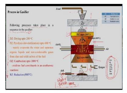
After understanding the gasification, let us see how the process of gasification it takes place in the gasifier. So, if you see this particular schematic here, the gasifier is divided into 4 zones that is dry zone, pyrolysis zone, this is the oxidation zone and this is the reduction zone. So, the producer gas in the gasifier is formed by partial combustion of the solid biomass in a vertical flow back bed.
