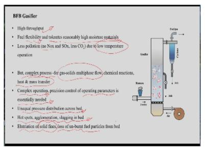
These represent the bubbling fluidized bed gasifier and this particular part here it represented the bubbles which are formed in the gasifier. So, in this case, if you see here, this kind of gasifier also achieve a high throughput and can operate on any kind of biomass material and tolerate reasonably high moisture material as well. The less pollution again in terms of NOx, SOx and CO 2, because of the low temperature operation in the bubbling fluidized bed gasifier.
