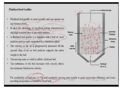
So, this is the schematic of the fluidized bed gasifier. So, the fluidized bed gasifier is considered as the most versatile and it can operate on any biomass form. And that is what is the advantage of the fluidized bed gasifier. It takes the advantage of excellent mixing characteristics and high reaction rates of gas solid mixture in the gasifier. A fluidized bed gasifier is a chamber with a bed of inner sand particles, which are supported by the distributor plate.
