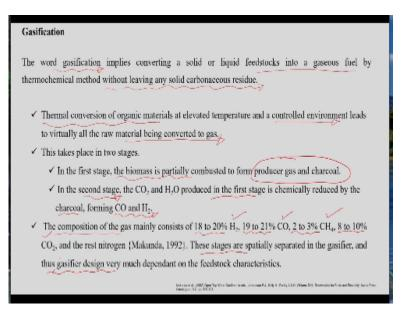
So, let us discuss about this gasification technology in more detail. So, what is gasification? The word gasification, it implies converting a solid or liquid feedstock into gaseous fuel by thermo-chemical method without leaving any solid carbonaceous residue inside the reactor. And the thermal conversion of organic material at elevated temperature and control environment, it leads to virtually all the raw material being converted to gas.
