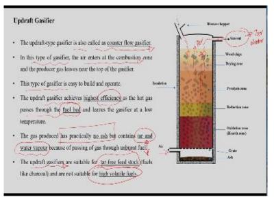
So, the up draft gasifier is also called as a counter flow gasifier. Because in this case, the biomass is also fed from the top and the producer gas is drawn off from the top of the gasifier here. So, in this type of gasifier, the air enters at the combustion zone. So, this is the entry of the air in the combustion zone here and produce gas leaves from the top of the gasifier as shown here.
