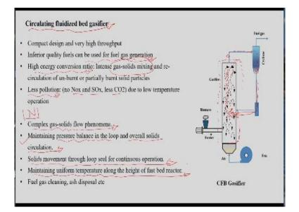
So, this is a schematic of the circulating fluidized bed gasifier. Where if you see here, the circulating fluidized bed design is a very compact and it achieves a high throughput as well. And inferior quality fuels can also be gasified to generate the fuel in the circulating bed fluidized gasifier. High energy conversion ratio because of the intense gas solid mixing which is taking place in the circulating fluidized bed gasifier recirculation of the unburned fuel back into the gasifier.
