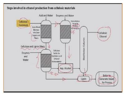
However, if you discuss the ethanol production from the non-edible feedstock, now, the number of operations required in this process are relatively higher than that of the edible feedstock. Let us see the example of the cellulosic feedstock here. So the cellulosic material first need to be pretreated so that it can separate the hemicellulose fraction from the cellulose fraction here.
