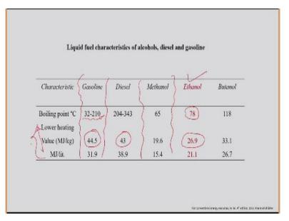
So, if you just try to compare these properties of the liquid fuel with alcohol, that is mainly the methanol and the ethanol, we can see that the boiling point in case of the ethanol is in one temperature, because ethanol is a single chemical. Whereas, in case of the fuel, it has a wide range of the chemical compound as a result, its boiling point is also having a certain wide range which varies from this particular range.
