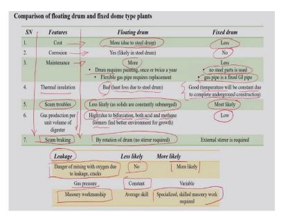
So, if you just now try to compare the floating drum and the fixed dome type biogas plant, so there are different features are listed here, by which we can compare the operation of these 2 particular plants. So, if we just talk about the cost at the beginning, so, cost involved in the construction of floating drum type of biogas plant is more and in the fixed drum, it is less. Why? Because in this particular construction, the steel drum is required.
