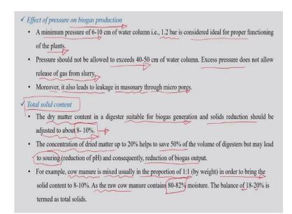
Minimum pressure of around like 6 to 10 centimeter of water column is essential in the digester. So, that means, like around this much bar 1.2 bar is considered as ideal for the proper functioning of a plant. And pressure should not be allowed to exceeds 40 to 50 centimeter of water column. Why?
