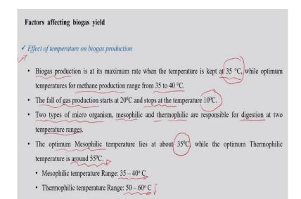
So, now, if we just talk about the effect of temperature first, temperature is a very important factor for the efficient bio digestion of the organic matter. Because, when we talk about the temperature, so, the gas production is reaches to its maximum value, when the temperature is maintained at around like 35 degree C in the digester. While the optimum temperature for the methane production, it is in the range of like 35 to 40 degree C.
