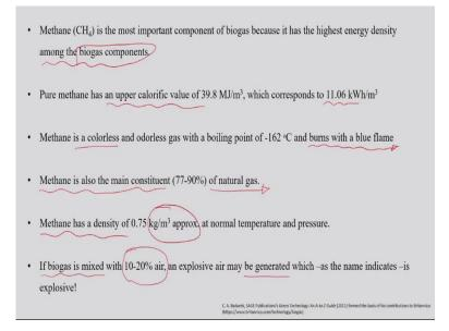
As I mentioned, the methane is the most important component of the biogas because methane is the only gas which has the highest energy density among the other gases present in the biogas. Apart from that, the pure methane has an upper calorific value of around 39.8 megajoule per meter cube. And it corresponds to around 11.06 kilowatt hour per meter cube of a gas.
