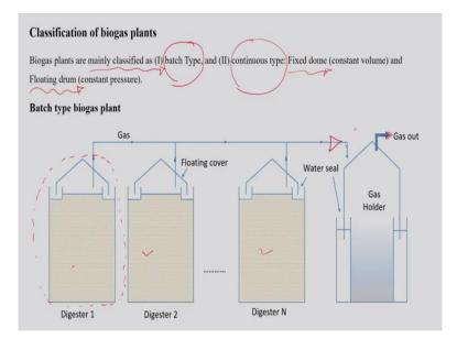
Now, based on these advantages as well as the importance of this particular process, let us discuss about in details, how this particular process carried out or what type of biogas plants are being used for the digestion purpose. The biogas plants are mainly classified as batch type and the continuous type plant. And continuous type plants are further sub classified as fixed dome type plant and the floating drum type plant.
