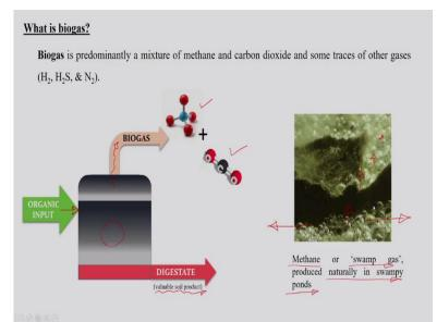
So, biogas is predominantly a mixture of methane and carbon dioxide and some traces of other gases such as H2, H2S and the nitrogen. So, the biogas is produced mainly by decomposition of the organic matter in a digester. So, this particular digestion process is carried out by the action of the microorganism in absence of oxygen. So, the biogas produced during this particular stage may act as a source of renewable energy as well.
