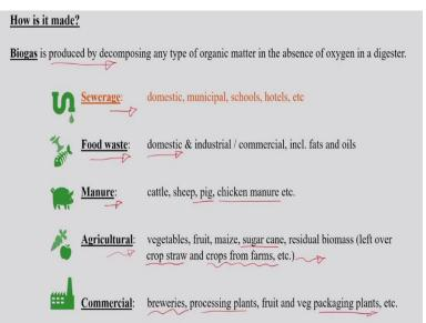
So, how it is made? So, the biogas says it is produced by decomposing any type of organic matter by the action of microorganism in absence of oxygen. So, the organic matter may be it in the form of sewerage. So, if you see here it may be a domestic, municipal, school or hotels. The sewerage of these particular sources which contains some organic materials can be digested to produce the biogas.
