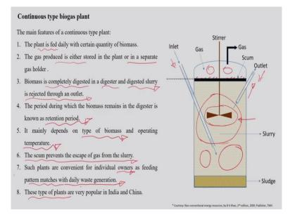
And this is how is the difference between the continuous and the batch type of biogas plant, because in the batch type of plant, as I mentioned, the amount of biomass is fed at a interval. So, first batch if it is fed today, so, once the digestion of this particular batch is over, we cannot fed another batch in between. So, once this particular digestion process is completed, then the best type of plant is emptied to recover the digested slurry.
