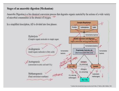
That means the anaerobic digestion is mostly a biochemical conversion process, and that degrades the organic matter in absence of oxygen by the action of wide varieties of the microorganism. So, if you just try to simplify this particular concept, so you can see that this anaerobic digestion process is carried out in 4 different stages. That means first is the hydrolysis stage, then the acidogenesis, acetogenesis and then the methanogenesis.
