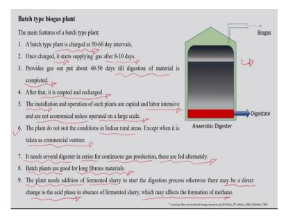
So, let us see some important feature of such kind of unit. So, a batch type of plant is charged at 50 to 60 days intervals. So, if it is a single unit, it is charged at 50 to 60 days interval. And once it is charged, it starts to produce gas after 8 to 10 days. And it continues to produce gas for 40 to 50 days, unless the digestion of the material is completed in the digester. Apart from that, once the digestion process is completed, then this particular plant can be (()) (36:33).
