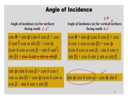
So, the next one is angle of incidence for surfaces facing south, as we already said azimuth angle is 0 degree. And if we substitute that, then this particular term would go because sine 0 is there. Other than that here cos gamma, so this becomes 1. And then, here also cos gamma, so this becomes 1. So, sine phi sine delta cos beta, and then cos delta cos gamma, that is 1 anyway we can override there is no harm in that.
