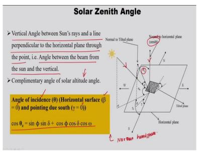
And then, solar zenith angle, vertical angle between sun's rays and a line perpendicular to the horizontal plane through the point. So, this is that line which is normal to the horizontal plane. And then this is the line of sun's rays. So, the angle made between these two lines is called zenith angle, or it is called us angle between the beam from the sun, and the vertical. Vertical is nothing but zenith.
