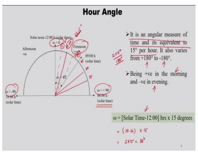
The next one is hour angle. It is an angular measure of time and is equivalent to 15 degree per hour. So, we have 12 hours from sunrise to sunset. So, 12 hour into 15 degree around 180, so sunrise to sunset again sunset to sunrise. So, it varies from plus 180 to minus 180, so being positive in the morning and negative in the evening. So, for example, here, the 6 hours in the morning. So, this is measured as 90 degree and solar time solar noon, which is 12 hours.
