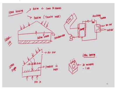
So, here too, we have two method one is active where we use fans and blowers. And the second one is passive method by natural circulation, the famous concept of Trombe wall (()) (11:41) from passive method. So, here to, just to review about, we have a flat plate collector, from which your hot water comes, goes to storage. From here it is taken using pump and goes to FPC, and from here you can take it out.
