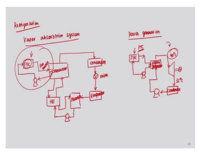
If you want to have higher temperature, then one may need to go to concentrating type collectors which is nothing but parabolic trough collector PTC. So, it depends purely on the application side. So, at what temperature you would be required. For example in the generator you would be producing the refrigerant vapors.
