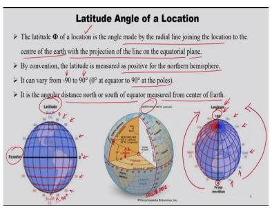
The first one is latitude angle of a location, the latitude angle of your location is the angle made by the radial line joining location to the center of the earth. So, that is this particular line. So, this is nothing but our location where we suppose to calculate the latitude. So, this is center of earth, so this is the line joining these two points with the projection of the line on the equatorial plane. So, that is this particular line.
