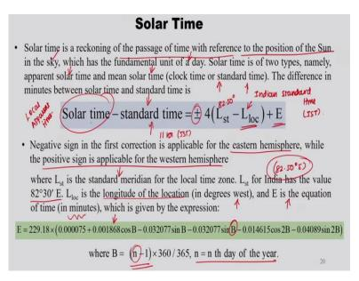
The next one is solar time. Now, solar time is the reckoning of the passage of time with reference to the position of the sun in the sky which has the fundamental unit of the day. So, there are two types of solar time, with which we can measure. So, one is apparent solar time so this we call it as a local apparent time. The second one is mean solar time, so which is nothing but a clock time or standard time.
