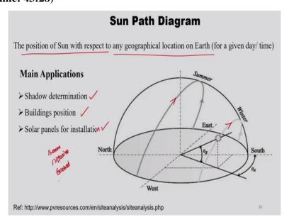
So, the next one is sun path diagram so this is nothing but the position of the sun with respect to any geographical location on the earth for a given day time. So, this is particular sun path during summer time. So, this is during winter time how the sun travels from sunrise to sunset
