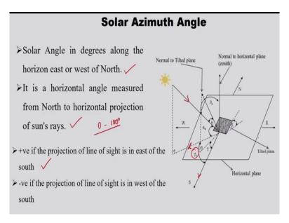
The next one is solar azimuth angle. Solar azimuth angle is nothing but gamma s, so solar angle in degrees along the horizon east or west of north. It is a horizontal angle measured from north to the horizontal projection of sun's rays. So, the horizontal projection of sun's rays, this particular line and this is the line due south, due south line.
