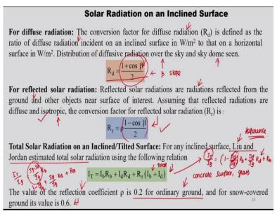
And, for diffusive radiation, so this is again, diffusive radiation is defined as the diffusive radiation incident on an inclined surface, which is again in watt per meter square to that of the horizontal surface again watt per meter square. So, usually, this is based on distribution of diffusive radiation over the sky, and sky dome seen from the tilted surface. So, this is defined as R d is 1 plus cos beta upon 2.
