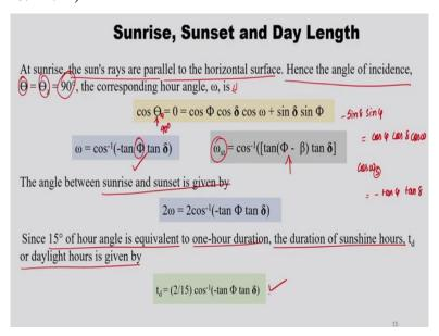
Then sunrise, sunset and day length. How to calculate them? So, at sunrise, the sun's rays are parallel to the horizontal surface. So, angle of incidence would be theta, theta z which is
