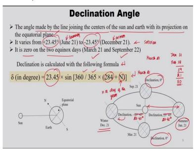
The second one is declination angle. So, this angle is nothing but, made by the line joining centers of the earth and sun with its projection on the equatorial plane. So, it varies from plus 23.45 degree on June 21 to minus 23.45 degree on December 21. So, these both we call it as a solstice, solstices. So, this is winter solstice. So, this is summer solstice. And this particular delta declination angle is 0 on 2 equinox days, one is on March 21 and another is on September 22.
