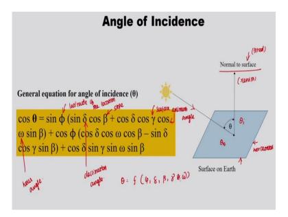
Next one is angle of incidence. So, this is suns ray or the line of sight, so this is considered as horizontal surface. So, this is normal to the surface. So, this angle made between the line of sight and the normal to the surface is called theta. So, if this surface is horizontal one, so then normal to that, we call it as a zenith. An angle made this zenith angle or normal angle of incidences, so this, if the surface is tilted one.
