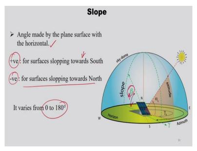
And then the next is slope, angle made by the plane surface with the horizontal. So, it varies from 0 to 180 degree. If the surface is sloping towards south, it is calculated as positive 0 to, 180, and for surfaces sloping towards north, so it is negative. So, in that way it is calculated as 0 to 180 with the negative sign. So, this is here, mentioned us beta. So, this is horizontal, this is inclined surface. This particular angle is slope.
