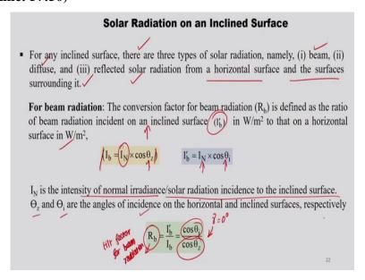
For beam radiation, we calculate the R b, which is nothing but the tilt factor or conversion factor. Tilt factor for beam radiation. So, the here R b is defined as the ratio of beam radiation incident on an inclined surface which is nothing but I b dash in watt per meter square to that on a horizontal surface, which is also in watt per meter square. So, I b is for horizontal surface, which is nothing but I N that is the beam flux into cos theta z.
