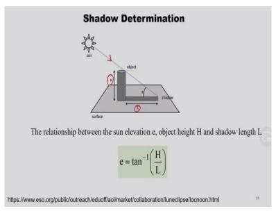
And then shadow determination. So, this is most of you know already, so this is nothing but an object, and its height is H and its projection is L, and this is nothing but elevation, suns elevation. So, in that way, tan e is nothing but H upon L, so e is tan inverse of H upon L. So, this way, the shadow determination can be done.
