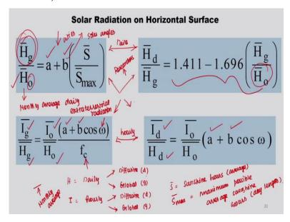
And then solar radiation on horizontal surface, so here it is mostly with all correlations. So, here this H refers to daily diffusive or global radiation, I refers to hourly diffusive and global radiation. So, this is d. So, this is g. This is d. This is g. So, this bar refers to monthly average. And then here if you see there are S bar which is nothing but, sunshine hours for a day. And S max is nothing but, maximum possible.
