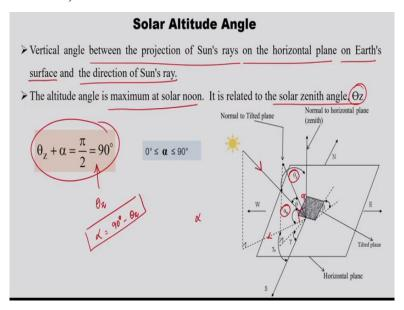
And then solar altitude angle, which is defined as alpha, vertical angle between the projection of sun's rays on the horizontal plane on earth's surface, and the direction of the sun's ray. So, this is sun's ray and its projection of sun's rays on the horizontal plane as this. So, this particular angle made between these two lines is called solar altitude angle. So, this is maximum at the solar noon, and it is related to the solar zenith angle theta z.
