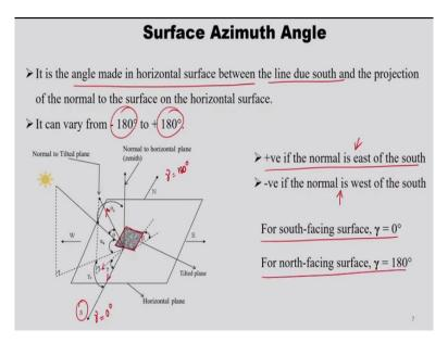
The next one is surface azimuth angle. So, it is the angle made in horizontal surface between the line due south. So, this is the line due south, so this particular line, and the projection of the normal to the surface on the horizontal plane. So, for example, so this is the tilted plane, as we have seen already, so the normal to the tilted plane is this particular line. So, it is projection of the normal to the horizontal surface.
