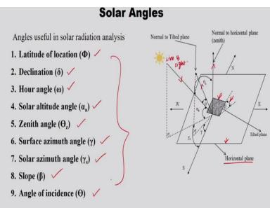
The solar angles, there are 9 various angles we suppose to be comfortable with to analyze solar radiation parameters which are latitude of the location, declination angle, hour angle, solar altitude angle, zenith angle, surface azimuth angle, solar azimuth angle, slope, and then angle of incidence. So, this diagram says about the horizontal plane, which is this, and then the tilted plane is the way we tilt the plane to absorb solar radiation maximum.
