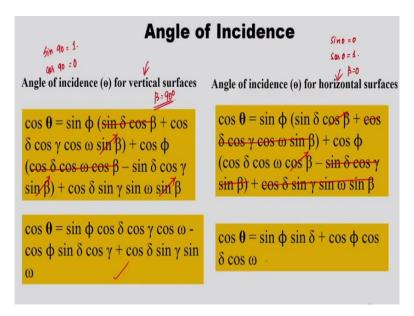
So, from the basic equation general equation we can derive it for different surfaces. So, vertical surfaces, beta equal to 90 degree, which is nothing but slope. So, we have this convention, sine 90 is 1, and cos 90 is 0. So, if we see the first term, so this will go cos 90 0. And then here, sine beta this becomes 1. And then so we have cos 90, so this particular term will go. And then we have sine beta, so this become 1.
