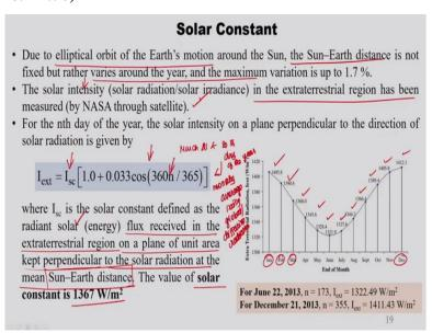
And then the solar constant, actually solar constant is defined as the radiant solar energy flux
