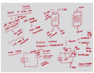
Liquid materials normally we use for solar water collector. And sensible heat can be done for wide range of temperatures. But in phase change materials you need to be careful about the
