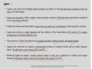
So now the last component of the cell wall is lignin. So now lignin is one of the most abundant organic polymers on Earth, it is the third important constituent of the cell wall of woody biomass. Lignin are amorphous, highly complex, mainly aromatic polymers of phenylpropane units that are considered to be decorating substances, unlike cellulose and hemicellulose, the lignin does not contain any carbohydrate in their polymeric structure.
