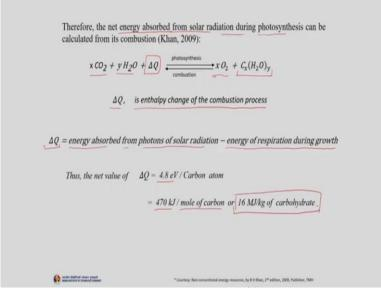
The net energy absorbed from solar radiation during photosynthesis can be calculated from its combustion process. Why we are saying here it is combustion, because the carbohydrate molecule is reacting with oxygen and then producing CO 2 water and energy. Although we mentioned here the combustion which is a respiration process, but conventionally if you try to see the combustion process which carries out at very high temperatures, say around like 400 degrees C.
