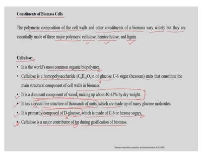
So, the next point is constituents of the biomass cells. The polymeric composition of cell walls and other constituents of biomass vary widely, but they are essentially made up of 3 major polymers and that is what I mentioned in the previous slide. The cell walls are majorly made up of 3 polymers these are cellulose, hemicellulose and lignin. First of all, let us see what is meant by the cellulose?
