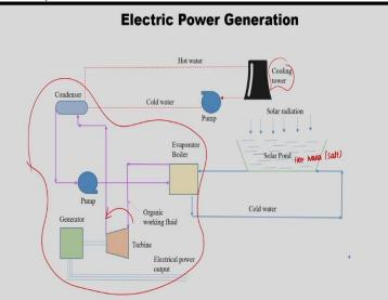
Here we are seeing the electric power generation. In the electric power generation unit this is the one so from the boiler it goes to turbine in the turbine. So, it should be reverse from the boiler it will go to turbine, from the turbine it goes to condenser the working fluid then after that it is pumped back to the evaporator right from the turbine if it is connected to the generator it produces the electricity for the year operator you might require the hot water.
