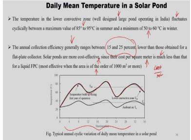
So, this is nothing but daily mean temperature in the solar pond, so if you see this is for almost 3 years it is taken. So here if you see it is almost a cyclic in nature with 1 or 2, months difference. The temperature in the lower convective zone if it is well designed well insulated and a large part operating in India. India in the sense like medium solar radiation happens throughout the year if
