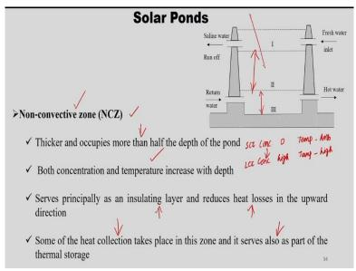
The non-convective zone here it is thicker and occupies more than half of the depth of the pond. So, here both concentration and temperature vary or increases with depth because we set concentration is 0 at the top layer to provide the conviction and concentration is high at the bottom layer this is top which is nothing but surface convective zone SCZ. So, this is last one is lower convective zone.
