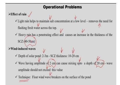
The operational problems the effect of rain when light rain helps to maintain the salt concentration at lower level because it dilutes the surface water and removes the need for flashing freshwater across the top. As I said earlier, there may be concentration change due to stratification, thermal stratification. So, in that case we then under flush the freshwater to dilute the concentration at the top if the light rain happens this helps in that way naturally if heavy rain penetrating.
