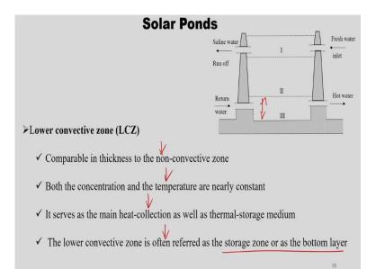
Lower convective zone is nothing but this zone comparable in thickness to the non-convective zone and both the concentration and temperature are nearly constant and high as well itself stuff mainly heat collection as well as the storage or thermal storage medium. The lower convection convective zone is often referred as the storage zone or the bottom layer of the solar pond.
