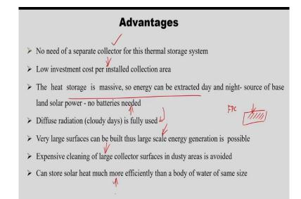
Advantages wise no need of separate collector for thermal storage, it can do both the operation collection as well as storage low investment cost per installed collection area the heat storage is massive. So, energy can be extracted day and night source of base land solar power, no batteries are needed for storage diffusive radiation is also fully used because it is an open area very large surfaces can be built thus large-scale energy generation is possible.
