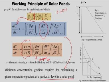
So, in this case, if you write rho as a function of C and T concentration and temperature or how do you write this is dou dou C of rho at a constant T into d dx of C + dou dou T of rho at constant concentration which is multiplied by d dx of T which is greater than 0. So, from this if you calculate dC dx which is greater than of minus of dou dou T rho at C into d dx of T upon dou dou C of rho at constant temperature.
