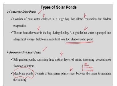
So, types of solar pond convective solar and non-convective solar pond. Convective solar pond we do not make any special effort here the it consists of pure water enclosed in a large back that allows the convection but hinders the evaporation the sun heats the water in the back during a day at night hot water is pumped into large heat storage tanks to minimize the heat loss. So, this example is shallow solar pond so, here we did not stop the convection by adding salt water or anything.
