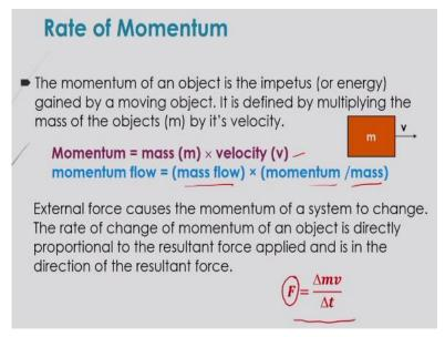
Next, let us consider that momentum rate. The momentum of an object actually is the impetus or you can say the energy that is gained by a moving object. It is defined by multiplying the mass of the objects by its velocity. So, momentum will be defined as mass into velocity and momentum flow would be basically that mass flow into momentum by mass. Now, external force generally causes this momentum of a system to change.
