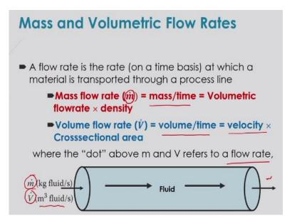
Now, coming to that point of that flow rates, first that mass and volumetric flow rates which is to be important aspects are you are going to analyze any process of that chemical engineering or biochemical engineering in a particular process unit and there you will see some streams will be coming to the process unit at a particular flow rate and also the systems will give you that output and that output will be coming out as a particular stream with certain flow rate.
