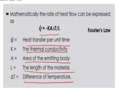
So, this mathematical expression given by Fourier. So, that is why it is called Fourier's law. So, mathematically the rate of heat flow by conduction can be expressed as Q dot will be is equal to minus KA delta T by L where Q dot is heat transfer per unit time, K the thermal
