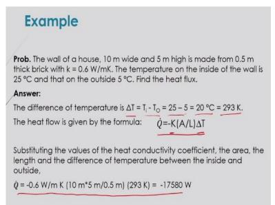
Let us do you an example based on this. Suppose, the wall of a house that is 10 meter wide and 5 meter high that is made from 0.5 meter thick brick with thermal conductivity that is K that will be is equal to 0.6 watt per meter K and the temperature on the inside of the wall is 25 degrees Celsius and that on the outside is 5 degree Celsius. Now in this case, find the heat flux. Now, the difference of the temperature is delta T, so this T of course always will be in terms of unit Kelvin.
