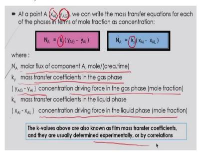
Now at a point suppose A where the concentration maybe mole in terms of mole fraction for the liquid as well as gas, generally for liquid it is expressed as XAX and for gas it is YY, so XAL and XAG. Suppose there is a mole faction in the two phases in the liquid and gas respectively, then we can write the mass transfer equations for each of the phases in terms of mole fraction as concentration like this NA is equal to Ky into YAG minus YAi and NA will be is equal to Kx into XAi minus XAL.
