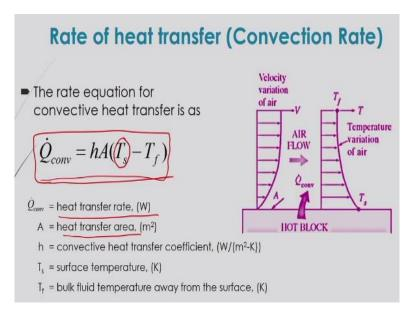
Now, the same way you can say that that rate of convective heat transfer depends on the temperature difference between two locations. Here in this case, one location will be in the hot surface and other will be in the fluid by which that heat will be transferred by convective mode and this law is called the Newton's law of heating or cooling and according to that, the rate of convective heat transfer can be expressed as Q dot convective that will be is equal to hA into Ts minus Tf.
