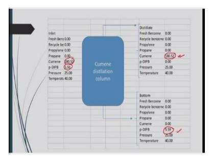
Where input of the Cumene distillation column will be the same that is Cumene and you know byproduct. And it is being separated and as a distillate on the you know that Cumene productive becoming. And at the bottom on that only you know p-DIPB will be coming. So, this final Cumene distillation column we are getting separation of this you know Cumene and byproduct.
