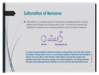
And sulphonation of benzene basically is reacted based on this, this is reversible reaction. That produces benzene sulphonic acid by adding sulfur trioxide and fuming sulfuric acid. The reaction is reversed by adding hot aqueous acids to benzene sulphonic acid to produce benzene. Now to produce a benzene sulphonic acid from benzene fuming sulfuric acid and sulfur trioxide are added, fuming sulfuric acid is a concentrated solution of dissolved sulfur dioxide in sulfuric acid.
