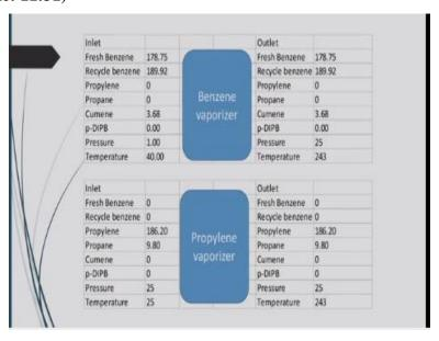
Similarly for benzene vaporizer propylene vaporizer, what are the different inlet and outlet compositions are given. So according to that calculation, you will see that at the same has already been discussed in details of that calculation given in the previous lecture. So, here just summarized that calculation, these are the things for mixer and furnace also it is given.
