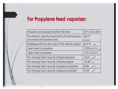
For propylene feed vaporizer similarly you can calculate what should be the you know heat required for those. Now in this case propylene and you know propane fed from the tank is at 25 degrees Celsius at 25 you know atmospheric pressure. The stream is vaporized and heat to the temperature and mixed with benzene feed is at you know 243 degrees Celsius.
