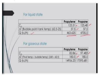
And for liquid state, the C p value for propylene is given 123.51 whereas it is for propane is 125.48. So, delta T is basically that bubble point temperature and tank temperature of this propylene propane mixer and it is basically 62.5 - 25, then it is coming 37.5. And then what will be the heat required for that liquid state to raise this the temperature from 25 degrees Celsius to you know bubble point temperature of 62.5 degree Celsius.
