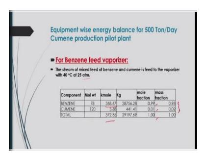
In that case if we do the energy balance equipment wise for this process, we can say that for benzene feed vaporizer, if we consider first that because benzene will be send to the reactor after mixing with the you know propylene. And before that, those propylene and benzene will be you know vaporized to a certain temperature. Now these are to be vaporize to you know at 40 degrees Celsius.
