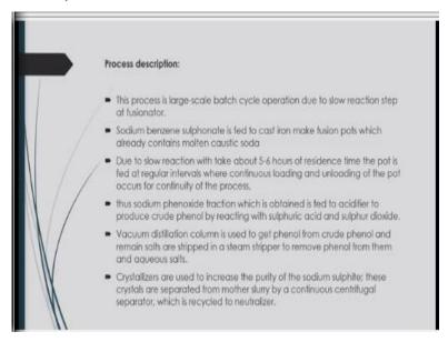
Now, process description that we have already described that this is the you know largest scale batch cycle operation due to slow reaction step at fusionator. Sodium Benzene sulphonate is fed to cast iron make fusion pots or who is already contains molten caustic soda there. Due to slow reaction with take about you know that 5 to 6 hours of residence time, the pot is fed at regular intervals where continuous loading and unloading of the pot occurs for continuation of the process.
