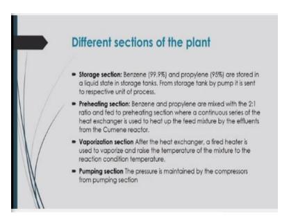
And different sections are here storage section, preheating section, vaporization section, pumping section and also reactor section there. And in the reactor section, the pressure up to 25 atmospheric pressure will be considered and the reaction will be done at 350 degree Celsius.
