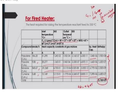
So, for that what would be the amount of heat required for raising this temperature of this reactant mixture of propylene and benzene to 350 degree Celsius. Now for that we have to calculate what from the enthalpy for that individual components of that mixture. So compound basically before going to that fire heater is you know that propylene, propane, benzene, Cumene all those things.
