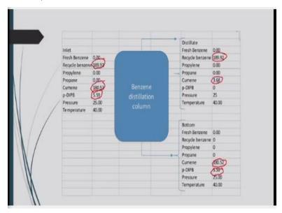
And then it will be going to that benzene distillation column where you will see that only recycle benzene and Cumene and a small amount of p-DIPB will be separated. Whereas in the top product of this benzene and benzene distillation column it will be only recycle the benzene and small amount of Cumene. And the bottom product the main product that is Cumene will be coming out along with that you know byproduct there.
