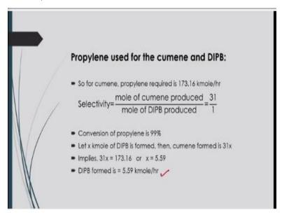
And also the selectivity of that reactions are based on which we have calculated the you know what will be the amount of byproduct will be produced that is given here. It is around 5.59 kilomole per hour. As per you know assume data for production of Cumene.
