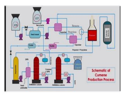
Still you know go through again that process for you know describing the energy balance equation here in this lecture. So basically that Cumene is produced from the benzene and propylene at a certain you know temperature and pressure in a particular reactor. And then the product is being separated by you know different separator units like flash drum distillation column.
