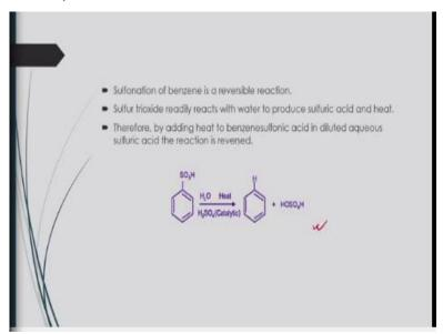
Now sulfonation of benzene is a reversible reaction that we know that sulfur trioxide readily reacts with water to produce sulfuric acid and heat. Therefore by adding heat to benzene sulphonic acid in diluted aqua sulfuric acid the reaction will be you know reversed, so this is your reverse reaction.
