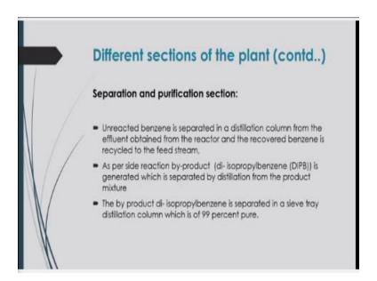
Now, separation and purification section that involves that you know flash drum benzene distillation column and Cumene distillation column.
