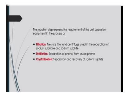
That reaction step explains the requirement of the unit operation equipment in the process are here filtration and distillation and crystallization.
