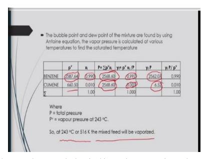
Now, based on these you have to calculate in this you know vaporizer, what would be the vapor pressure of those you know components in this you know feed vessel of benzene. Now, the bubble point and the dew point of the mixer are found by using Antoine's equation. That means, how to you know get that you know bubble point from that Antoine's equation.
