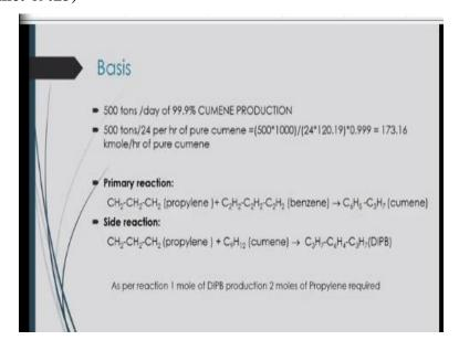
So, in this case based on this data assumptions we have done, that material balance by considering that reaction stoichiometry.
