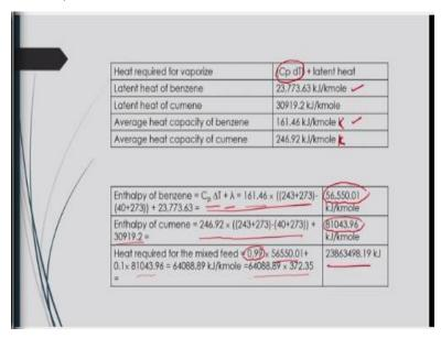
Now heat required for vaporized this basically one should be that due to the raise in temperature and also due to the feed change of that you know feed mixer. Now for that for feed change of course you have to consider that latent heat and for temperature difference that heat to be calculated based on that sensible heat like this is C p into D t. So, heat required for the vaporize you know that it will be summation of that sensible heat and latent heat.
