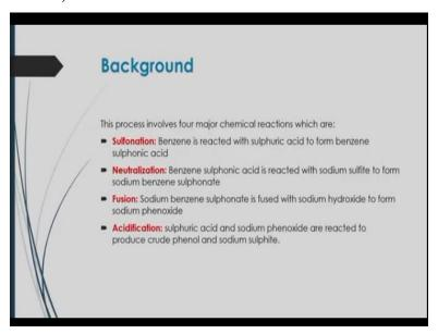
Now in this case the process involves 4 major chemical reactions, whose as sulphonation where benzene is reacted with sulfuric acid to form benzene sulphonic acid. Neutralization where benzene sulphonic acid is reacted to sodium sulfite to form sodium benzene sulphonate. And in the fusion reaction the sodium benzene sulphonate is fused with sodium hydroxide to form sodium phenoxide.
