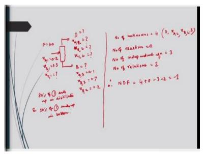
Let us consider another examples as per this diagram here like this in this case like one separation process by distillation here. Here again distillate here x A 2 is unknown to you x B 2 is unknown to you, x C 2 is unknown to you whereas here in the bottom it is also unknown to you. And then what is that x A 3 = 0.1, x B 3 that will be equal to 0.7 and x B C that will be equals to 0.2.
