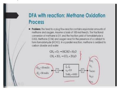
Like here if we consider another examples with reaction what will be the degrees of freedom like methane oxidation process. In this case the feed to a plug flow reactor contains equi molar amounts of methane and oxygen. Assume a basis of 100 moles feeds per second, the fractional conversion of methane is 0.1 and the fractional yield of formaldehyde is 0.855, methane and oxygen react in the presence of a catalyst form this formaldehyde.
