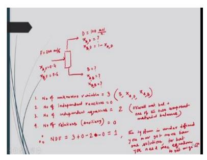
Let us do another examples, suppose a problem let us have this problem here again one distillation column. Where in this distillation column the feed will be entering at a rate of 200 mole per hour where composition at this feed as x A F that will be close to 0.4. And x B component B in this feed is equal to 0.6 and bottom product here B is unknown to you x A at this B it is also unknown to you, x B B it is unknown to you.
