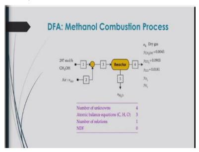
Another example, methanol combustion process how to analyze the degrees of freedom. Here also you can get this degrees of freedom as 0 with this known and unknown variables in the flowchart.
