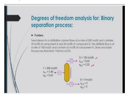
Now let us have an examples to calculate the degrees of freedom for binary separation process. Now, let us have this problem like if you have the feed stream to a distillation column that flows at rate of 200 mole per hour and contains 40 mole percent of component A and 60 mole percent of component B. The distillate flow is at a rate of 400 mole per hour and contains 65 mole percent of component A and remaining is 35% of component B.
