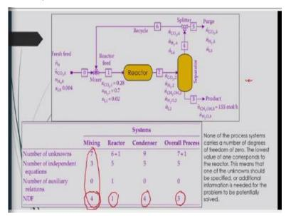
Here this flowchart is given and in different you know inlet and outlet streams for different you know units there all knowns and unknowns variables are specified. And accordingly what will be the number of unknowns, number of independent equations and number of auxiliary relations are given. And then according to what should be the number of degrees of freedom that is analyzed based on individual equipment, it is shown in the slides.
