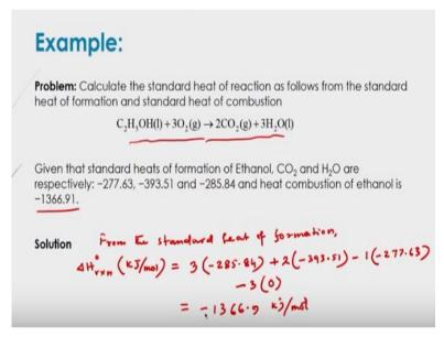
In this case ethanol will be you know reacting with oxygen which will give you that carbon dioxide and water after complete combustion. Now in this case the heat of formation of ethanol, carbon dioxide and water are respectively given as -277.63, -393.51 and -285.84. And heat of combustion of ethanol is given as -1366.91.
