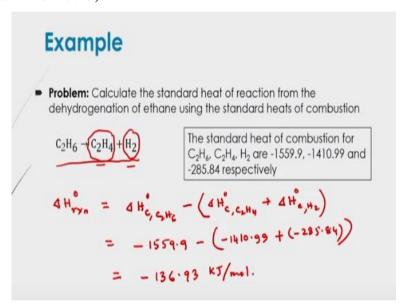
Let us do another example. In this case, calculate the standard heat of reaction from the you know dehydrogenation of ethane using the standard heat of combustion. This reaction is given to you here in this case dehydrogenation of ethane giving you that here ethane and hydrogen.
