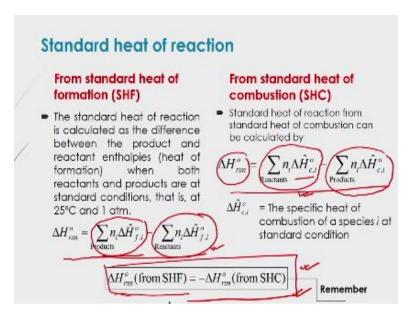
As we know that standard heat of reaction that is actually obtained based on that heat of you know formation of that constituents, which are taking part in the particular reactions.
