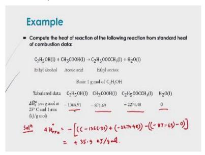
Like you have to calculate the heat of reaction of the following reaction from the standard heat of combustion data. Here ethyl alcohol will be you know, reacting with acetic acid which will give you that ethyl acetate and water. In this case one gram mole of ethanol is considered.
