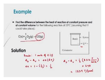
Now let us do an example for such cases. Here in this case, you have to find out what should be the you know the difference between the heat of reaction at constant pressure and constant volume for the following reaction at 25 degree Celsius assuming that it could take place here as per reactions here.
