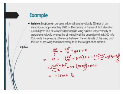
Like this let us do an example here. Suppose an aero plane is moving at a velocity 250 meter per second at an elevation of approximately 8000 meters Now, the density of the air at that elevation is considered as 0.4 kg per meter cube the air velocity at under side wing here of that aero plane has the same velocity of the aeroplane velocity whereas, the air velocity at the underside wing is 300 meter per second.
