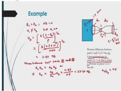
Let us do another examples here see 1 figure is given in the slides this case water is flowing from a tank to a you know that converging diverging, you know 5 this called you know venturing 5 and you will see that when you are this venturing pipe is let us to that tank at this location. The diameter of this part of this density is here at this study one for us at this you know converting section of this venturing at point 2 its diameter is d2.
