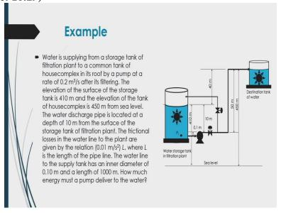
Now, let us do an example with this you know, mechanical energy balance equation. So, this is basically mechanical energy balance equation. So, in this case, if we consider that the water is supplying from a storage tank or filtering plant of a you know common tank of house complex in its roof by a pump at a rate of 0.2 meter cube per second after this filtering and the elevation of the surface of the storage tank is a 410 meter.
