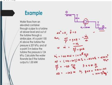
Now, let us do another example, like water flows from any elevated container through a pipe to a turbine at a level at a lower level and out of the turbine to a similar pipe here has given in the picture in the slide and you will see that at a point 100 meters above from this you know turbine the pressure is 207 kilo Pascal and at a point 3 meter below the turbine the pressure is 124 kilo Pascal.
