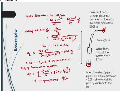
Let us do another example of this Bernoulli's equation like here one you know that nozzle is shown in the slide here and water is flowing through a nozzle before coming to that or before playing to that nozzle here, this is 1 nozzle at this point 2 and before flowing through that nozzle, the fluid is coming from a pipe at point 1. Now, the pipe diameter at point 1 it is given a certain
