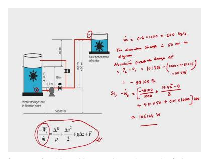
Now, in this case how to solve this problem, we know that mechanical energy balance by this equation here we have already described. So, based on this mechanical energy balance you have to calculate what should be the you know energy required to you know supply that water from that you know storage tank to the you know destination tank here. So, this -W is by m dot that will be equal to delta p by rho + delta U squared by 2 + g delta z + F.
