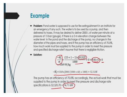
Let us do another example here like suppose, a pond water is supposed to use for fire extinguishment in an you know Institute for an emergency if any sauce case, that is the water is to be used by a pump and then delivered to hoses it may be designed to deliver 2000 liter of water per minute at a pressure of 15 bar gauge if there is a 5 meter elevation change between the water level in the pond and the discharge of the pump that case no change in the diameter of the pipes and hoses.
