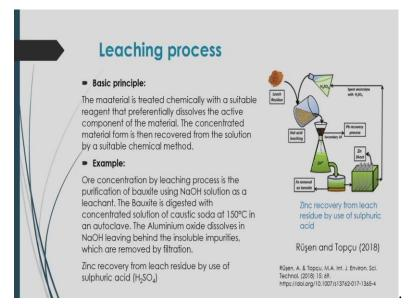
Leaching process like in this case the martial is treated chemically with a suitable reagent that preferentially dissolves the active component of the material. The concentrated material from is then recovered from the solution by a suitable chemical method. In this case on example say that,
