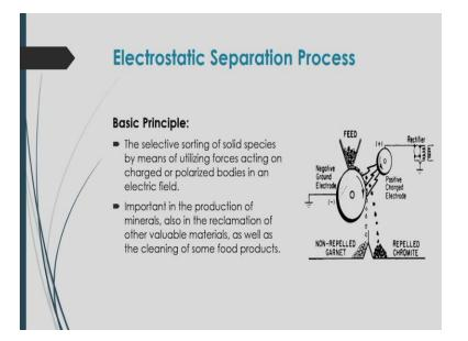
Electrostatic separation process also regarded as chemical engineering process where selective sorting of solid species by means of utilizing forces acting on charged or you can say that polarized bodies in an electric field. So this case it is important in the production of minerals also the reclamation of other valuable materials, as well as the cleaning of some food products there.
