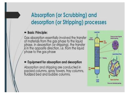
Absorption and desorption process the gas absorption is one of the important separation process in chemical engineering, where gas absorption essentially involved the transfer of materials from the gas peace to the liquid phase. And oppositely you can see that, desorption of course there. It is also sometimes called stripping.
