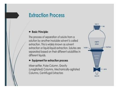
Extraction process in this case the process of separation of solute is being taken place from a solution by another in soluble solvent and this is widely known as solvent extraction. Or liquid-liquid extraction, salutes are separated based on their different solubilities in different liquids. Mixer-settler, Pulse column, Gravity columns, Mechanically-agitated column, Centrifugal extractors these are the some common equipment, that are being used for this extraction process.
