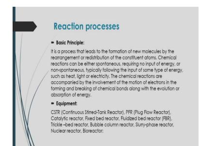
Similarly, reaction process it is process that leads to the formation of new molecules by rearrangement or redistribution of the constituent atoms. That chemical reaction can be either spontaneous, requiring no input of energy, or non-spontaneous, typically following the input of some type of energy such as heat, light or electricity. So in this case after reactions you will see different types of products output will be coming at a certain condition pressure and temperature.
