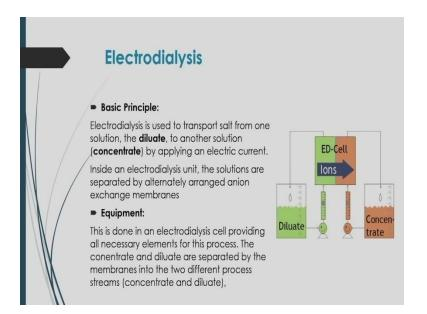
Electro dialysis also important chemical engineering process, where transportation of salt from one solution is required in that case, it is called dilate , To another solution by applying an electric current and this is done electro dialysis cell that providing all necessary elements of the process.
