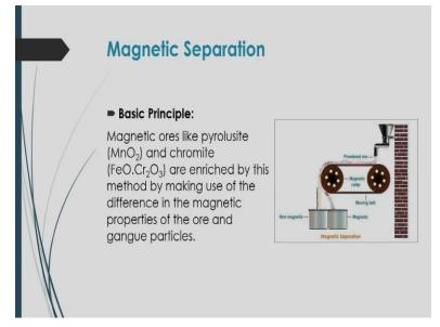
Magnetic separation is also one mechanical operation there. Magnetic ores like pyrolusite like manganese oxide and cromite are enriched by this method by this method making use of the difference in the magnetic properties of the ore and gangue particles.
