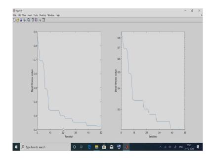
So, we get these two plots. So, as we can see this is the first position, wherein the y axis is not in the logs case; whereas in the second plot, the y axis is in the log scale. So, here we can see that, the objective function value or the fitness function value has been continuously decreasing, right and it is a monotonic convergence because we are plotting the f of g best, right. So, this helps in visualization of the results as to what is happening as the iteration progresses so.
