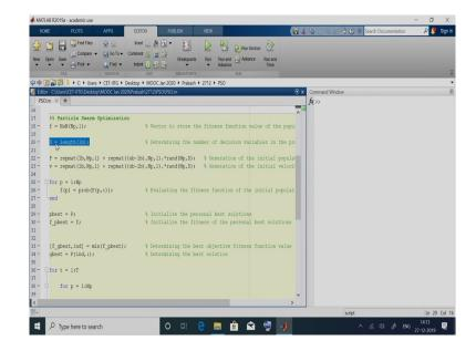
And then we also require these settings to be given by the user. So, number of particles here we have taken it as 10 particles for T is equal to 50 indicates the number of iterations we want to perform, w is the inertia weight which we have initially set to 0.8, c 1 and c 2 are the acceleration coefficients with respect to the social and cognitive part, right.
