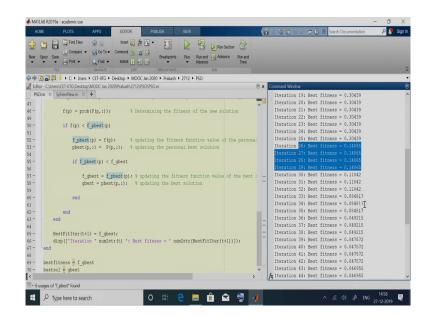
So, now, if we execute this; this displays the best fitness with respect to every iteration. So, we can see that the value 0.39194 is constant for three iterations; that means that for three iteration, there was no update in g best, right.
