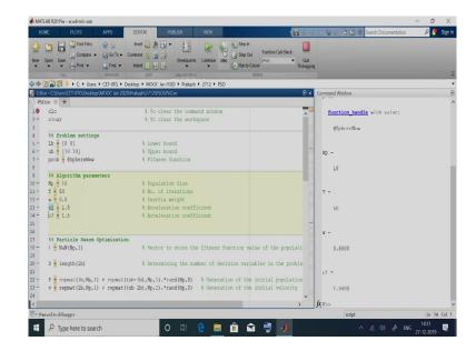
And then we are defining the population size, the number of iterations, the inertia weight, the acceleration coefficient c 1, the acceleration coefficient c 2, right.
