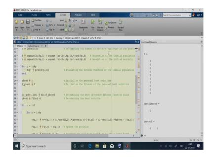
At the end of the entire procedure, since we have not given a semicolon in at the end of line 65 and 66; it is displaying the best fitness and the best solution. So, at the end of all the iterations for all the members, the best solution that we get is 0 comma 0 for the sphere function; and the best fitness function value corresponding to this 0 comma 0 is 0, right.
