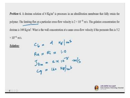
So a very small problem we will see then we will wind up todays lecture. A dextran solution of 4 kilogram per meter cube is processes, in a ultrafiltration membrane that fully return the polymer. The limiting flux that is J limiting, at a particular cross flow velocity is given to be 2 into 10 power of - 5 meter per second. The gelation concentration for the dextran is 160 kilo per meter cube.
