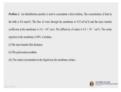
So let us see another example, I am reading out that actually the problem statement, so an ultrafiltration module is used to concentrate a feed solution, the concentration of heat in the bulk is 0.6 mass %. The flux of water through the membrane is 0.53 meter cube per meter square hour and mass transfer coefficient at the membrane is 3.6 into 10 power of -5 centimeter per second.
