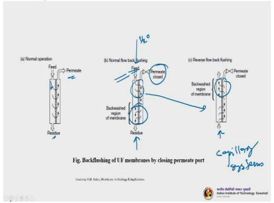
And let us see the back flushing we have never discussed black flushing in detail, we will just try to understand how back flushing actually happens. So, actually the cleaning process mechanism is that first once the process is over, so, you take out the membrane system. And try to use the fresh water from permeate side of the membrane and depending upon what type of membrane actually you are having and then try to clean it.
