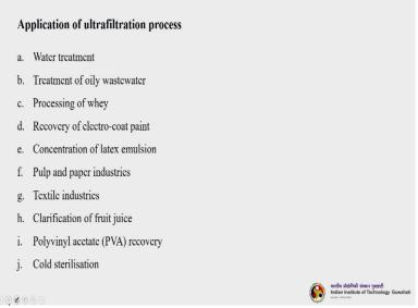
Now, let us understand and discuss different types of ultrafiltration processes applications basically. So, water treatment, treatment of oily waste water, processing of whey, recovery of electro coat paint, concentration of latex emulsion, pulp and paper industries application, textile, clarification of fruit juice, PVA recovery in the this one cloth manufacturing industries and cold sterilisation.
