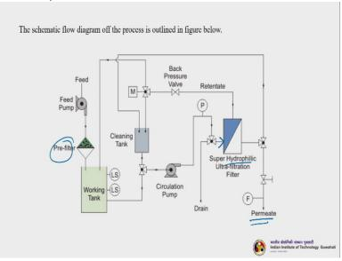
So, just closely have a look at this particular figure, a schematic diagram which is used to treat the wastewater. So, your feed is coming here. So, there is some sort of pre-filters on here as we have discussed just why pre-filter is required, we put it is being fed to the ultrafiltration
