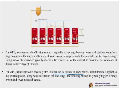
So this is a WPC system so, a continuous ultrafiltration system is typically set up stage by stage so it is not a single ultrafiltration membrane will do the job. So they are stage by stage or in series, along with the diafiltration in later stage to increase the removal efficiency of so in between a few ultrafiltration test, which is removed during the WPC, there are some repetition membranes also installed.
