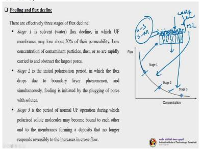
So, let us understand the different stages of fouling. So, usually stages in ultrafiltration fouling has been described by 3 stages stage 1, stage 2 and stage 3. So, in stage 1 the solvent or water flux decline is happening actually. So, I here from here to here. So, the membrane
