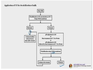
So, this is a schematic diagram of how that how decalcification of milk is achieved. So, skim milk is passed through ultrafiltration to increase the concentration almost to up to 4X at 10 degrees centigrade using a 10 kilo delta membrane. Then whatever the retentate is coming the retentate is actually calcium fortified, it will reduced with reduced lactose and skim milk retentate.
