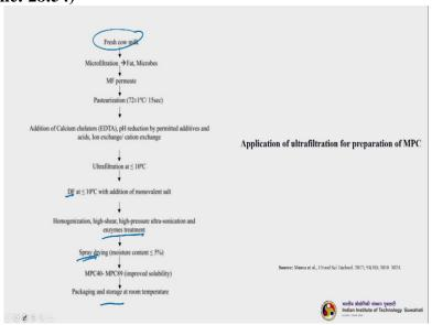
So, this is flowchart actually, this tells us about how ultrafiltration is being used for preparation of the milk protein concentrate. So, you take your fresh cow milk, so, it goes to the microfiltration test and as you have discussed, it will remove the fat and as well as other
