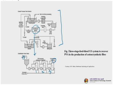
So, this scheme you can see. So this is the complete process. So, in which 3 stage feed-and-bleed ultrafiltration systems was used to recover PVA in the production of cotton and synthetic fibre. So here the ultrafiltration system is being shown here. It is a 3 stage feed-and-bleed system. So that you can see that in the feed the PVA percentage is only 1 percent. So now using a 3 stage, stage 1, stage 2, stage 3, we are enriching up to 8 %. So this is how PVA is being enriched and then recover.
