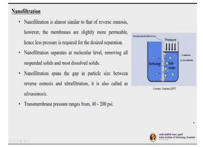
Then we will discuss about nano filtration, so nano filtration is almost similar to that of reverse osmosis, however membranes are slightly more permeable. Since the membranes of nano filtration are little more permeable hence the pressure required for nano filtration is obviously lesser than that of the reverse osmosis and nano filtration separates at molecular level removing all suspended solids.
