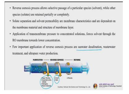
So reverse osmosis process allows selective pressures of a particular species usually the solvent while other species solutes are written or partially or completely. Solute separation and solvent permeability are membrane characteristics and that dependent on the membrane material and structure of the membrane layer. So application of transmembrane pressure to concentrated solutions forces solvent through the RO membrane towards the lower concentration.
