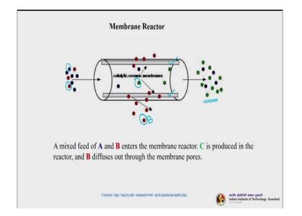
So let us see this figure here you can see there is a mixture of A and B. So this is A and this the red one is B so both are passing or entering through the membrane reactor and inside the membrane reactor catalytic conversion takes place so we can see two ceramic membranes here tubular ceramic membranes here, there can be many more just for our understanding we have seen two I have shown two here.
