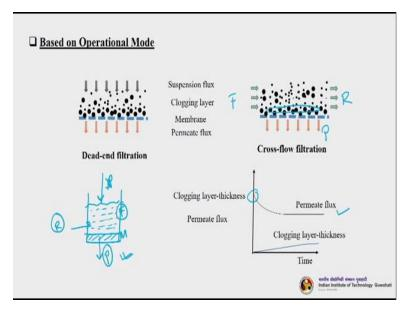
So the next one is based on operational mode so we can have a dead end filtration or we can have a cross-flow filtration. So mostly the membranes works in these two different modes so a deadend filtration I just try to draw something so here you can see so let us say this is a cell in which I have put the membrane here, so this is my membrane okay and then we can fill in my mixture here which containing the solute which I want to separate.
