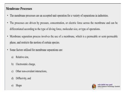
As you know membrane processes are an accepted unit operation, for a variety of separation in most of the industries whether it is a chemical or a veriety of industries. The processes are driven by pressure, concentration or electric force across the membrane. And can be differentiated according to the type of driving force, molecular size or type of operations now membrane separation process involves the use of a membrane.
