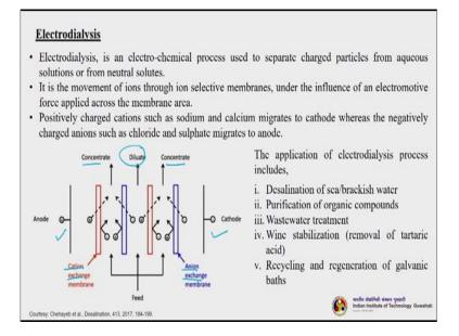
So the next process that will discuss is electro dialysis. So it is a dialysis process which is happening under a electric gradient, so electro dialysis is an electrochemical process used to separate charged particles from aqueous solutions or from neutral solutes. So it is the movement of ions through ion selective membranes under the influence of an electro-motive force applied across the membrane area.
