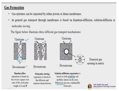
So the next application is gas permeation, so gas permeation or gas separation is one of the most important application of membrane separations and it has lot many industrial applications. So gas mixtures can be separated by either porous or dense membranes we can use both porous and non porous membranes, so in general the transport through membrane is based on knudsen diffusion, solution diffusion or molecular sieving.
