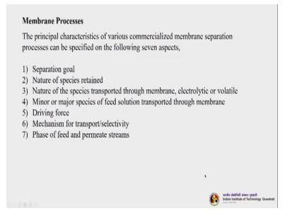
So the principal characteristics of various commercialized membrane separation processes can be specified on the following 7 aspects, these are very important. So these 7 aspects are separation goal, the nature of species retained, nature of the species transported through the membrane either electrolytic or volatile, minor or major species of feed solution transported through membrane, the driving force.
