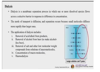
So the next process is dialysis so dialysis is a membrane separation process in which one or more dissolved species flows across a selective barrier in response to a difference in concentration, so please remember that dialysis is a concentration driven membrane separation process. so the mode of transport is usually diffusion, and the separation occurs because small molecules diffuses more rapidly than larger ones.
