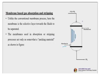
Here the membrane is the Selective barrier or selective layer towards the fluids to be separated, the membrane used in absorption or stripping processes act only as somewhat a picking material as shown in the figure. So you can see this instead of having a peg bed for doing the adsorption we can have membranes okay pegged as a packing material. So we can have the absorbent in here okay an absorbent out here.
