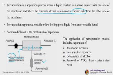
Important application in membrane separation, so it is a process where a liquid mixture is in direct contact with one side of the membrane and where the permeate stream is removed in vapor state. So this is very important the permeate is getting removed in a vapor state, okay from the other side of the membrane. So for the pervaporation the name comes actually from the from what I said just before that it is permeate vaporization.
