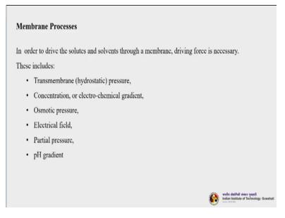
In order to drive the solutes and solvents through a membrane, driving force is necessary. If you remember students last class I told you that in the driving force is of various forms but the true driving force is always the difference in chemical potential. Since we cannot measure chemical potential directly hence we have to express the driving force in a measurable quantity or parameter which can be either transmembrane.
