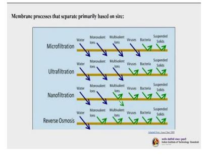
So let us now see if this slide will tell you, how the membranes which basically separate based on the size. So I have given the 4 basic membrane pressure driven membrane processes microfiltration ultrafiltration nanofiltration and reverse osmosis. Please have a close look to the slide you can see that in micro filtration water then different monovalent ions multivalent ions as well as viruses passed through.
