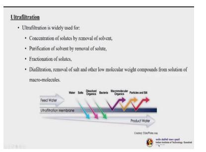
So ultra filtration is widely used for concentration of solutes by removal up by removing the solvent, purification of solvent by removal of solute, fractionation of solutes either binary fraction teritary or even more than that so you can have caskets also. Then diafiltration that is removal of salt and other low molecular weight compounds from solutions of macromolecules you can see this figure okay.
