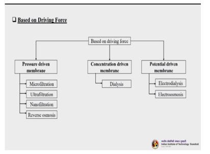
So the next one is based on driving force, so we can have three different types of classification under this particular sub classification. We can a pressure different and driven membrane under which the microfiltration, ultrafiltration and reverse osmosis nano filtration comes then we can have a concentration driven system or a membrane under which dialysis, hemodialysis comes.
