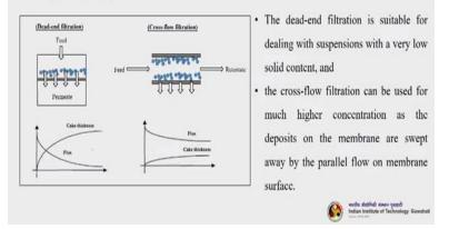
And now we will see one by one different membrane processes and I will try to give a brief introduction about that different types of membrane processes starting with microfiltration. So as you know that microfiltration can be defined as a pressure driven process where it is used to separate micron sized particles from fluid there are two types of micro filtration configuration namely one is dead-end and cross-flow filtration.
