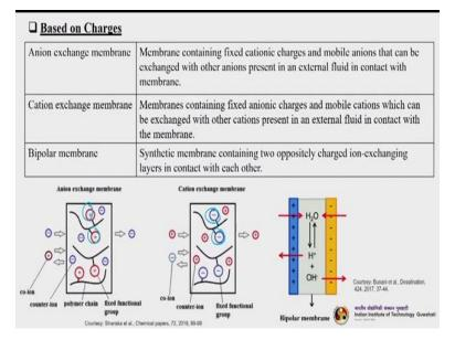
So the next one is based on charges, so we can have three different types of membranes here one is anion exchange membrane, another is cation exchange membrane and then the next one is bipolar membrane now, what is anion exchange membrane? So the membranes containing fixed cationic charges and mobile anions, that anions that can be exchanged with other anions present in an external fluid in contact with membrane.
