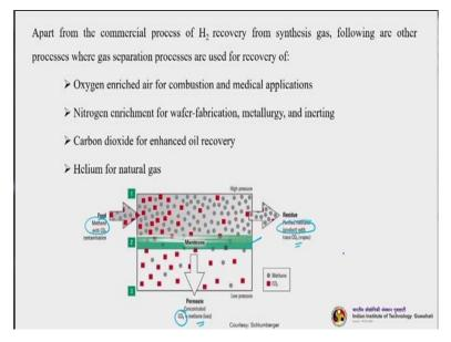
So, the one of the most important commercial application is the hydrogen recovery from synthesis gas okay. And then oxygen enriched they are for combustion and medical applications. Nitrogen enrichment for wafer-fabrication metallurgy and other applications carbon dioxide for enhanced oil recovery, minimal up carbon dioxide then helium for natural gas. Now you can see this particular application in which we are trying to remove carbon dioxide from a mixture of methane and carbon dioxide.
