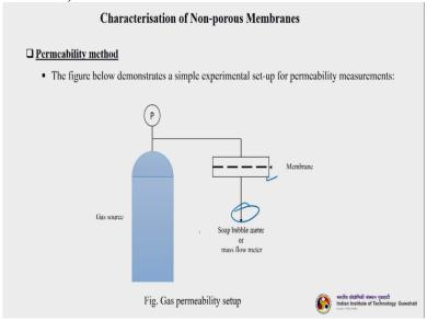
So, the first one is permeability method. So, you remember we discussed permeability of how to calculate water flux and all during our porous membrane characterisation also micro filters and membrane. Now, we will quickly discuss about the permeability method here in non-porous membrane also. Now, here actually instead of water here, we are using gas because since the water flow inside the non-porous membrane will be very difficult.
