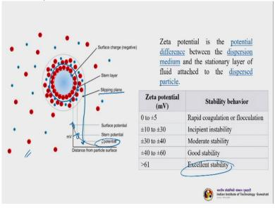
So, now please look at this particular figure, so, here this is also tells you about what is zeta potential. You can see that the surface charges negative this is for example. It is not that all surfaces are negatively charged surfaces can be positively charged also. So then their corresponding ions which will be deposited on immediately on the surfaces this will be the negatively charged just a reverse of this phenomena.
