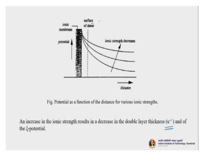
Please look at this particular figure this is what I was just telling the slide before that in increasing the ionic strength result in a decrease in the double layer thickness and this was K inverse which is the divide length and of zeta potential. So, when you are increasing the ionic strength so, the double layer thickness actually is getting decreased. So, the zeta potential will also decrease. This particular figure shows that.
