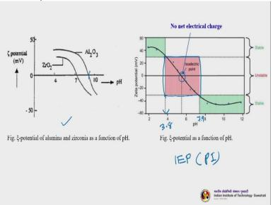
Now have a close look at this particular figures there are 2 distinct figures I am showing here. To understand more about a little better zeta potential it you can see this this particular left hand side figure. So, it is showing zeta potential of alumina and zirconia is a function pH. So alumina zirconia are materials to prepare ceramic membrane in organic membrane. So, what it says this particular figure says this particular figure from here we are finding zeta potential absolutely true.
