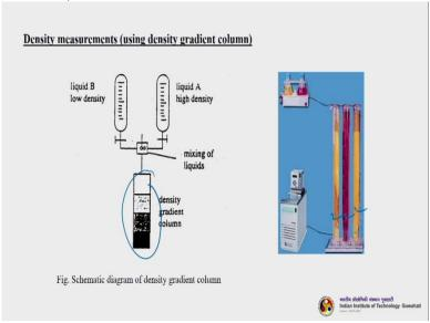
We will see the density gradient column. So, let us look at this particular image. So, this is a schematic representation of the density gradient column what is happening is there are 2 different types of liquids, one having high density and other have been low density and mixed at different proportions in a mixing chamber and they are allowed to flow through my density gradient column.
