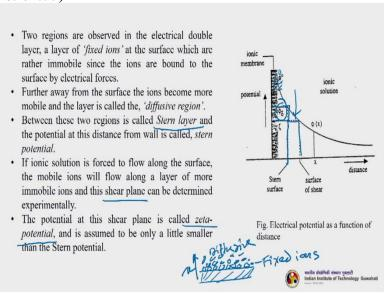
So, let us closely look into this particular figure, which is showing you the electrical potential is a function of distance. Now, 2 regions can be observed in the electrical double layer, a layer of fixed ions at the surface which are rather immobile since ions are bound to the surface by electrical forces. So, basically what is happening this is your membrane actually.
