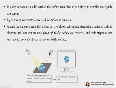
Now, in order to examine a solid surface the surface must be first stimulated to examine the signals that appears. So, to stimulate that we can use either light or x rays in electrons. Different types of electrons per surface stimulation. So, among the various signals that appear as a result of soft surface stimulation particles, such as electron center that are only given above the surface.
