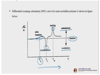
Now, please have a close look at this particular DSC curve this is representative DSC curve or polymeric sample. So, you can see d Q / d t is plotted versus temperature. So, when we start the process we heat basically we start, we are heating in this direction, we are increasing the temperature so, what is happening that something will call there is a glass transition phase will come.
