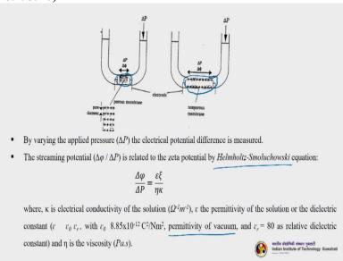
Now we will discuss actually how it happens. So you can see there are 2 figures here. So, capillary tube or u tube manometer type of arrangements in which are holding porous membrane as well as non-porous membrane. So porous membrane is fixed here. So this is actually a porous membrane this is non-porous membranes are arranged in his slit since they do not have pore so they are arranged in a particular way edge slits.
