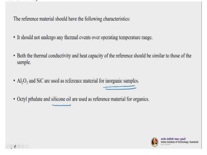
So what is the reference material. What is it is important that we understand the importance of reference material. It is inner material mostly and it is not the with whatever the amount of it that is being supplied. So, it should not undergo any thermal events over operating temperature range. I am telling you about the characteristic which is up the reference materials.
