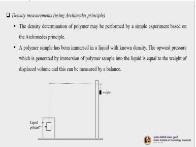
So, you can measure density by Archimedes principle also very easy. So, then density determination of polymer may be performed by simple experiment based on Archimedes principle. So, what is been happening here you can see here a polymer sample has been immersed in a liquid within non density. So, we are taking a polymer sample of which we want to measure the density we are immerse it in a liquid whose density is known to us.
