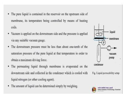
Now pure liquid is contained in the reservoir now when we talk about actually liquid permeability, the mechanism by which both air permeability or gas permeability and liquid permeability or this one carried out are mostly the same. So, the liquid is contained in the reservoir on the upstream side of membrane and its temperature being controlled by means of heating coils.
