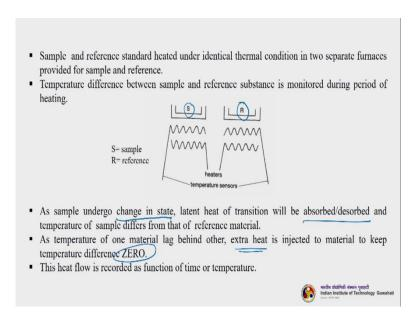
So, let us understand what DTA is so the sample in reference standard heated under identical thermal condition in 2 separate furnaces provided for sample and reference. So, there are 2 furnaces another single furnace DTA. So, you can see here this furnace is holding the sample this furnaces is holding the reference now and both sample and references are getting heated. Or heat is being supplied to them and uniform heat is being supplied to them. Now as sample undergo change in state.
