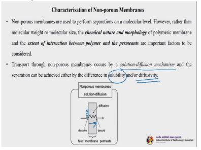
So, now, let us understand the characterization of non-porous membranes So, will exclusively discuss about non porous membranes and non-porous membranes are used to perform separations on a molecular level however, other than molecular weight or molecular size, the chemical nature and morphology of the polymeric membrane and the extent of interaction between the polymer and the permeants are important factors to be considered.
