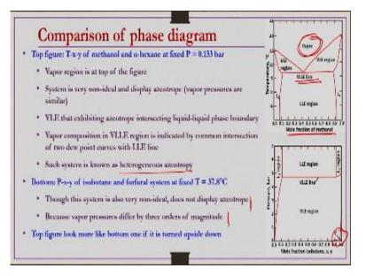
Comparison of phase diagram. T-x-y diagram that we have drawn for Methanol n-hexane system in previous lecture is given here. T-x-y of Methanol n-hexane at fixed pressure of 0.133 bar is given shown here and then bottom figure indicates the P-x-y diagram of whatever the iso-butane and then furfural that we have just taken example problem we solve the problem and then draw this phase diagram.
