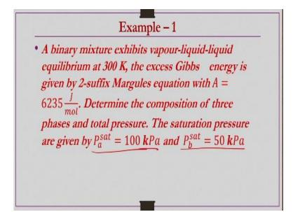
So now what we have we will take an example problem, a binary mixture exhibit vapor liquid liquid equilibrium at 300 K, the excess gives energy is given by 2-suffix Margules equation with A = 6235 Joules per mole. Determine the composition of 3 phases and total pressure this saturation pressures are given as  $P_a^{sat}$  100 kilopascals and  $P_b^{sat}$  50 kilopascals that is 1 bar or it is approximately 1 bar  $P_a^{sat}$  and  $P_b^{sat}$  is approximately 0.5 bar.
