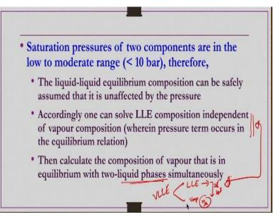
Saturation pressures of 2 components are in the low to moderate range therefore the liquid-liquid equilibrium composition can be safely assumed that it is unaffected by the pressure. Accordingly one can solve LLE composition independent of vapor composition wherein the pressure term
