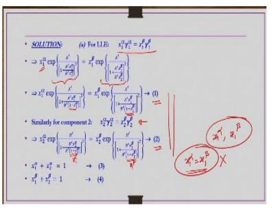
So for LLE component 1 and 2 take  $x_1^{\alpha} \gamma_1^{\alpha} = x_1^{\beta} \gamma_1^{\beta}$  for component 1, so  $x_1^{\alpha}$  and then  $\gamma_1^{\alpha}$  for Van Laar equation is nothing but  $\exp\left\{\frac{A'}{\left[1+\frac{A'x_1^{\alpha}}{B'x_2^{\alpha}}\right]^2}\right\} = x_1^{\beta}$  and then  $\gamma_1^{\beta}$  is nothing but  $\exp\left\{\frac{A'}{\left[1+\frac{A'x_1^{\beta}}{B'x_2^{\alpha}}\right]^2}\right\}$ .
