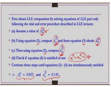
Because the pressure is in the low to moderate range. So first obtain the LLE composition by solving equations of LLE part only following the trial and error solution procedure described in LLE lectures. What we have done there, we have to assume a value of  $x_a^{\alpha}$  and then using equation 1 in the previous slide I have written, compute  $x_a^{\beta}$  and then from equation 3 you obtain, what is  $x_b^{\alpha}$ .
