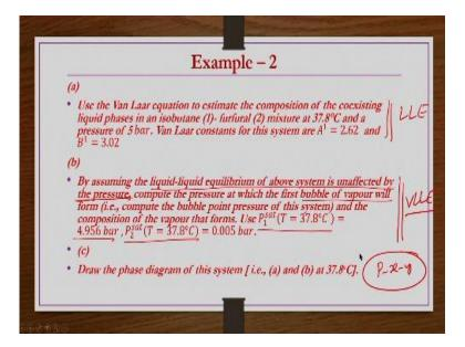
Now what we do we take another example problem. Use the Van Laar equation to estimate the composition of the coexisting liquid phases in an iso-butane and furfural mixture at 37.8 degree centigrade and a pressure of 5 bar. Van Laar constants for this system are given as  $A^1$  is nothing but 2.62 and  $B^1$  is nothing but 3.02. So that is first part that is only LLE part is there, there is no vapor.
