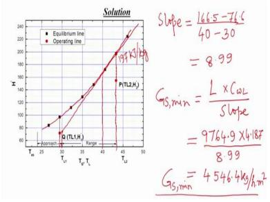
Both the values we have so that the bottom point that is Q is pointed here like this a TL1 is 29.4 degrees Celsius and Enthalpy value is 71.7 kilo Joule per kg dry air. So this Q point is the bottom point of the operating line. Now we have to do one thing. We have to draw the equilibrium curve So this for this equilibrium curve this Enthalpy values are already giving whatever the H star
