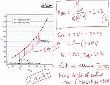
So this Ntog will be equal to say integration H2 prime to H1 prime and DH prime by H star prime minus H prime. So it will be coming at 2.82. So just area under the curve whatever we have drawn this one like this area under the curve from this point to this and say this portion from this we can say this one total area under the curve that is Ntog.
