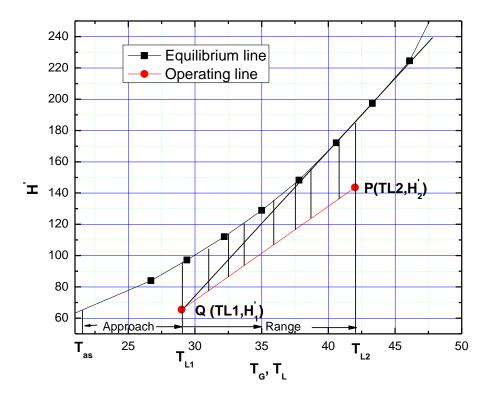
$T_{Gl}$ =32°C,  $T_{wl}$ =22°C, From psychrometric chart,  $Y_1' = 0.013 \ kg/kg \ dry \ air$
