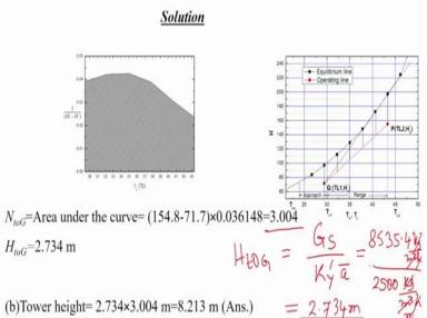
Now we will be calculating this Htog. That Htog will be calculating just by we can say this one Htog that is we can say this one Htog that is from the formula whatever is we know Gs by capital Ky prime a bar is equal to say that is Gs is given as 8535.4 say kg per meter square hour so kg
