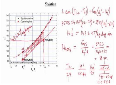
Now say we have this equilibrium line then we have this slope, will say 6 using this slope 6.006 we can draw this line actually. But you see this one using this minimum flow rate we have drawn this line so this for we can minimum gas flow rate. This is for actual gas flow rate using this we can say 5923 kg per hour meter square. Okay.
