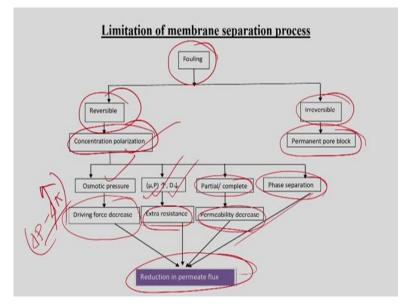
Then we have already discussed in detail about the limitation of the membrane separation processes like this we also highlighted that the fouling is the major drawback of the membrane separation processes because as this is the red separations processes with time the solutes will be deposited on the membrane surface and then fouling will take place. And that fouling may be of 2 type like 1 is the reversible fouling and another is the irreversible fouling.
