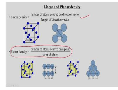
And then we have discussed about the linear density like number of the atoms centred on the direction velocity direction vector divided by the length of the direction vector and in case of the planar density we described about this number of atom to centred on a plane divided by area of the plane.
