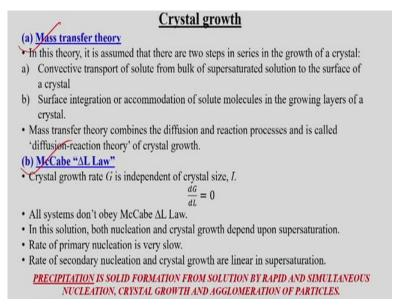
And then so we discussed about the crystal growth like using this mass transfer theory is the MeCabe delta L law and we this one explained that the precipitation is solid formation from the solution by rapid and simultaneous nucleation crystal growth and agglomeration of the particles.
