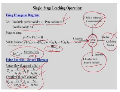
Like the single stage operation that is for extraction whatever we have discussed the same thing is applied here means the leaching process suppose we have the solid to be least means this is one particular solid with insoluble A mass insoluble or inert is there, then here actually in leaching process we are adding this leaching solvent like extracting solvent, then under flow will be there where the inert will be coming with the small amount of this one target component say C.
