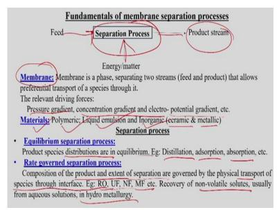
Now, we will be discussing this membrane separations technology there this we have already discuss this fundamentals of the membrane separation process like say if we say this is the process then feed is entering and we are suppose suppling energy or matter, then products are actually formed like this, so for that we described this membrane as we say phase, separating two streams like this feed and product that allows the preferential transport of a species through this barrier.
