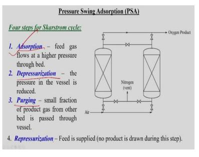
And then we discussed about the pressure swing adsorption process, then adsorption, then depressurization, then purging and then this one repressurization also we have discussed this one.
