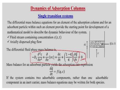
And we have discussed in detail about the dynamic of the adsorption column and like the single transition system that differential form is like:
