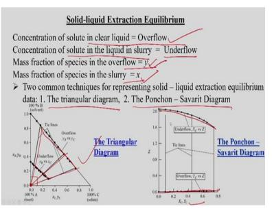
Like this Solid Liquid Extraction Equilibrium, it is equivalent to that of the liquid liquid extraction equilibrium like this concentration of the solute in the clear liquid that is overflow, then concentration of the solute in the liquid in the slurry that we say this an underflow or this like carrier solvent here is this inert solid, so that is underflow.
