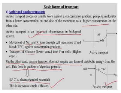
Now, this active and passive transport is there through the membrane like this, this are the basic form of the transport. Active transport processes usually work against a concentration gradient, this pumping molecules from a lower concentration on one side of the membrane to a higher concentration on the other side like this. So, that is why we can see this one that is active transport is an important phenomenon in biological system.
