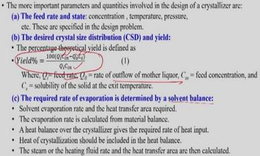
And we discussed about the design of the crystallizer, by this on the feed rate and the state by the desired crystal size distribution and the yield like this yield as calculated like this 100 into Qi into Cin minus Q into Cs divided by Qi into Cin, where Q is equal to feed rate and Q is equal to rate of the outflow of the mother liquor.
