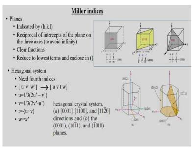
With the different example. And miller indices also that is indicated by h k l, in this x y z in 3 directions using this these indices we are able to designate particular hexagonal crystal system.
