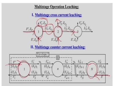
Like this Multistage leaching operation similar to that of the extraction process, suppose this feed is entering and extracting solvent is added then we have this overflow then underflow, then underflow of the stage 1 will be the feed to the stage 2, then again we are adding solvent and then we are getting overflow like that is continued.
