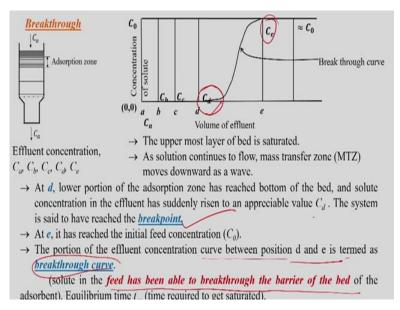
And this breakthrough like this whenever we say this one whenever this this concentration of the solute in the effluent actually we will suit up from Cd to Ce, this one at point d the lower portion of the adsorption zone has reach bottom of this bed. And this solute concentration in the effluent has suddenly risen to the appreciable value Cd.
