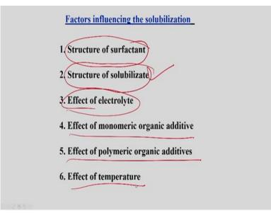
And the factors that influencing the solubilisation are like this structure of the surfactant like this and structure of the solubilizate which we actually try to trap using the surfactant, then effect of the electrolyte then effect of the monomeric organic additive, then effects of the polymeric organic additives, then effect of temperature also.
