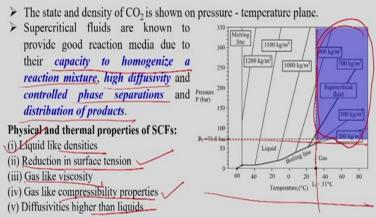
And another point actual we discuss this under this solid liquid extraction process or leaching that is the super critical feed extraction that is in this in case of this this one what is called TBT diagram, suppose this above a critical particular temperature and above a critical pressure there is 1 zone where it is actually to behaving as supper critical fluid.
