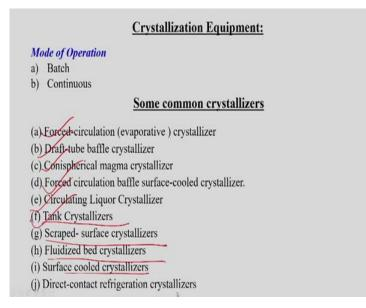
And some equipment for crystallization are of like batch and continuous, some common crystallizer are like forced circulation, then draft tube, then conispherical, forced circulation baffle surface cooling crystallizer, then circulating liquid crystallizer, then tank crystallizer it is used like scraped surface crystallizer, fluidized bed, then surface cooled and direct contact refrigeration crystallizer also.
