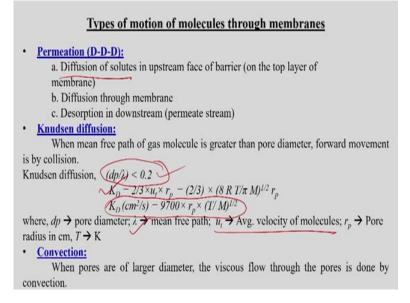
Like this this types of motion of the molecules through the membranes that is one is the permeation D-D-D concept like this a diffusion of the solutes in the upstream face of the barrier and then diffusion through the membrane and then desorption in the downstream.
