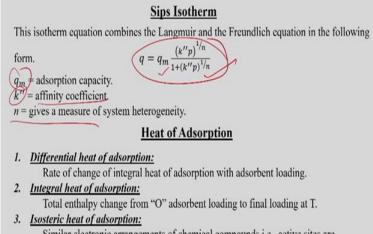
Similar electronic arrangements of chemical compounds i.e., active sites are energetically homogeneous  $\rightarrow$  heat of adsorption is independent of adsorbent loading.
