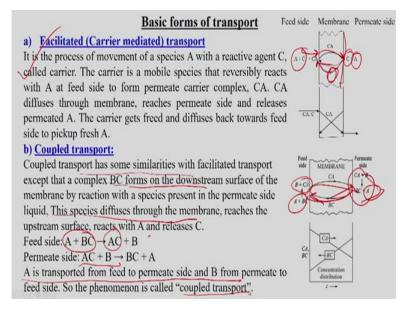
Now the basic forms of the transport like this one of this facilitated transport like this carrier mediated transport and like this first one like this, A plus C that will coming as CA and it will be transport porting to this opposite side of the membrane and then it will be separated into C and A and carrier will be coming back to the back side of the feed.
