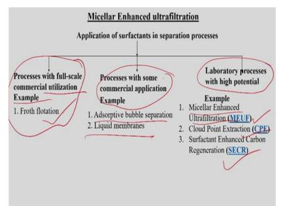
Then we have discussed in detail about the micellar enhanced ultrafiltration where if the surfactants are solubilised over there critical micelle concentration then micelle is formed then this micellar will be able to trap these solutes and then make the big globules.
