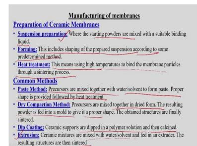
Now, this for ceramic membranes the preparations of ceramic membranes are done by mostly the suspension preparation for the starting powders are mixed with a suitable binding liquids. Then forming is done this shaping of the prepared suspension according to some predetermined method. Then heat treatment is done this means this one using high temperature to bind the membrane particles through sintering process.
