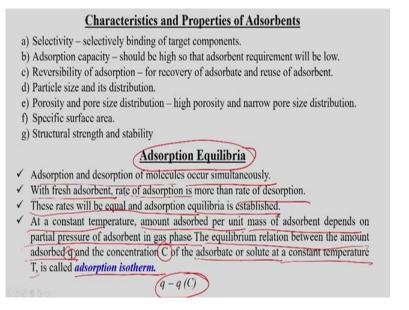
And characteristic and the properties of the adsorbent are like this selectivity then adsorption capacity, then reversibility, then particle size and its distribution, then porosity and pore size distribution, then specific surface and structural strength of the and the stability also.
