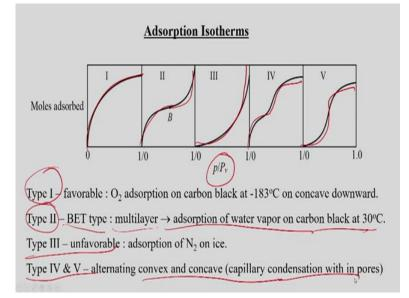
Now, you say we learned also hat types of isotherms are different 5 types like this 5 type, type a is favourable hence with P by Pv this moulds absorb actually is increasing constantly. Type b actually BET type B is multilayer in the beginning it is increasing but this rate actually is decreasing after that, like adsorption of the water vapour on the carbon black at 30 degree Celsius.
