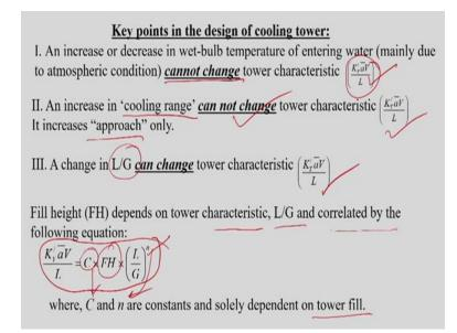
And the key points in the design of the cooling towers are like this an increase or decrease in the wet bulb temperature of the entering water that is mainly due to the atmospheric condition like this I told that say in the winter or in the monsoon period or in maybe in summer, so we can say
