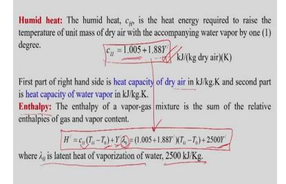
Then we have learned also the humid heat that humid heat or we say this CH that is we can say we expressed in using one equation like:
