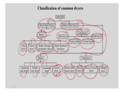
Then the classification of the common dryer actually we discussed in terms of direct heat drying and in terms of indirect heat drying like this in terms of direct heat drying that was one was batch and one was continuous, in batch that was tray dryer then truck dryer and we have this batch through circulation dryer then batch fluidized bed dryer.
