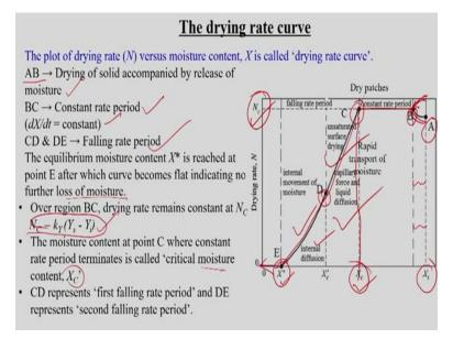
And we have also learned the details about the drying rate curve, so we started from this suppose this point A and then it move to point B by we can say this initial adjustment during this drying process that A be here also like this sometimes this drying rate may increase, sometimes this drying rate may decrease also during this initial adjustment.
