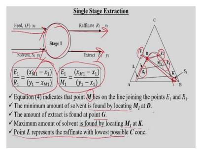
Now we have discussed about the single stage extraction process like this suppose this is the single stage and then feed is entering from here and solvent is added and then raffinate and the extract phases are separated:
