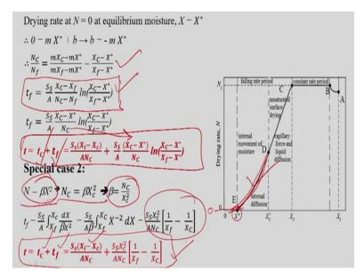
And drying rate N is equal to zero at equilibrium moisture content that we know this one that N is equal to zero here actually and in that case we can say 0 is equal to MX star plus b were b is equal to minus MX star will be and in that equation previous NC by Nf we will be getting as XC minus X star by Xf minus X star.
