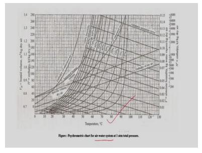
So this is the we can say for air water system this is the psychrometric chart I think we have used several times for solving so many problems in both the humidification and drying also. Because the same psychrometric chart is used for the any of the drying of the wet solutes as well as this humidification operation as well as this air conditioning system because there water is evaporated in air, so that is why we able to use the psychrometric chart.
