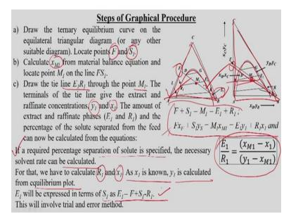
And the steps of the graphical procedure we have already derived described this one like say we need to locate this S1 we need to locate the F like draw the ternary diagram first we have to draw the this ternary diagram like this one or we have to draw this one and then we can say this one on the equilateral triangular diagram or any other diagram like this right angle diagram whatever maybe then we need to locate this point feed point and the solvent one.
