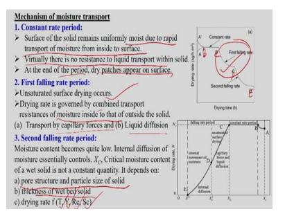
So the mechanism of the moisture transport also from this A point to B to C to D to E like here you can say this A to B, B to this is like this is C, C to D, D to E I can say, A to B here like this constant rate period that we can say surface of the solid remains uniformly moist to the rapid transport of the moisture from the inside to the surface.
