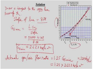
So whenever will be drawing, draw a tangent to the equilibrium line say suppose through Q suppose this one this black line actually we can say we need to draw this, so first we have identified this bottom point then we have drawn this equilibrium line and then we have drawn a tangent to the we can say equilibrium line through Q.
