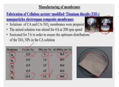
And another one is the fabrication of cellulose acetate-modified-titanium oxide nanoparticles electrospun composite membrane, that is also used for a particular application, okay? So for that case suppose this is a cellulose acetate solution and this is cellulose acetate titanium dioxide solution and then say the mix solution was stirred for 4 hour at 200 rpm speed and then sonicated for 3 hour in order to ensure the optimum distributions of the TiO2 nanoparticles in the cellulose acetate.
