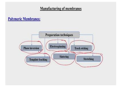
We will be discussing first the manufacturing of the polymeric membranes. There are six manufacturing processes for the polymeric membrane fabrication, one is this phase inversion technique, then another is template leaching and one process is electrospinning and another processes sintering and one processes track etching and another process is stretching.
