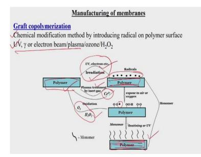
And another method of the manufacturing of polymeric membrane using graft copolymerization process, this is we can say the specific application, for the specific application of the polymeric membrane that is done like chemical modification method by introducing radicals or on the polymer surface and then we can say this one UV, gamma or electron beam or plasma or ozone or hydrogen peroxide, these are used as the grafting.
