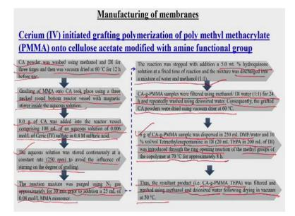
And now we can get this one cerium initiated grafting polymerization of poly methyl methacrylate (PMMA) into cellulose acetate modified with amine functional group also. In that case we can say this we can, we need to take the cellulose acetate powder that will be say we need to wash using this methanol and deionized water for three times and then was vacuum dried at 60 degree Celsius for 12 hours before this use.
