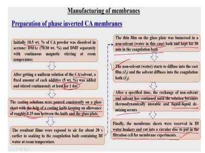
And regarding this manufacture of the cellulose acetate membrane using this phase inversion technique and then by applying this digital film applicator or casting knife, so this is a typical procedure actually of the manufacture of phase inverted cellulose acetate membrane. Suppose initially 10.5 wt percent cellulose acetate powder was dissolved in acetone DMAc mixture that is 70 is to 30 and DMF separately with continuous magnetic stirring at room temperature.
